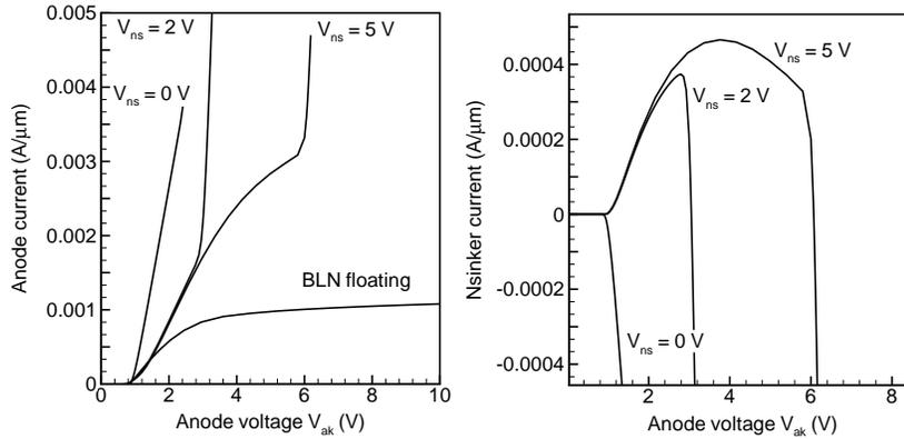
**Figure 5.30** Anode currents at  $V_{gk} = 3.3\text{ V}$  in the case of floating and contacted BLN (left). Currents at  $V_{gk} = 3.3\text{ V}$  through the nsinker contact in the case of a contacted BLN (right).
