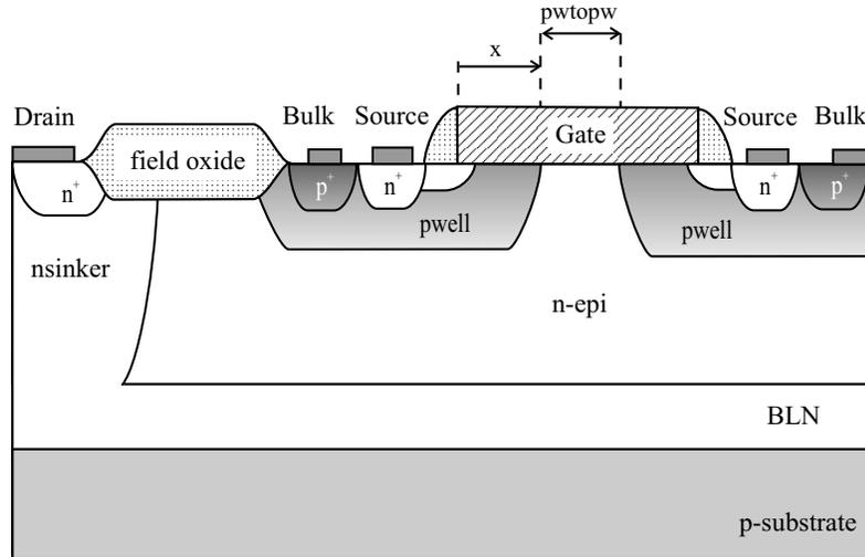
**Figure 4.30** A floating integrated vertical nDEMOS device with BLN and its most important layout parameters.
