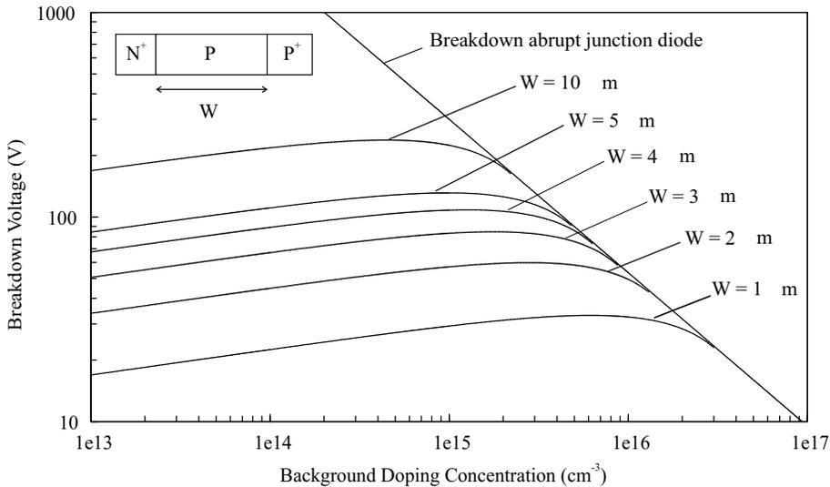
**Figure 2.6** Breakdown voltage for an abrupt junction diode and for a punch-through diode of several widths. The insert shows a punch-through diode.
