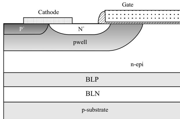
**Figure 5.43** An integrated non punch-through IGBT.
