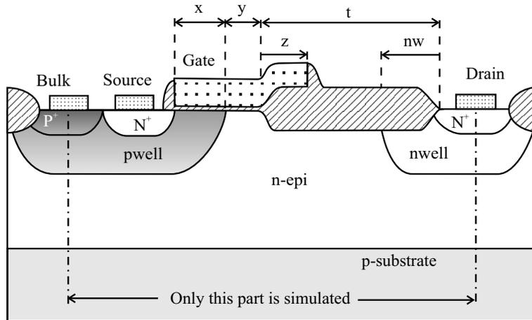
**Figure 4.15** The low-side “free” RESURF nLDEMOS device and its most important layout parameters.
