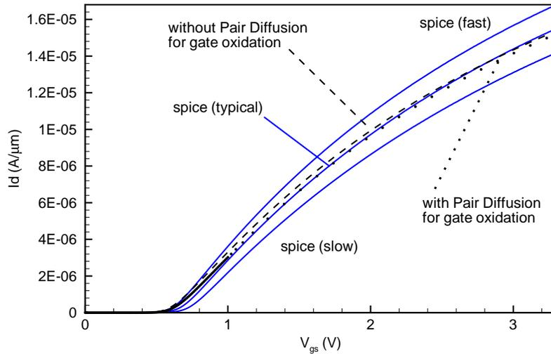
**Figure 3.7**  $I_d(V_{gs})$  for a nMOS with drawn channel length of  $2\ \mu\text{m}$ : SPICE simulations versus TCAD simulations.
