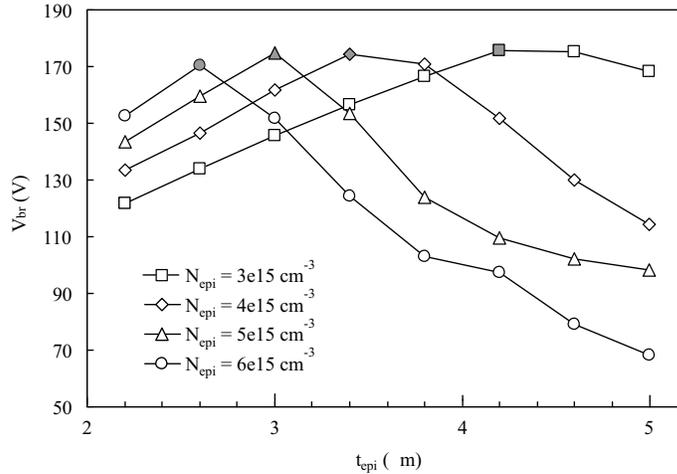
**Figure 4.16** Breakdown voltage of the “free” RESURF nLDEMOS device as a function of epi thickness for several n-epi doping levels. Filled data points are the optima for each doping level.
