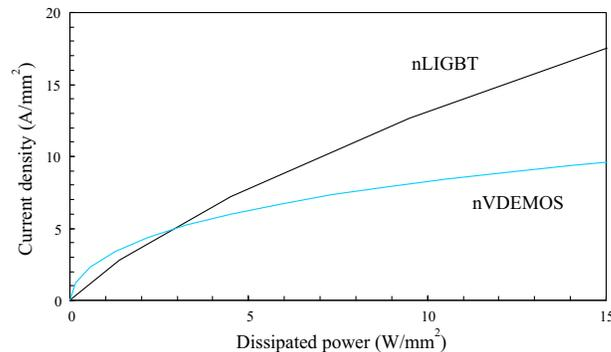
**Figure 5.49** *Measured* current density versus power dissipation at  $V_{gk} = 3.3$  V for the nLIGBT with BLN and BLP compared with a typical nVDEMOS (at  $V_{gs} = 3.3$  V).
