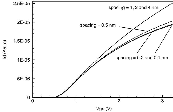
**Figure 3.6**  $I_d(V_{gs})$  at  $V_{ds} = 0.1$  V for a nMOS with drawn channel length of  $2\ \mu\text{m}$  for several distances between the mesh lines in the y direction in the channel (i.e., the parameter ‘spacing’).
