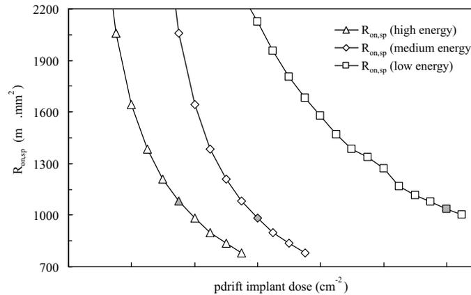
**Figure 4.40** Specific on-resistance  $R_{on,sp}$  as a function of the pdrift implant dose for several implant energies. Filled data points correspond to the maxima in  $V_{br}$  (figure 4.39).
