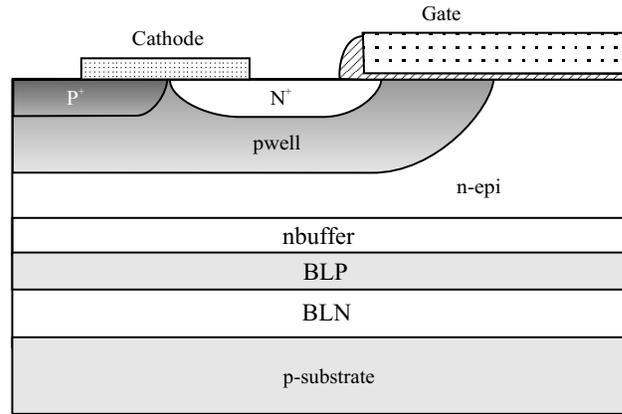
**Figure 5.44** A vertical punch-through IGBT.
