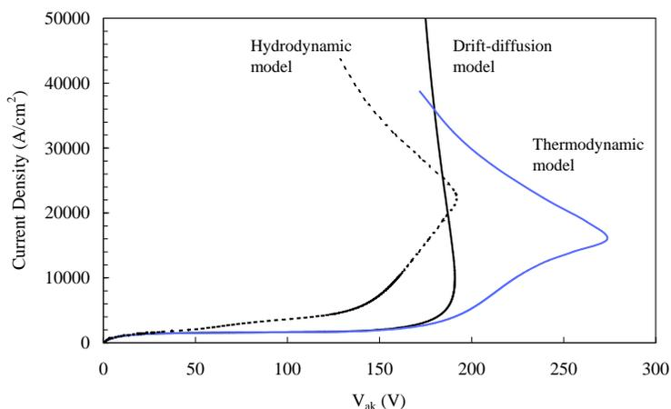
**Figure 2.2** Current density versus applied voltage for a silicon bar, simulated with the drift-diffusion model, the thermodynamic model and the hydrodynamic model.
