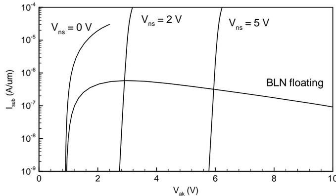
**Figure 5.31** Substrate currents at  $V_{gk} = 3.3\text{ V}$  in the case of floating and contacted BLN.
