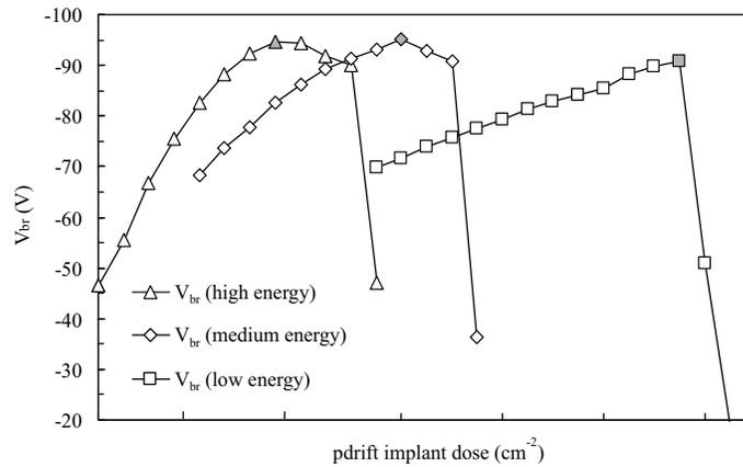
**Figure 4.39** Breakdown voltage  $V_{br}$  as a function of the pdrift implant dose for several implant energies. Filled data points show the maxima.
