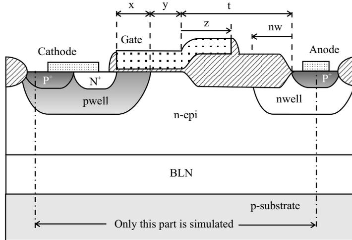
**Figure 5.5** The LIGBT with standard I3T80 layers.
