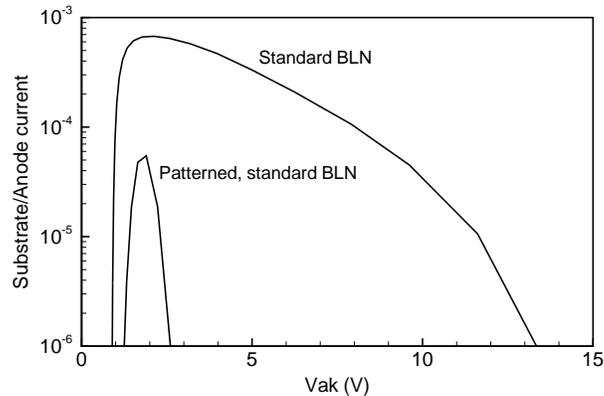
**Figure 5.37** Substrate to anode current ratio at  $V_{gk} = 3.3$  V for the nLIGBT with a patterned BLN, compared to the standard case (no BLN mask).
