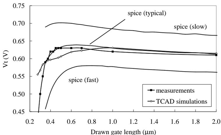
**Figure 3.8** Threshold voltage versus drawn channel length for nMOS transistors: comparison between measurements, TCAD and SPICE simulations.
