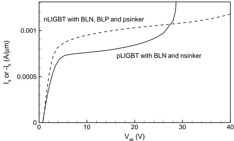
**Figure 5.39** The output characteristic of a pLIGBT (at  $V_{ga} = -3.3$  V) with  $blnend = 0$   $\mu\text{m}$  compared with a nLIGBT (at  $V_{gk} = 3.3$  V) with a floating BLN, BLP and psinker.
