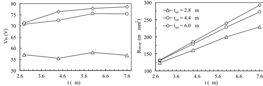
**Figure 4.28** Breakdown (left) and specific on-resistance of a floating nLDE-MOS on top of a BLN with  $N_{epi} = 4e15\text{ cm}^{-3}$  as a function of the field oxide length  $t$  for several variations of epi thickness.
