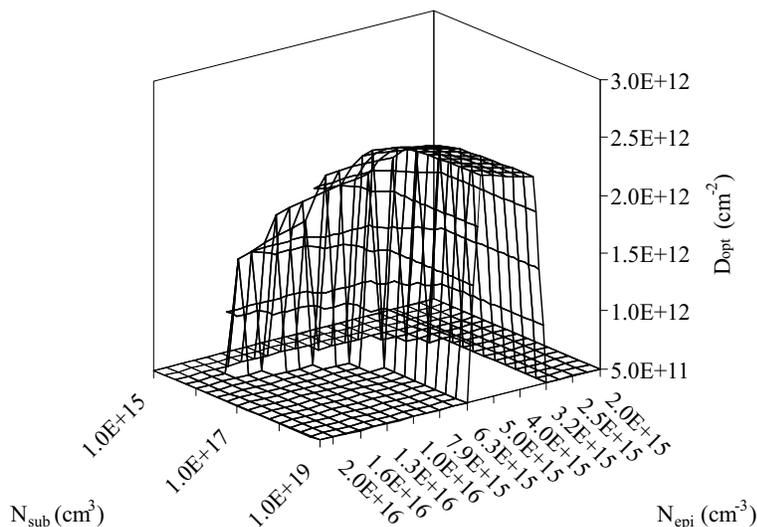
**Figure 4.6** Optimal RESURF epi dose  $D_{opt}$  for a corresponding ideal RESURF breakdown between 80 V and 120 V, and  $t_{epi,opt} > 1 \mu\text{m}$ .
