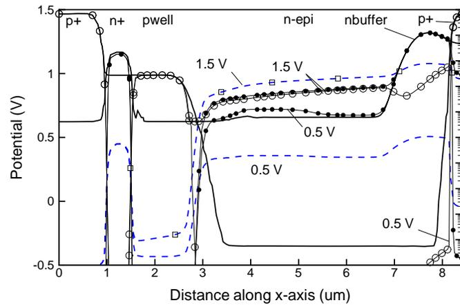
**Figure 5.7** Electron density ( $\bullet$ ), hole density ( $\circ$ ), donor and acceptor concentrations (solid lines) are plotted against the right y-axis (log scale), the potential (dashed lines) against the left y-axis for the LIGBT of figure 5.6 at  $V_{gk} = 1.1\text{ V}$  with  $V_{ak} = 0.5\text{ V}$  and  $V_{ak} = 1.5\text{ V}$ . The cutline runs parallel with the silicon surface, along the entire device length, just underneath the field oxide.
