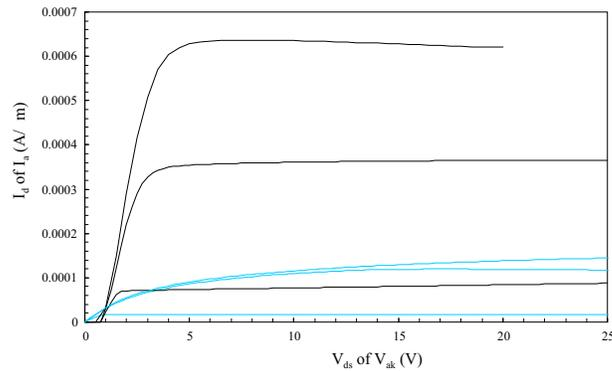
**Figure 5.48** *Measured* output characteristics at  $V_{gk} = 1.1, 2.2$  and  $3.3$  V for the nLIGBT with BLN and BLP compared with a typical nVDEMOS (blue, at  $V_{gk} = 1, 2$  and  $3.3$  V).
