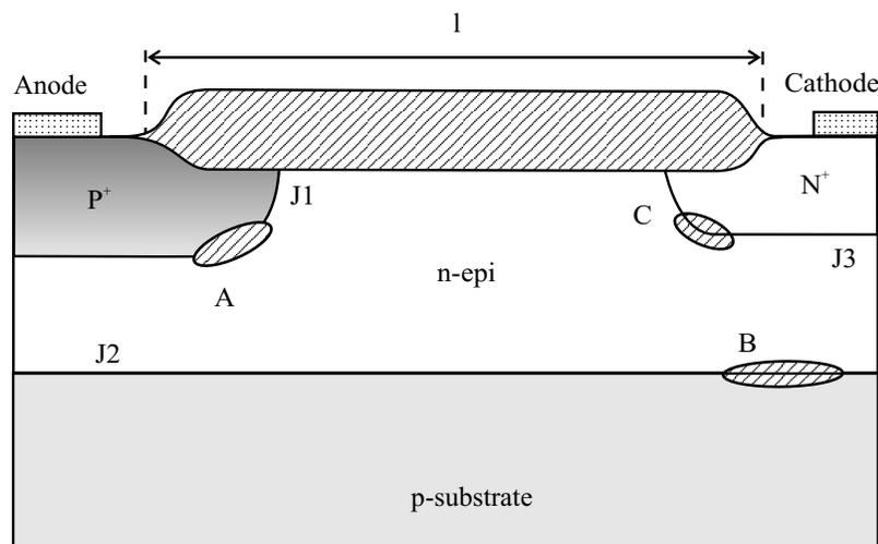
**Figure 4.1** A RESURF diode.
