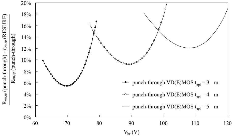
**Figure 4.13** Relative difference (in %) between the silicon limit for punch-through vertical nD(E)MOS devices and lateral RESURF nD(E)MOS devices.
