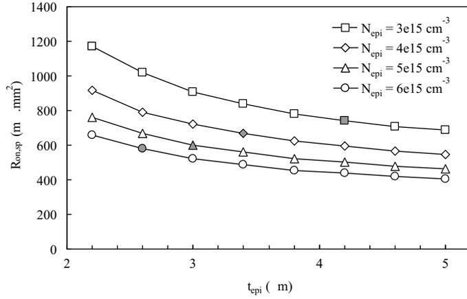
**Figure 4.17** Specific on-resistance of the “free” RESURF nLDEMOS device as a function of epi thickness for several n-epi doping levels. Filled data points correspond to the optima in breakdown voltage (figure 4.16).
