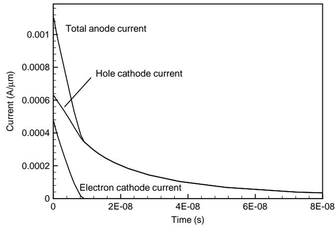
**Figure 5.18** Gate controlled turn-off from  $V_{gk} = 3.3\text{ V}$  to  $V_{gk} = 0\text{ V}$  in 10 ns with a resistive load of  $10\text{ k}\Omega$  and an off-state voltage of  $40\text{ V}$ . The initial current level is equal to the static latch-up onset current.
