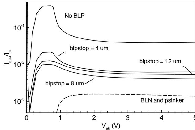
**Figure 5.22** Substrate to anode current ratio at  $V_{gk} = 3.3\text{ V}$  of a non-floating nLIGBT (figure 5.19 with several blpstop values) compared with a floating nLIGBT with BLN and psinker (figure 5.13).
