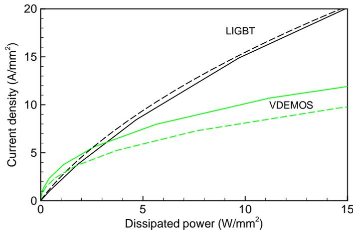
**Figure 5.17** Current density versus power dissipation at  $V_{gk} = 3.3\ \text{V}$  for an LIGBT as shown in figure 5.13 (solid black) compared with a typical VDEMOS (solid grey) at  $27^\circ\ \text{C}$ . The dashed curves are at  $125^\circ\ \text{C}$ .
