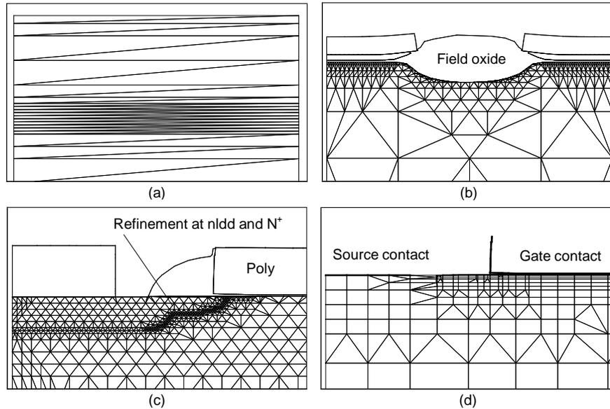
**Figure 3.2** Evolution of the mesh during simulation: (a) 1D in process simulation, (b) first process step in 2D, (c) at the end of the process flow, and (d) regridding before device simulation.
