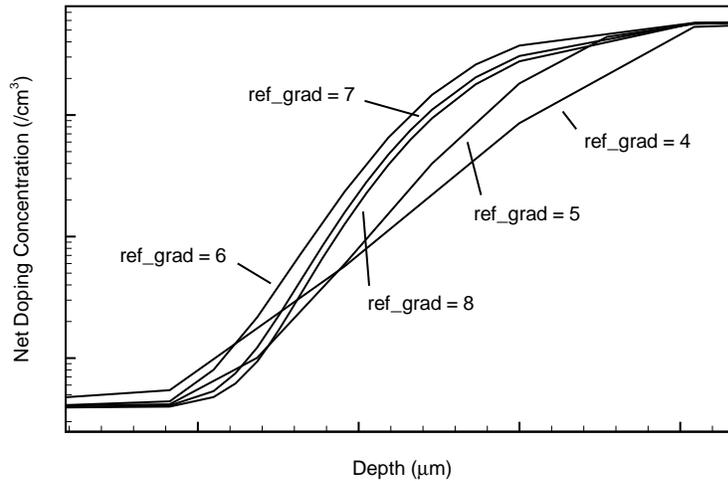
**Figure 3.1** Influence of the refinement gradient parameter on a doping profile.
