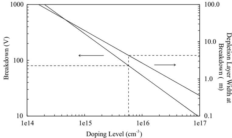
**Figure 2.5** Breakdown voltage and depletion layer width for an abrupt parallel-plane  $n^+$ /p junction diode versus the doping level of the p side.
