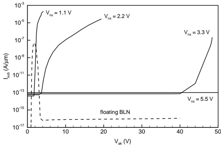
**Figure 5.36** Substrate currents at  $V_{gk} = 3.3$  V in the case of a contacted non-standard BLN.
