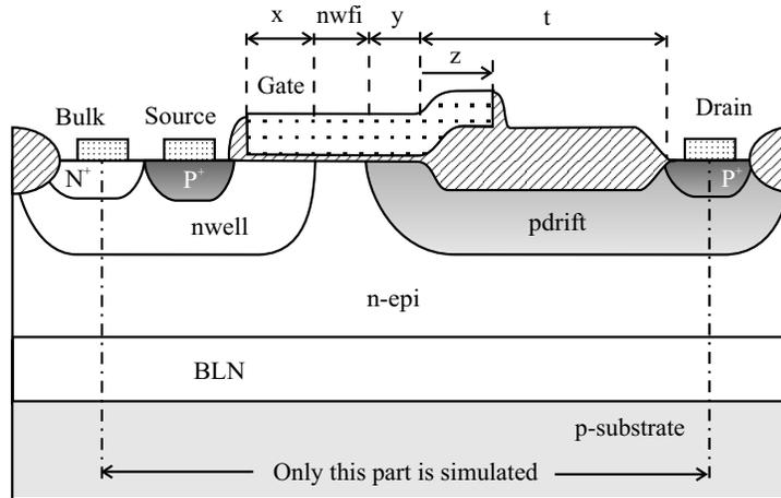
**Figure 4.35** A high-side RESURF pLDEMOS device with its most important layout parameters (described in table 4.8).
