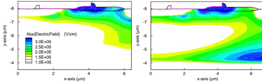
**Figure 4.24** Absolute value of the electric field at breakdown for a device with a lowly doped substrate ( $= 1e15 \text{ cm}^{-3}$  and  $N_{epi} = 6e15 \text{ cm}^{-3}$ , left) and a highly doped substrate ( $= 6e17 \text{ cm}^{-3}$  and  $N_{epi} = 8e15 \text{ cm}^{-3}$ ).
