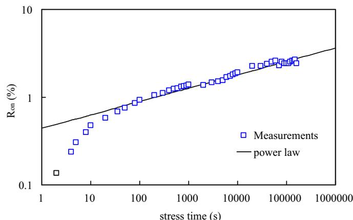
**Figure 4.47** Degradation of the pLDEMOS: measurements (squares) and fitted power law.
