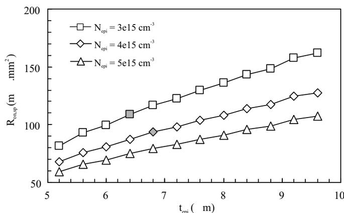
**Figure 4.32** Specific on-resistance of a floating nVDEMOS with an optimal pwtow as a function of the n-epi thickness for the highest possible n-epi doping levels. Filled data points indicate the device with a breakdown voltage over 80 V with the lowest specific on-resistance.
