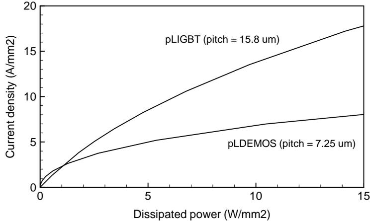
**Figure 5.40** Current density versus power dissipation (at  $V_{ga} = -3.3$  V) for an pLIGBT with  $blnend = 0$   $\mu\text{m}$  compared with a typical pLDEMOS (at  $V_{gs} = -3.3$  V).
