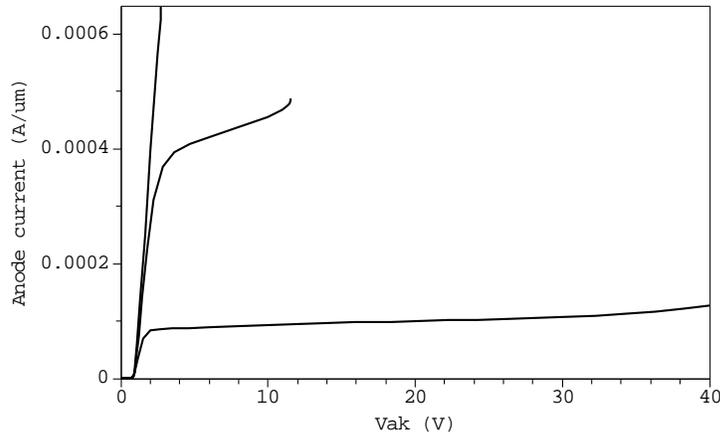
**Figure 5.11** Output characteristics at  $V_{gk} = 1.1, 2.2$  and  $3.3\text{ V}$  of an LIGBT with a nbuffer dose of  $1e15\text{ cm}^{-2}$  of table 5.1, and with pdrift over pwell.
