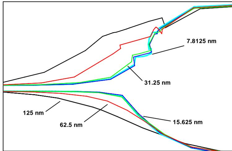
**Figure 3.3** Dependence of the bird's beak's shape on the edge length of the triangles.
