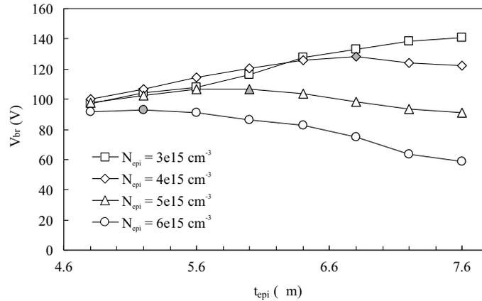
**Figure 4.20** Breakdown voltage of the RESURF nLDEMOS device with BLP as a function of epi thickness for several n-epi doping levels. Filled data points are the optima for each doping level.
