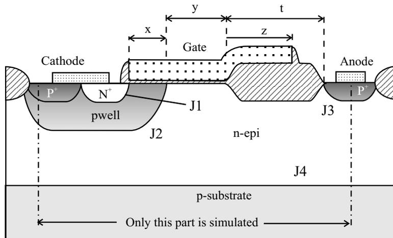
**Figure 5.1** The LIGBT device and its most important layout parameters.
