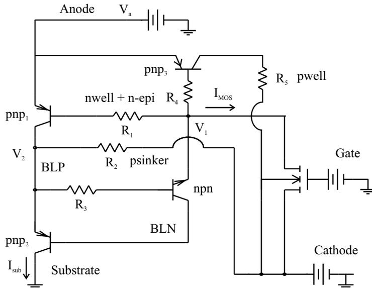
**Figure 5.28** Equivalent circuit for a nIGBT with floating BLN.
