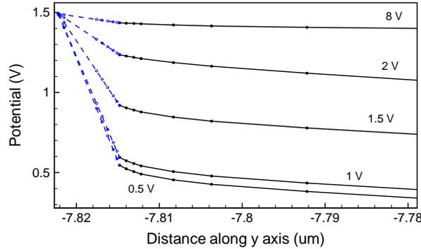
**Figure 5.8** Potential at the end of the channel (y-axis is perpendicular to the silicon surface) for  $V_{gk} = 1.1$  V and  $V_{ak} = 0.5, 1, 1.5 \dots$  V. The dashed lines show the potential in the gate oxide, the solid ones the potential in the silicon.
