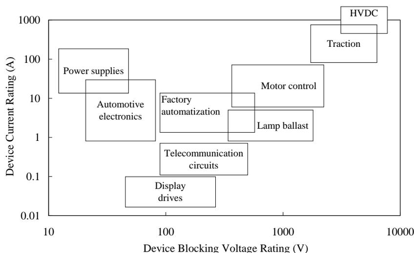
**Figure 1.1** Applications for power devices (after Baliga [Bal96b]).
