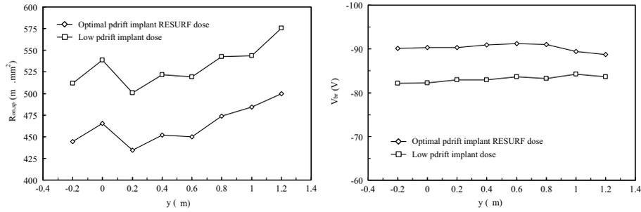
**Figure 4.42** *Measured*  $V_{br}$  and  $R_{on,sp}$  as a function of  $y$  for two pdrift implant doses.
