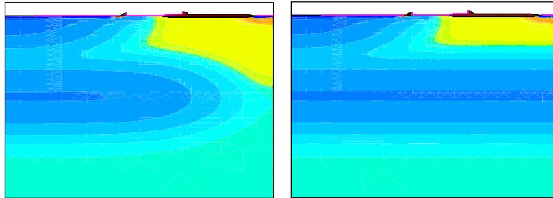
**Figure 5.20** The non-floating nIGBT with  $\text{blpstop} = 8\ \mu\text{m}$  has a better RESURF state (left) than the nIGBT with blank BLP implant (right) due to the bevelled edge of the blp/n-epi junction.
