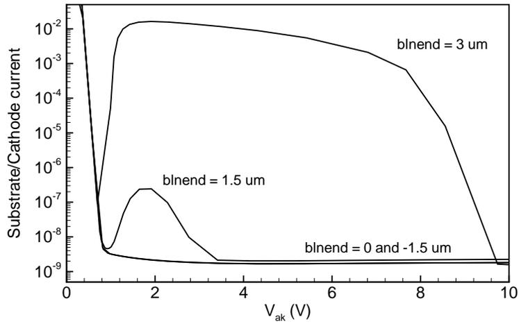
**Figure 5.41** Substrate to cathode current ratio (at  $V_{ga} = -3.3$  V) as a function of  $V_{ak}$  for pLIGBTs with different *blend* values.
