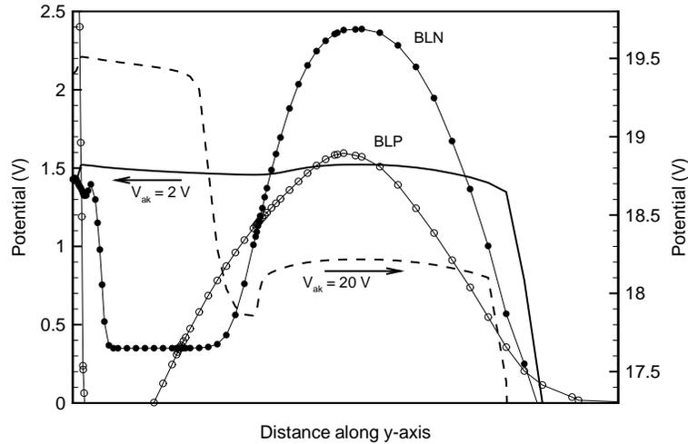
**Figure 5.27** Donor (●) and acceptor concentration (○), potential distribution for  $V_{gk} = 3.3$  V, and at  $V_{ak} = 2$  V (solid line) and  $V_{ak} = 20$  V (dashed line) as a function of depth taken at the end of the device ( $x = \text{pitch}$ ). Note that both the left and the right axis use the same scale for the potential, which shows that the potential bump at  $V_{ak} = 2$  V becomes a serious barrier at  $V_{ak} = 20$  V.
