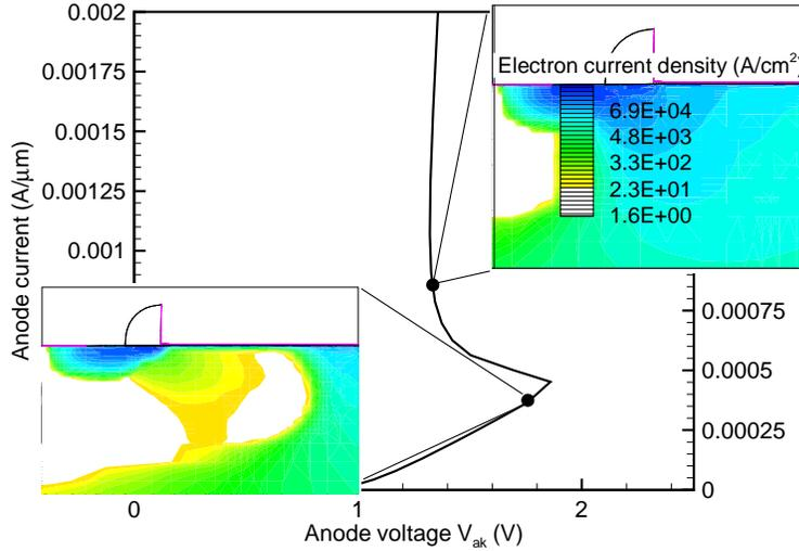
**Figure 5.9** Snapback at  $V_{gk} = 3.3$  V for the device which output characteristics are shown in figure 5.6. The lower inset shows the electron current density at the onset of latch-up, the upper inset the electron current density in thyristor mode.
