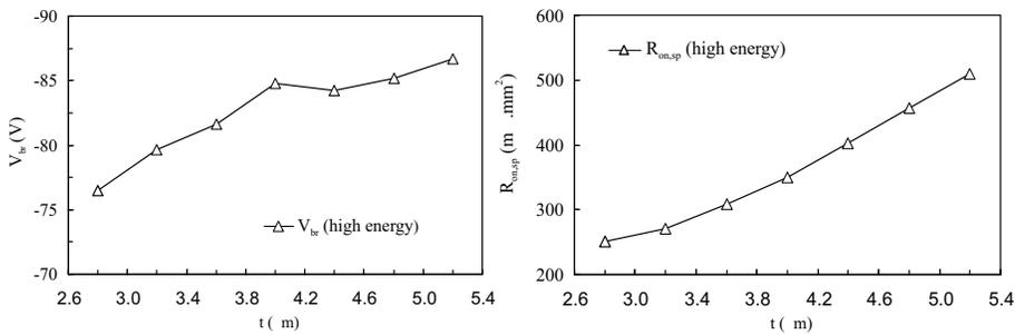
**Figure 4.41** Breakdown voltage  $V_{br}$  and specific on-resistance  $R_{on,sp}$  as a function of the layout parameter  $t$  for the highest pdrift implant energy with its corresponding optimal pdrift implant dose (simulated results).
