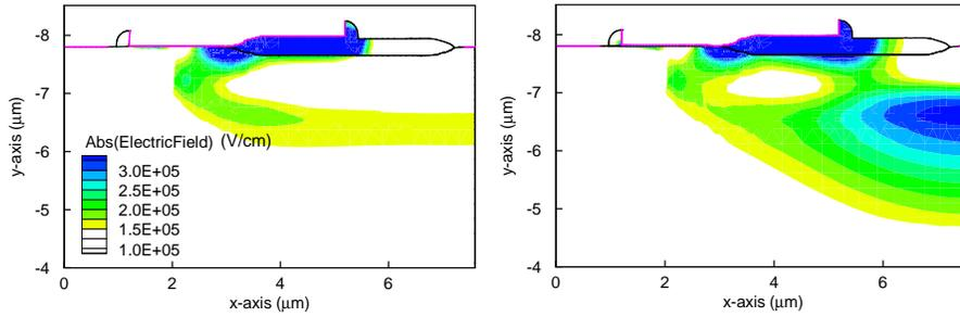
**Figure 4.46** Electrical field at breakdown in an “under resurfed” structure at  $V_{gs} = -1.5$  V and  $V_{ds} = -3.0$  V.
