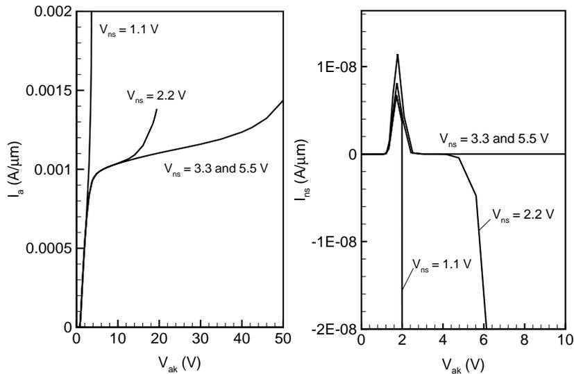
**Figure 5.35** Anode currents at  $V_{gk} = 3.3$  V in the case of a contacted non-standard BLN (left). Currents at  $V_{gk} = 3.3$  V through the nsinker contact in the case of a contacted non-standard BLN (right).
