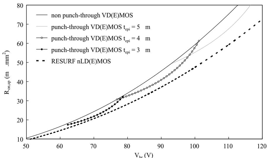
**Figure 4.12** Silicon limits for non punch-through and punch-through vertical nD(E)MOS devices, and for a lateral RESURF nD(E)MOS.
