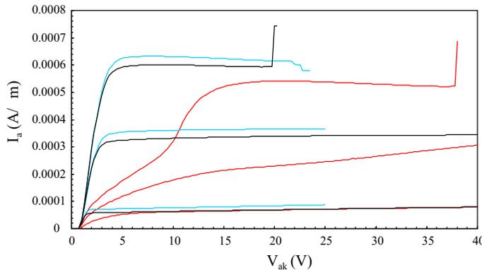
**Figure 5.47** *Measured* anode currents at  $V_{gk} = 1.1, 2.2$  and  $3.3$  V for the nLIGBT with BLN and BLP with three different values for  $ps$  (in  $\mu\text{m}$ ): 2.0 (red), 3.0 (blue) and 3.5 (black).
