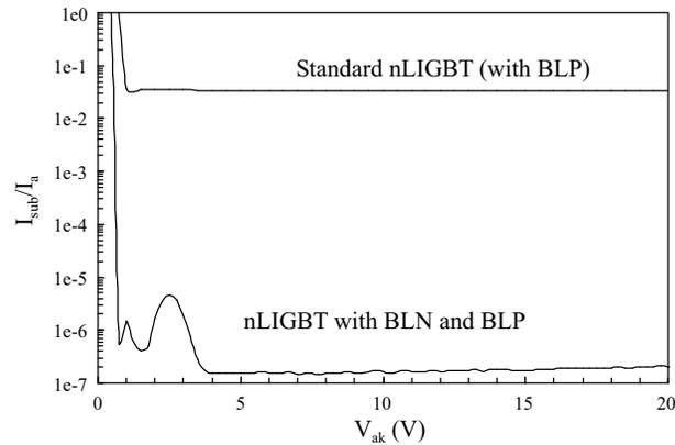
**Figure 5.50** *Measured* substrate to anode current ratio at  $V_{gk} = 3.3 \text{ V}$  for the nLIGBT with BLN and BLP, compared to the standard nLIGBT (only BLP present with  $blpstop = 8 \mu\text{m}$ ).
