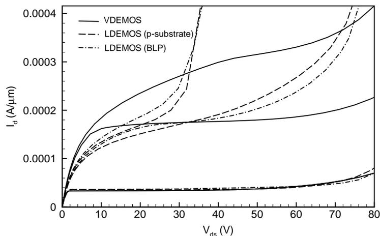
**Figure 4.34**  $I_d(V_{ds})$  characteristics at  $V_{gs} = 1.1, 2.2$  and  $3.3$  V for the best floating nVDEMOS and non-floating nLDEMOS devices on a n-epi with  $N_{epi} = 4e15 \text{ cm}^{-3}$  (as given in table 4.7). The nVDEMOS has clearly a larger SOA than the lateral RESURF devices.
