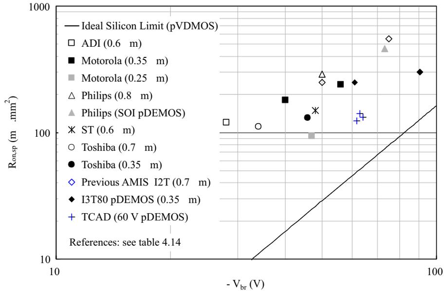
**Figure 6.2** Benchmark and competitors for the pDMOS devices.
