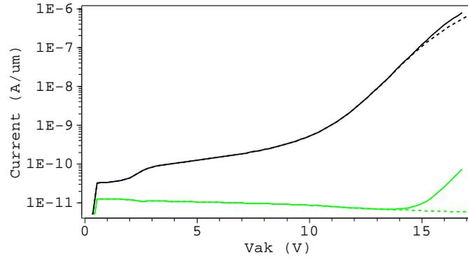
**Figure 5.3** Current through the anode (black) and substrate (green) contacts of a small LIGBT (figure 5.2) before and at breakdown. Solid lines are simulated with impact ionization, dashed ones without.
