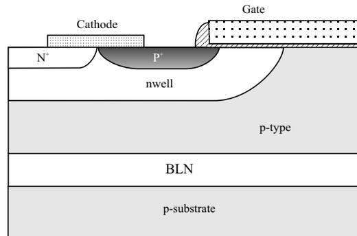
**Figure 5.46** A p-type quasi-vertical non punch-through IGBT.
