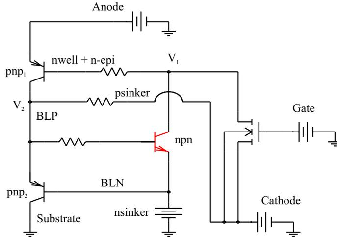
**Figure 5.29** Equivalent circuit for a nIGBT with contacted BLN, in the case where the nsinker contact is at low voltage compared to the anode voltage.
