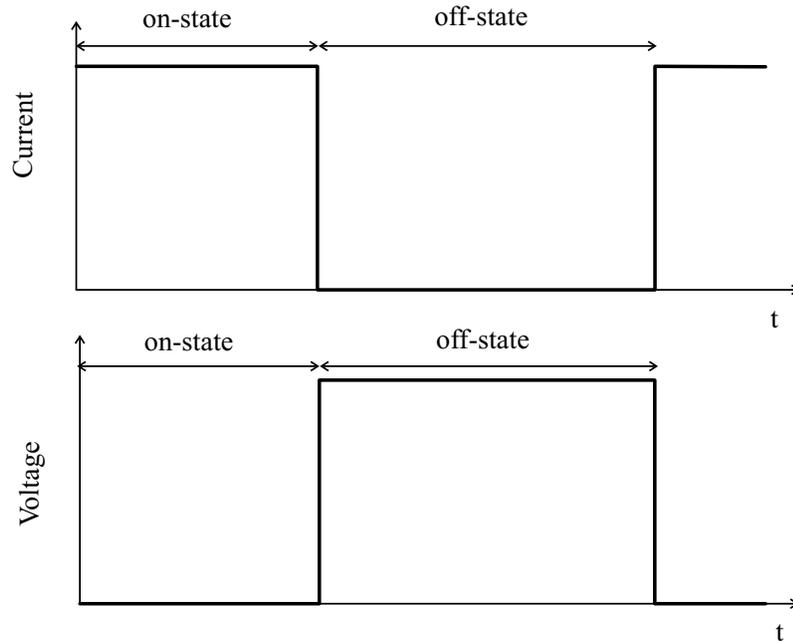
**Figure 2.3** Current and voltage waveforms of an ideal power device.
