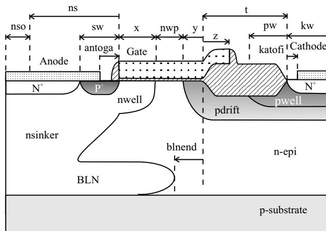
**Figure 5.38** The floating pLIGBT with nsinker and BLN. All the layout parameters defining this device are shown.
