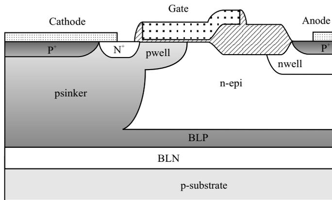
**Figure 5.23** The LIGBT device with psinker, BLP and BLN.
