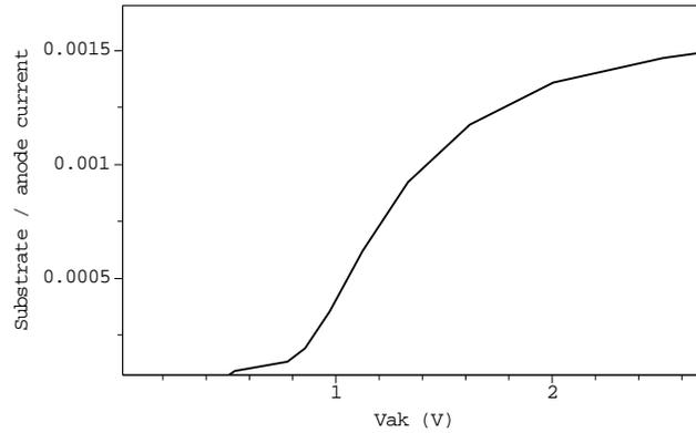
**Figure 5.12** The substrate current at  $V_{gk} = 3.3$  V is about 0.1% of the anode current in the forward conduction mode for the IGBT of figure 5.11.
