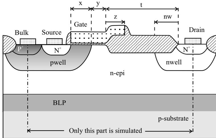
**Figure 4.19** The low-side RESURF nLDEMOS device on top of a BLP and its most important layout parameters.
