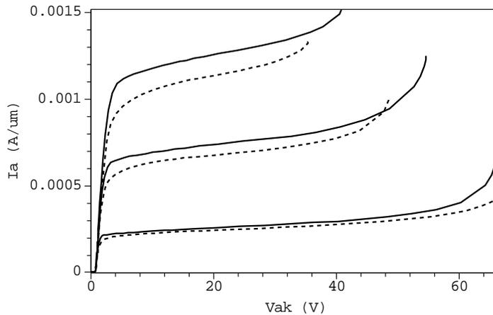
**Figure 5.32** Output characteristics at  $V_{gk} = 1.1, 2.2$  and  $3.3$  V of a floating nLIGBT with non-standard BLN (solid lines) compared with a floating nLIGBT with standard BLN (dashed lines). The non-standard BLN dose is 20 times lower than the standard dose.
