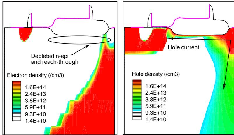
**Figure 5.2** Electron and hole densities at breakdown (forward, i.e.,  $V_{ak} > 0 \text{ V}$ ) for an IGBT with  $x = 1$ ,  $y = 0.3$ ,  $t = 3.6$  and  $z = 2.4 \mu\text{m}$ .
