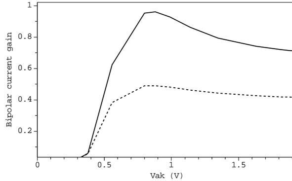
**Figure 5.10** The common-emitter current gain  $\beta$  (solid) and the common-base current gain  $\alpha$  (dashed) at  $V_{gk} = 3.3$  V of the intrinsic bipolar of the LIGBT with a buffer dose of  $1e15 \text{ cm}^{-2}$  of table 5.1.
