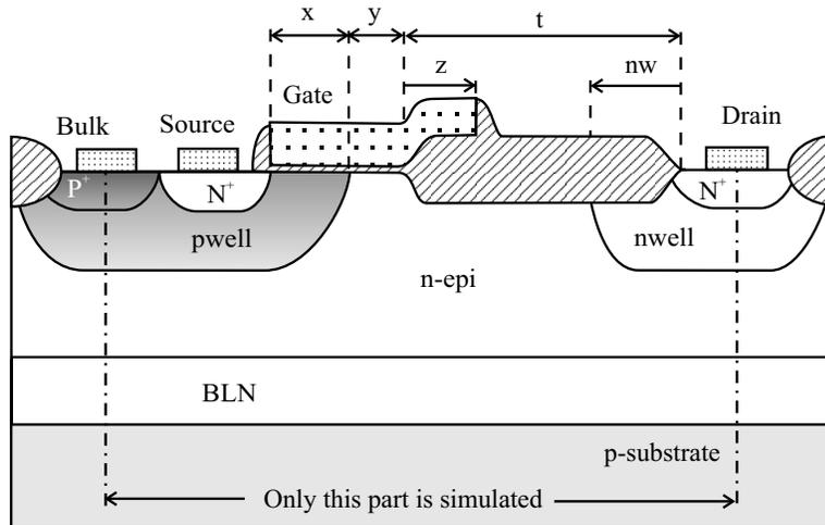
**Figure 4.26** A floating non-RESURF nLDEMOS device with BLN and its most important layout parameters.
