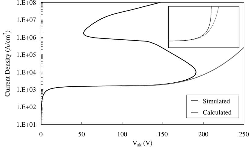
**Figure 2.1** Current density versus applied voltage for a silicon bar, simulated with the drift-diffusion model and calculated as explained in the text. The insert is a detail around the first breakdown on a lin-lin scale.
