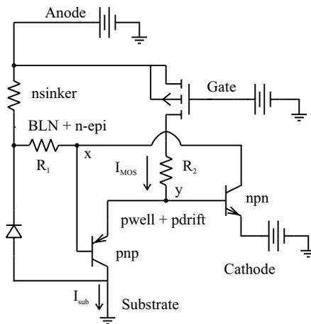
**Figure 5.42** Equivalent circuit for an pLIGBT.
