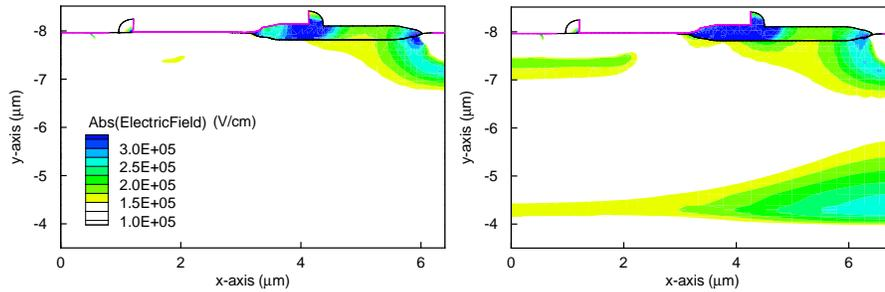
**Figure 4.25** Absolute value of the electric field at breakdown in the on-state ( $V_{gs} = 3.3 \text{ V}$ ) for a device with a lowly doped substrate ( $= 1e15 \text{ cm}^{-3}$  and  $N_{epi} = 6e15 \text{ cm}^{-3}$ , left) and a highly doped substrate ( $= 6e17 \text{ cm}^{-3}$  and  $N_{epi} = 8e15 \text{ cm}^{-3}$ ).
