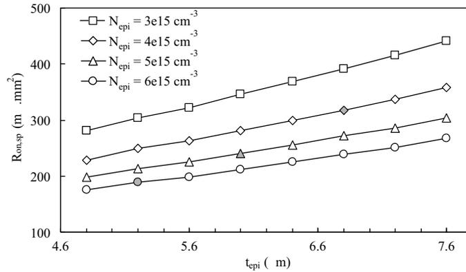
**Figure 4.21** Specific on-resistance of the RESURF nLDEMOS device with BLP as a function of epi thickness for several n-epi doping levels. Filled data points correspond to the optima in breakdown voltage (figure 4.20).
