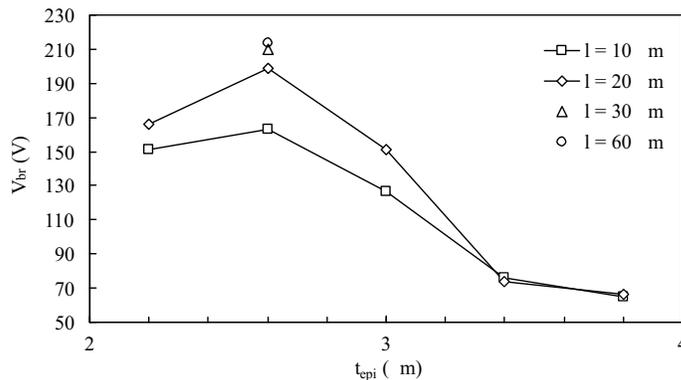
**Figure 4.8** Simulated breakdown voltage in a RESURF diode as a function of the epi thickness for the case where  $N_{sub} = 1e15 \text{ cm}^{-3} < N_{epi} = 4e15 \text{ cm}^{-3}$ .
