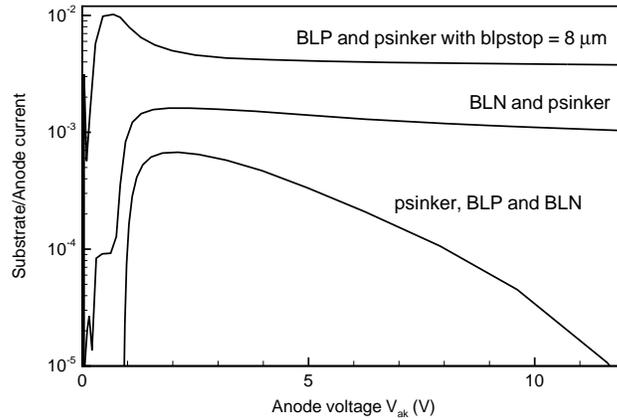
**Figure 5.26** Substrate to anode current ratio at  $V_{gk} = 3.3$  V for an LIGBT with psinker, BLP and floating BLN compared with previous designs.
