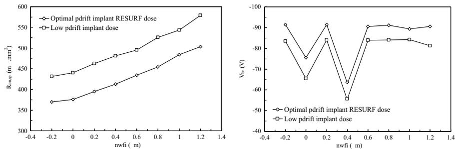
**Figure 4.43** *Measured*  $V_{br}$  and  $R_{on,sp}$  as a function of  $nwfi$  for two pdrift implant doses.
