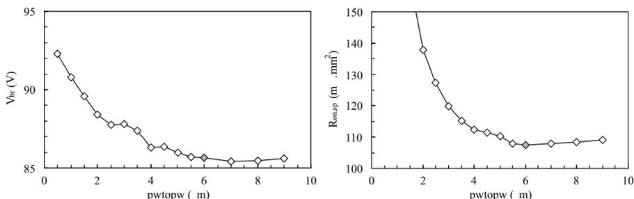
**Figure 4.33** Breakdown (left) and specific on-resistance of a floating nVDE-MOS with an optimal epi-thickness and doping level as a function of the layout parameter  $pwtow$ . Filled data points show the optimum.
