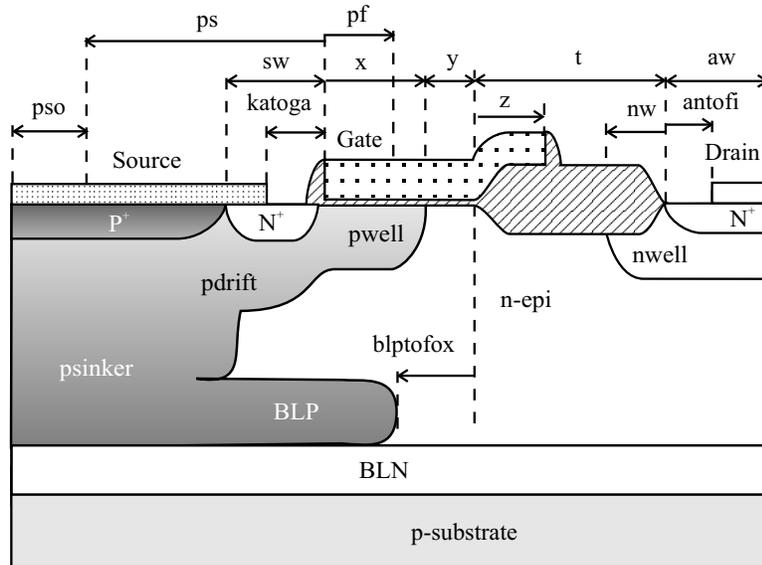
**Figure 4.29** A floating RESURF nLDEMOS device with BLN and BLP and all layout parameters defining the device.
