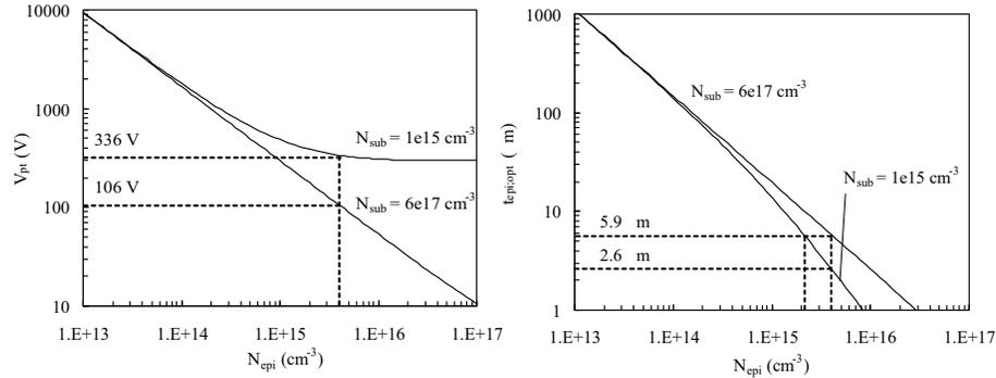
**Figure 4.7** The optimal RESURF punch-through breakdown voltage (left), and the optimal epi thickness as a function of the entire range of realistic n-epi doping levels for the cases with  $N_{sub} = 1e15 \text{ cm}^{-3}$  and  $N_{sub} = 6e17 \text{ cm}^{-3}$ .
