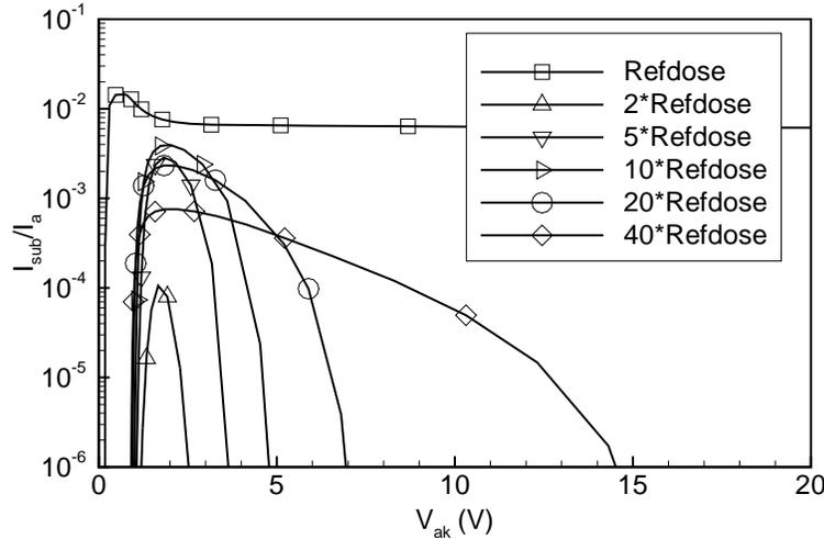
**Figure 5.33** Substrate to anode current ratio at  $V_{gk} = 3.3\text{ V}$  for several LIGBTs with different BLN doses. Note that the lowest dose yields a device without BLN and that the highest dose is the standard dose.
