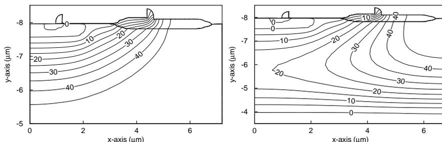
**Figure 4.27** Potential lines (5 V steps) at breakdown ( $V_{br} = 48$  V) for a floating nLDEMOS on top of a BLN (left) with a  $N_{epi} = 8e15$  cm $^{-3}$ . The figure on the right shows the optimal nLDEMOS on top of a BLP with the same n-epi doping level at the same biasing conditions (far below breakdown for this RESURF structure).
