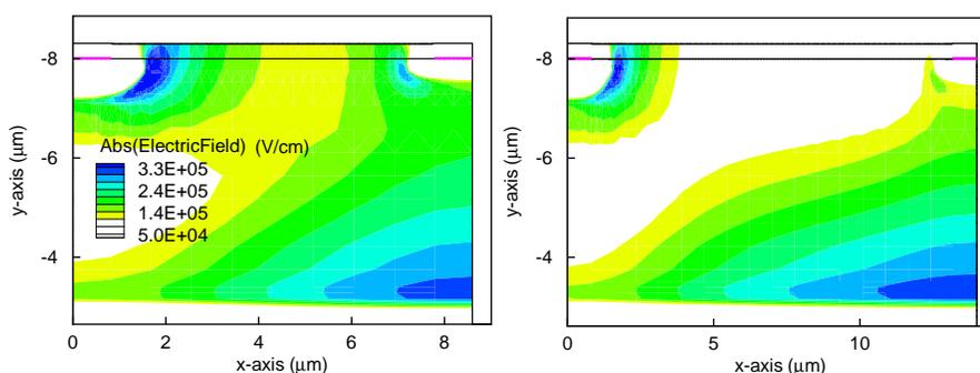
**Figure 4.10** Electric field (in absolute value) distribution for two RESURF diodes with optimal epi thickness ( $t_{epi} = 5.2\ \mu\text{m}$ ) and  $N_{sub} = 6e17\ \text{cm}^{-3} > N_{epi} = 4e15\ \text{cm}^{-3}$ . The diode on the left has a  $l = 6.6\ \mu\text{m}$  and the diode on the right  $l = 12\ \mu\text{m}$ .
