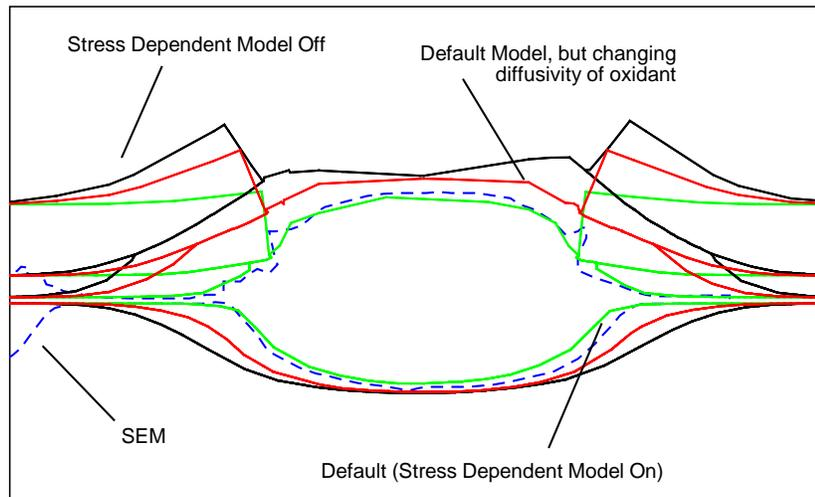
**Figure 3.4** Comparison of different oxidation models with SEM picture.
