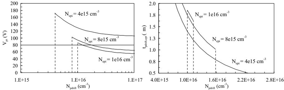
**Figure 4.36** Punch-through breakdown of the vertical diode in a pLDEMOS as a function of the pdrift doping level at several n-epi doping levels (left). The optimal RESURF pdrift thickness for the pdrift doping levels corresponding to a  $V_{pt} > 80$  V and satisfying the condition  $N_{pdrift} > N_{epi}$  (right).
