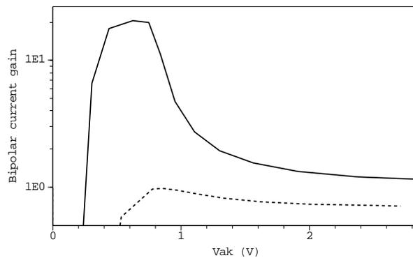
**Figure 5.15** The common-emitter current gain  $\beta$  at  $V_{gk} = 3.3$  V of an IGBT as shown in figure 5.13 (solid line) compared with an IGBT of the previous section (with pdrift).
