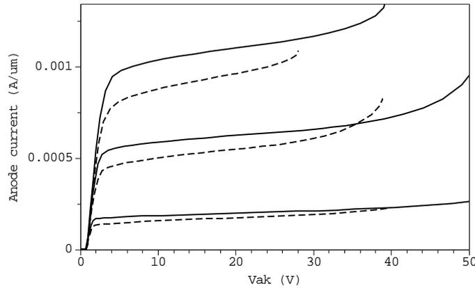
**Figure 5.21** Output characteristics at  $V_{gk} = 1.1, 2.2$  and  $3.3\ \text{V}$  of a non-floating nIGBT (figure 5.19 with  $\text{blpstop} = 8\ \mu\text{m}$ , solid lines) compared with a floating nIGBT with BLN and psinker (figure 5.13).
