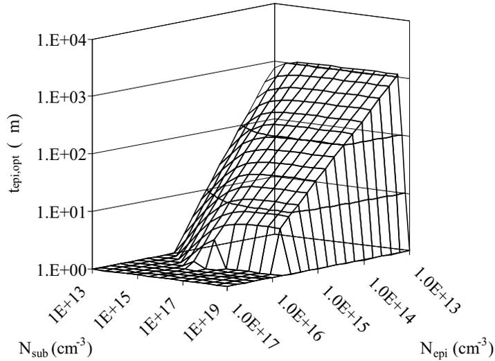
**Figure 4.4** Optimal RESURF epi thicknesses larger than  $1\ \mu\text{m}$  and corresponding to an ideal RESURF breakdown larger than  $80\ \text{V}$  for the entire range of realistic n-epi and p-substrate doping levels.
