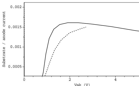
**Figure 5.16** Substrate to anode current ratio at  $V_{gk} = 3.3\text{ V}$  of an LIGBT as shown in figure 5.13 (solid line) compared with an LIGBT of the previous section (with pdrift).
