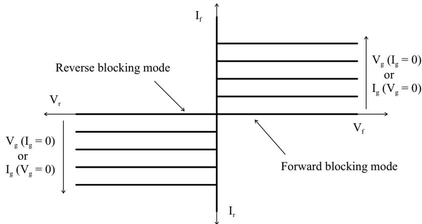
**Figure 2.7** Output characteristics (forward and reverse) of an ideal switch.
