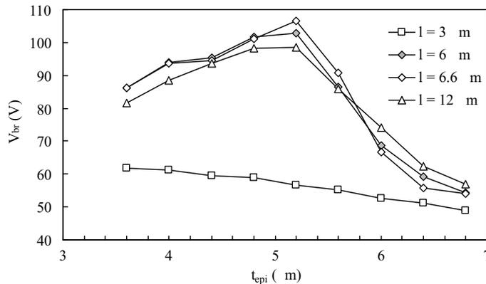
**Figure 4.9** Simulated breakdown voltage in a RESURF diode as a function of the epi thickness for the case where  $N_{sub} = 6e17 \text{ cm}^{-3} > N_{epi} = 4e15 \text{ cm}^{-3}$ .
