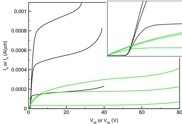
**Figure 5.14** Output characteristics at  $V_{gk} = 1.1, 2.2$  and  $3.3$  V of an IGBT as shown in figure 5.13 (black) compared with a typical VDEMOS (grey). The inset shows the important region at low  $V_{ak}$  (or  $V_{ds}$ ) values.
