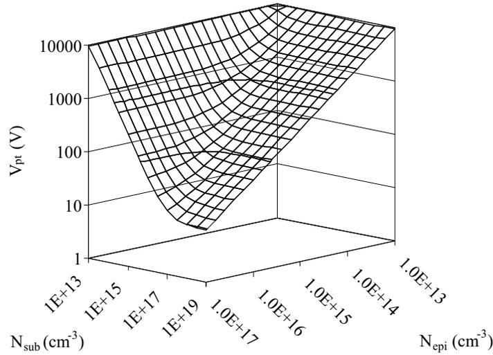
**Figure 4.3** Breakdown in an ideal RESURF diode is given by the vertical diode punch-through breakdown voltage and is a function of the n-epi and p-substrate doping levels.
