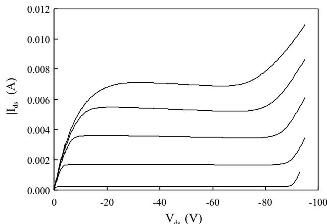
**Figure 4.44** Measured  $I_d(V_{ds})$  characteristics at  $V_{gs} = -1.1, -2.2 \dots -5.5$  V of a pLDEMOS (width  $W = 40$   $\mu\text{m}$ ) under optimal RESURF conditions.
