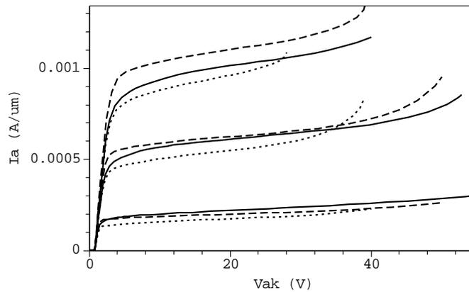
**Figure 5.24** Output characteristics at  $V_{gk} = 1.1, 2.2$  and  $3.3\text{ V}$  of a floating nLIGBT (figure 5.23, solid lines) compared with a non-floating nLIGBT (figure 5.19 with  $\text{blpstop} = 8\text{ }\mu\text{m}$ , long dashed) and with a floating nLIGBT with BLN and psinker (figure 5.13, short dashed).
