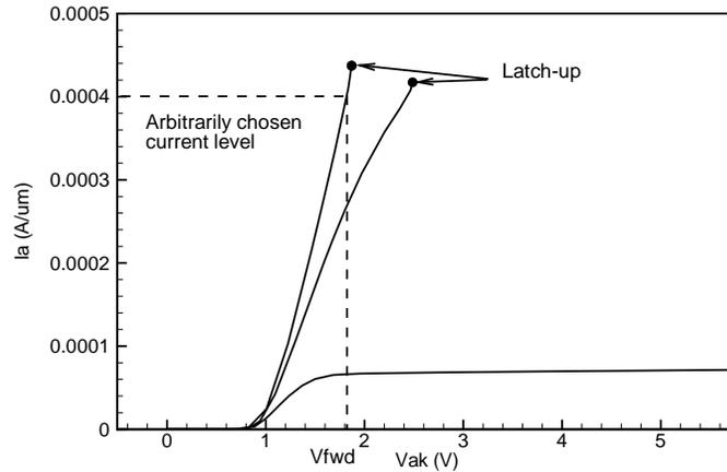
**Figure 5.6** Output characteristics at  $V_{gk} = 1.1, 2.2$  and  $3.3 \text{ V}$  of an LIGBT with a nbuffer dose of  $1e15 \text{ cm}^{-2}$  of table 5.1.
