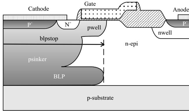
**Figure 5.19** The non-floating LIGBT device with psinker and BLP. One extra layout parameter in comparison with figure 5.13 is needed here: blpstop.
