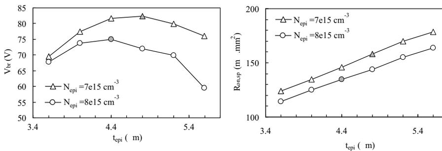
**Figure 4.22** Breakdown voltage (left) and specific on-resistance of the RESURF nLDEMOS device with BLP as a function of epi thickness for the highest possible n-epi doping levels. Filled data points are the optima for each doping level.
