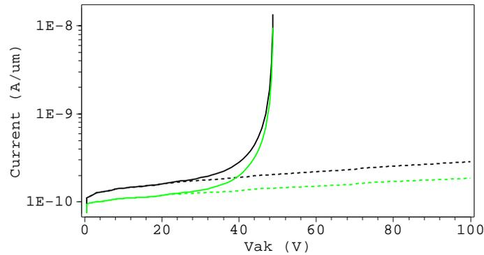
**Figure 5.4** Current through the anode (black) and substrate (green) contacts of a large LIGBT before and at breakdown. Solid lines are simulated with impact ionization, dashed ones without.
