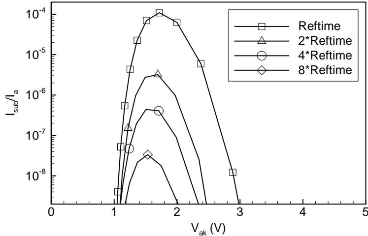
**Figure 5.34** Substrate to anode current ratio versus  $V_{ak}$  (at  $V_{gk} = 3.3$  V) for different BLN anneal times (BLN dose =  $2 * Refdose$ ). *Reftime* is the standard anneal time as used in figure 5.33.
