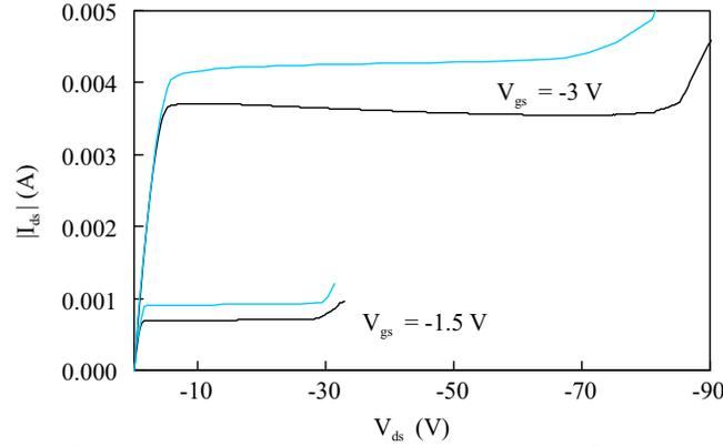
**Figure 4.45**  $I_d(V_{ds})$  characteristics at  $V_{gs} = -1.5$  and  $-3.0$  V of an “under resurfed” device (width  $W = 40 \mu\text{m}$ ): *measured* (black) versus simulated (blue).
