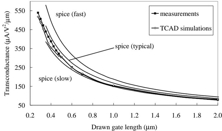
**Figure 3.9** Transconductance per  $\mu\text{m}$  width versus drawn channel length for nMOS transistors: comparison between measurements, TCAD and SPICE simulations.
