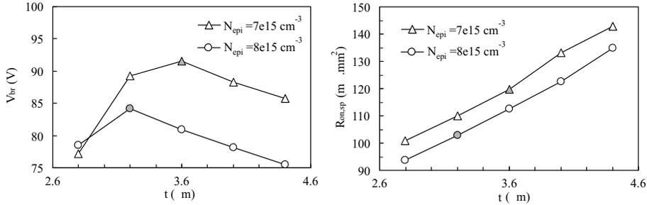
**Figure 4.23** Breakdown voltage (left) and specific on-resistance of the RESURF nLDEMOS device with BLP as a function of the field oxide length  $t$  for the highest possible n-epi doping levels. Filled data points are the optima for each doping level.
