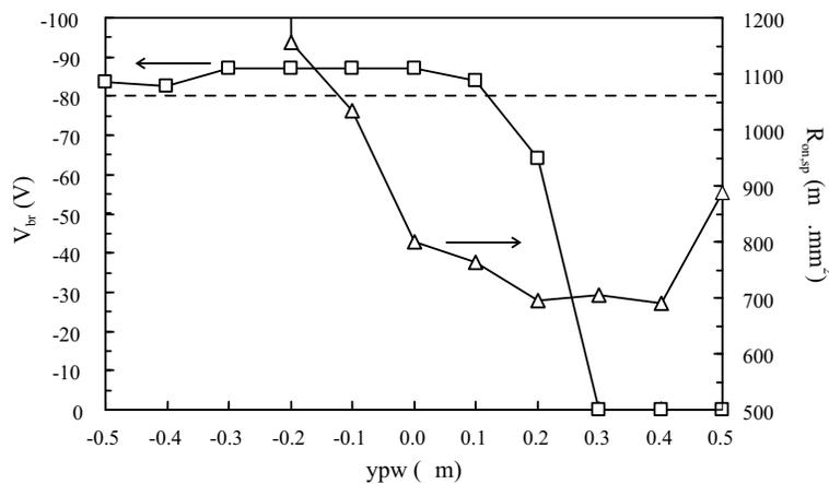
**Figure 4.38** *Measured*  $V_{br}$  and  $R_{on,sp}$  as a function of  $ypw$ .
