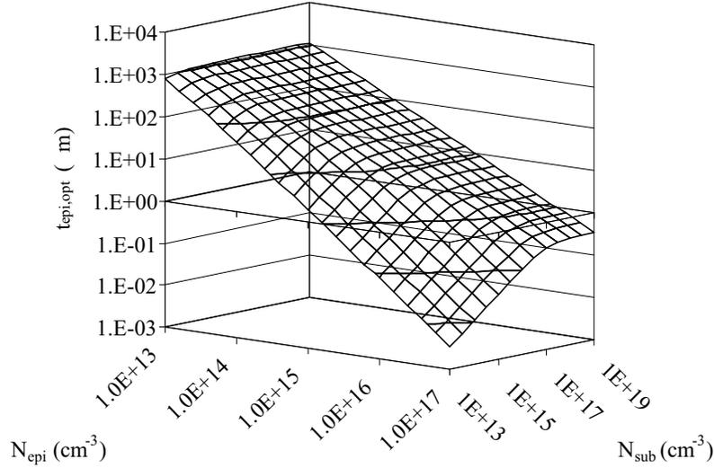
**Figure 4.2** Optimal RESURF epi thicknesses for the entire range of realistic n-epi and p-substrate doping levels.
