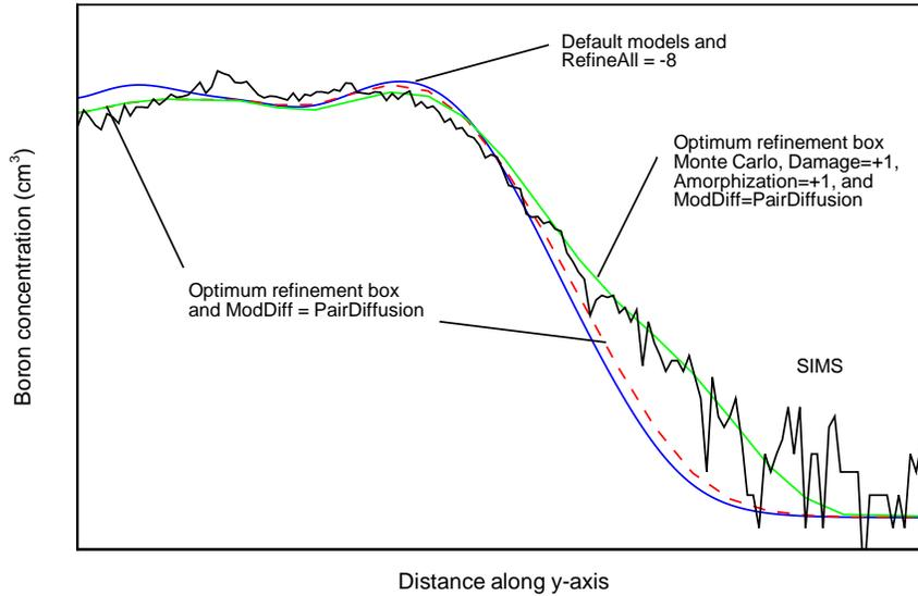
**Figure 3.5** Comparison of SIMS profile of the pwell after gate oxidation in active area with several simulation results.
