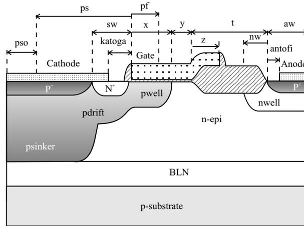
**Figure 5.13** The LIGBT device with BLN, psinker, and pdrift. Note the introduction of a set of new parameters, of which the definition should be clear from the figure. Except maybe the opening in the psinker mask,  $pso$ .
