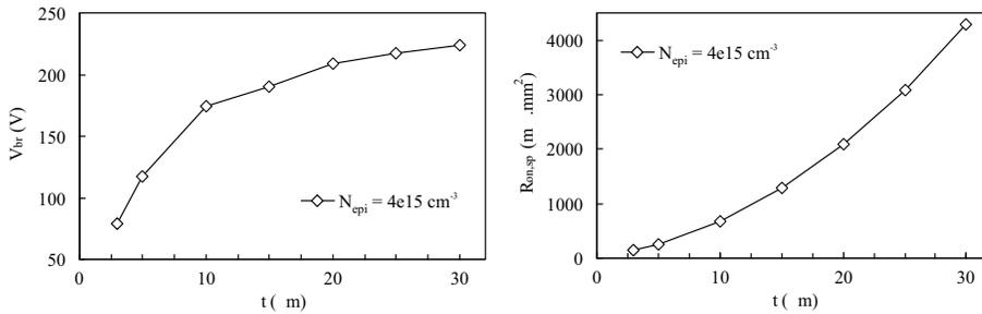
**Figure 4.18** Breakdown voltage (left) and specific on-resistance (right) of the “free” RESURF nLDEMOS device as a function of the field oxide length  $t$  for one chosen optimal RESURF case ( $t_{epi} = 3.4 \mu\text{m}$  and  $N_{epi} = 4e15 \text{ cm}^{-3}$ ).
