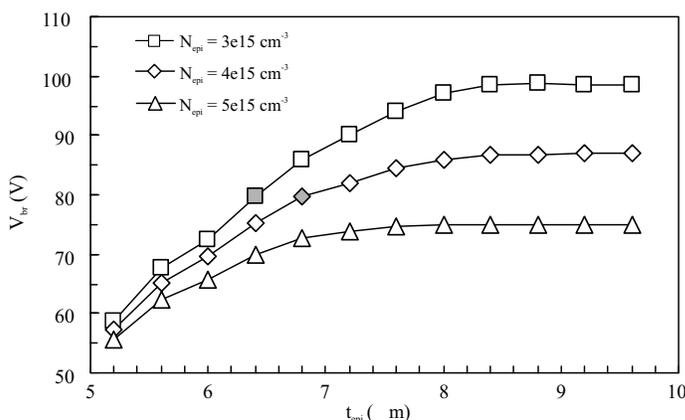
**Figure 4.31** Breakdown of a floating nVDEMOS with an optimal  $pwtow$  as a function of the n-epi thickness for the highest possible n-epi doping levels. Filled data points indicate the devices with a breakdown voltage over 80 V with the lowest specific on-resistance for each doping level.
