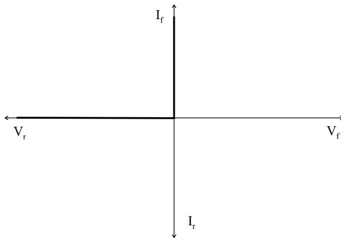
**Figure 2.4** Output characteristic (forward and reverse) of an ideal diode.
