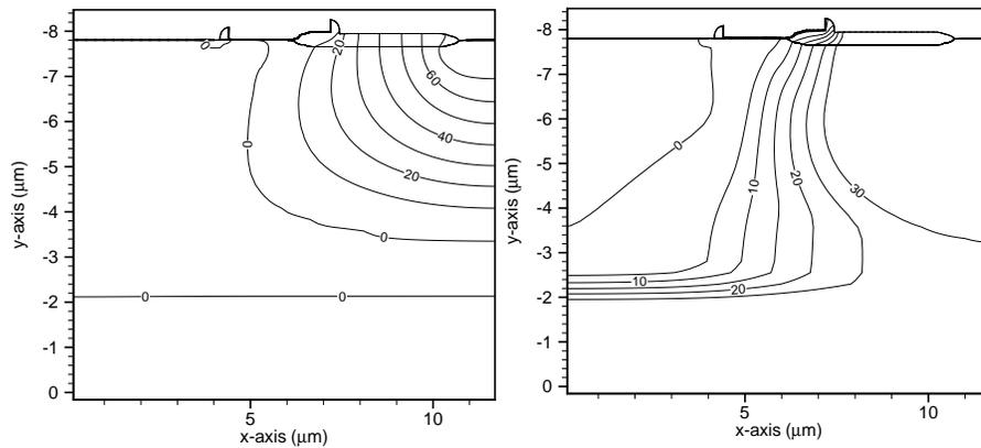
**Figure 5.25** Electrostatic potential distribution (V) in the off-state (left) and the on-state (right) for a nLIGBT with psinker, BLP and BLN.
