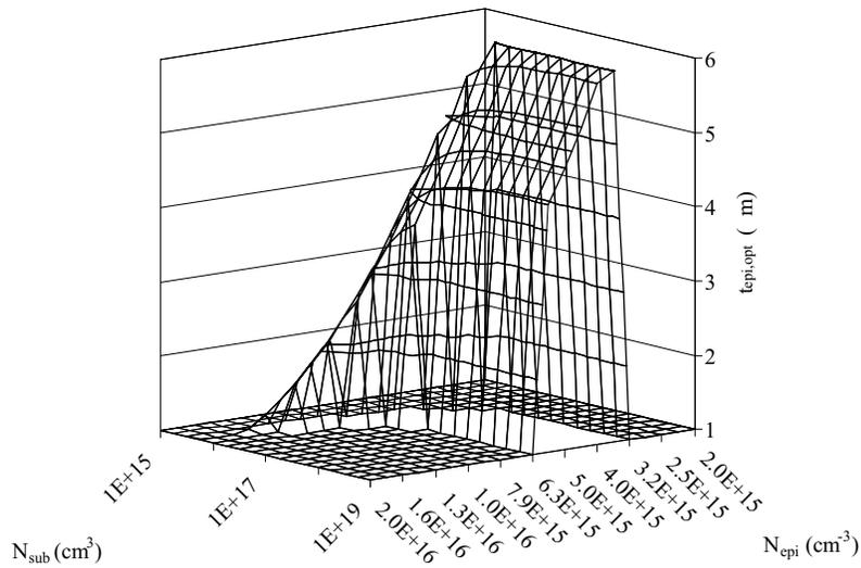
**Figure 4.5** Optimal RESURF epi thicknesses larger than  $1\ \mu\text{m}$  and corresponding to an ideal RESURF breakdown between  $80\ \text{V}$  and  $120\ \text{V}$ .
