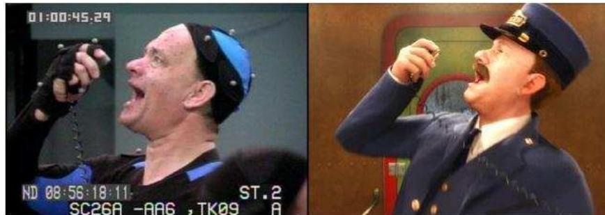
*Figure 1.2: The posture of the person on the left is captured using an optical system and mapped to a computer generated character on the right.*
