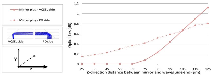
Figure 7.7: Optical loss simulation in function of the Z-distance between the micro-mirror and the start/end of the waveguide.
