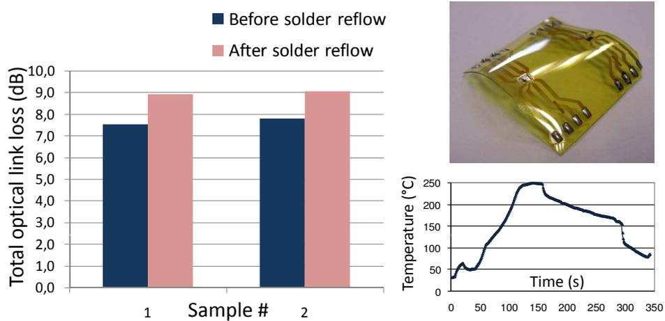
Figure 8.23: Total optical link loss changes and substrate deformation due to exposure to a standard solder reflow temperature cycle.
