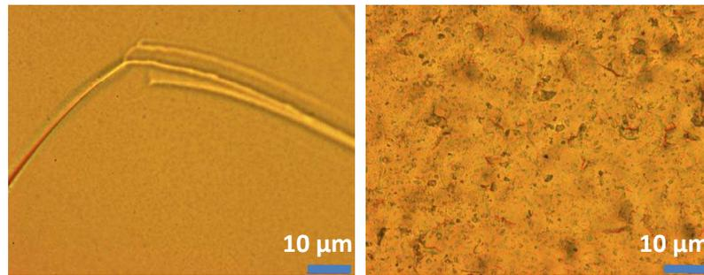
**Figure 4.11:** Microscopic picture of the surface of an untreated UPILEX S-25 Polyimide foil (left, the scratch is intentional to focus the microscope) and the same foil after sandblasting (right).
