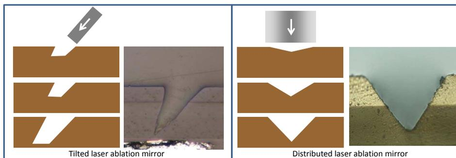
**Figure 7.14:** Schematic comparison and cross-sections of the tilted laser ablation mirror and the distributed laser ablation mirror.
