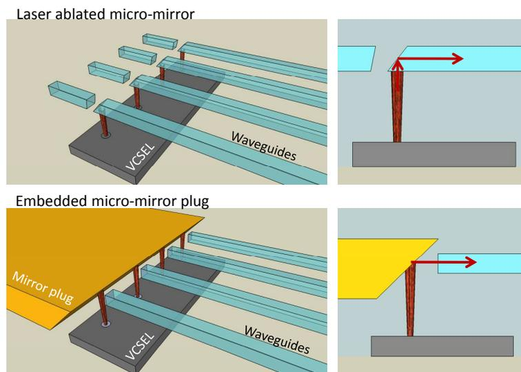
**Figure 7.1:** Schematic explanation of the difference between the laser ablated micro-mirror and the mirror plug approach.
