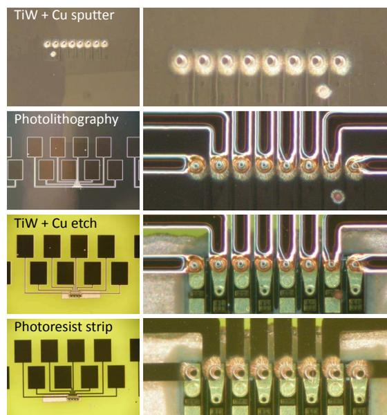
**Figure 6.11:** Process flow for the metallization of  $\text{CO}_2$  laser ablated via's and fan-out from and to embedded opto-electronics in SU-8.
