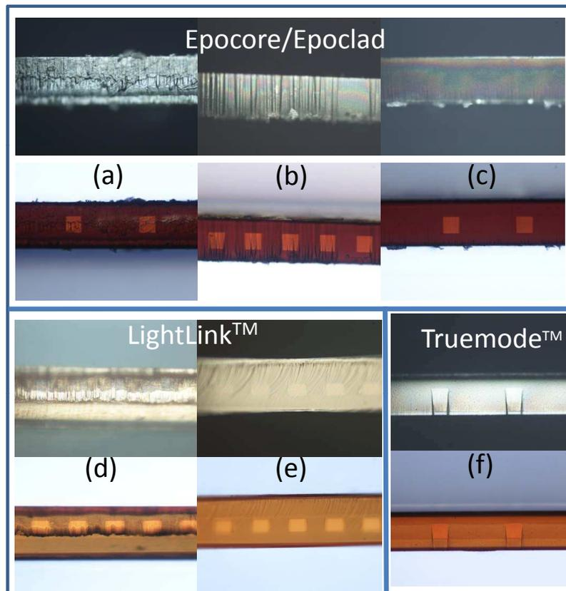
**Figure 4.18:** Picture matrix of flexible waveguide facets fabricated with different techniques and different parameters for Truemode™ Backplane Polymer , LightLink™ and Ormocers® materials
