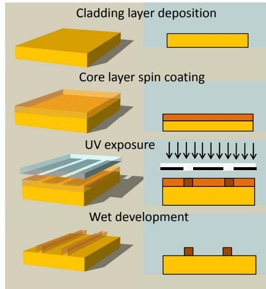
**Figure 3.9:** Schematic process flow for the fabrication of photolithographic optical waveguides.
