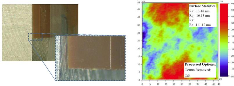
Figure 7.22: Picture of the mirror facet on the PI motherpiece (left) and a WYKO optical non-contact profilometer plot of the mirror surface (right).
