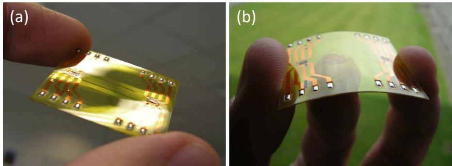
Figure 8.16: Finalized flexible active optical link substrate flat (a) and bended (b).
