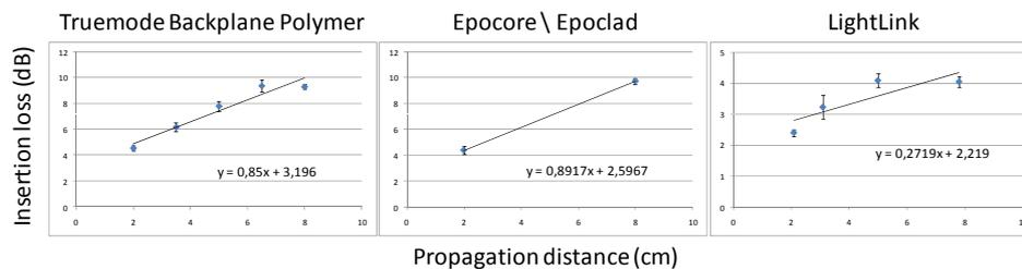
**Figure 4.19:** Cut-back optical waveguide propagation loss measurements for Truemode™ Backplane Polymer , Epocore / Epoclad and LightLink™ flexible waveguides.
