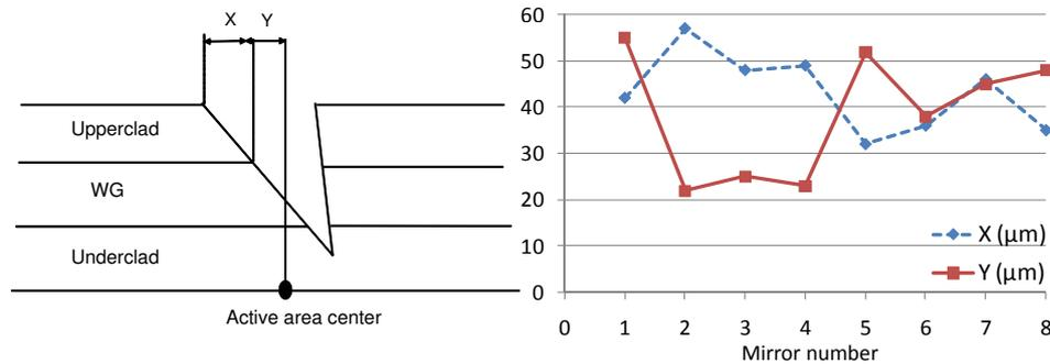
**Figure 7.17:** Misalignment of the laser ablated mirror with respect to the embedded actives due to the variation in uppercladding layer thickness.
