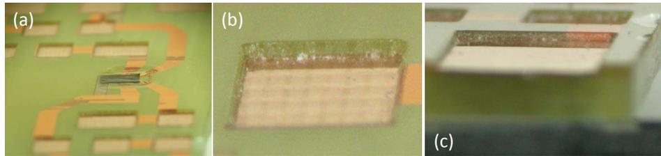
**Figure 8.9:** Pictures of the laser ablation opened contact pads in the middle of the substrate for SMD components (a & b) and at the edge for side launch coaxial SMA connectors (c).
