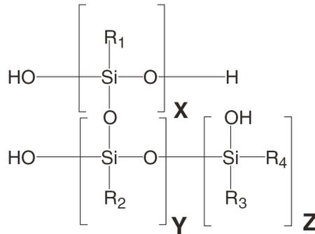
Figure 2.4: Inorganic / organic polymer backbone of LightLink™ .
