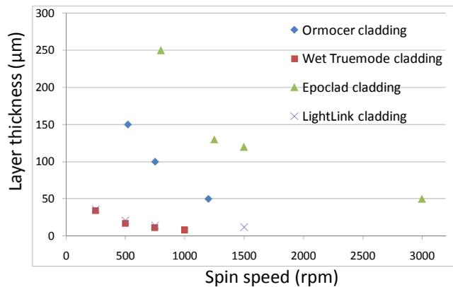
Figure 3.4: Layer thickness versus spin speed for 4 cladding materials on top of an FR4 substrate.
