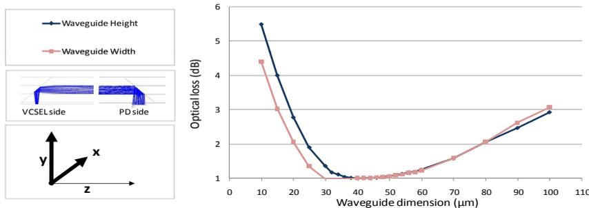
Figure 7.9: Optical loss simulation in function of the waveguide height and width.
