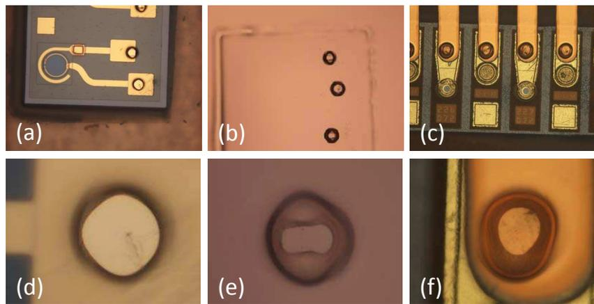
**Figure 6.8:** Pictures of Excimer laser ablated via's to embedded opto-electronic components
