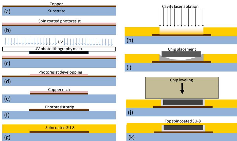
**Figure 6.1:** Process flow for the embedding of ultra thin opto-electronics in SU-8 material
