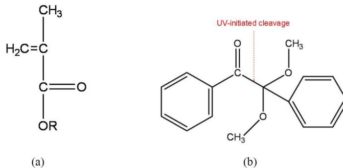
**Figure 2.3:** Basic structure of methacrylate (a) and of the photo-initiator Irgacure651 for the Truemode™ Backplane Polymer material.
