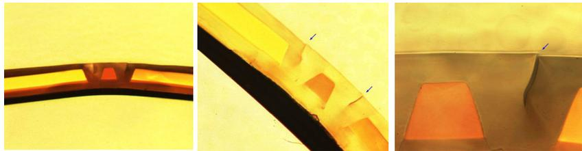
**Figure 4.13:** Damage of the optical layers at the waveguides due to a local peak in tensile stress in a Truemode™ Backplane Polymer waveguide stack on top of a Polyimide foil.
