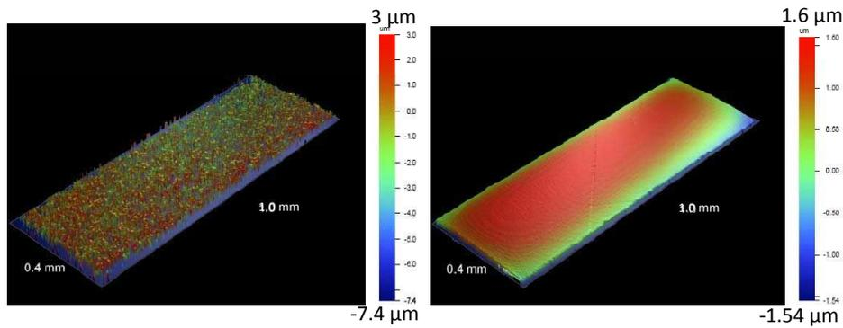
**Figure 5.12:** Backside profile measurement with a non-contact profilometer WYKO of a lapped (left) and a polished (right) 1 x 4 VCSEL array
