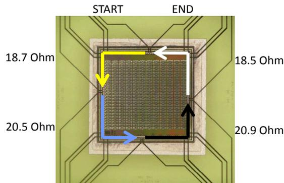
Figure 6.28: Daisy chain resistance measurement for the the four quarters of the embedded die.
