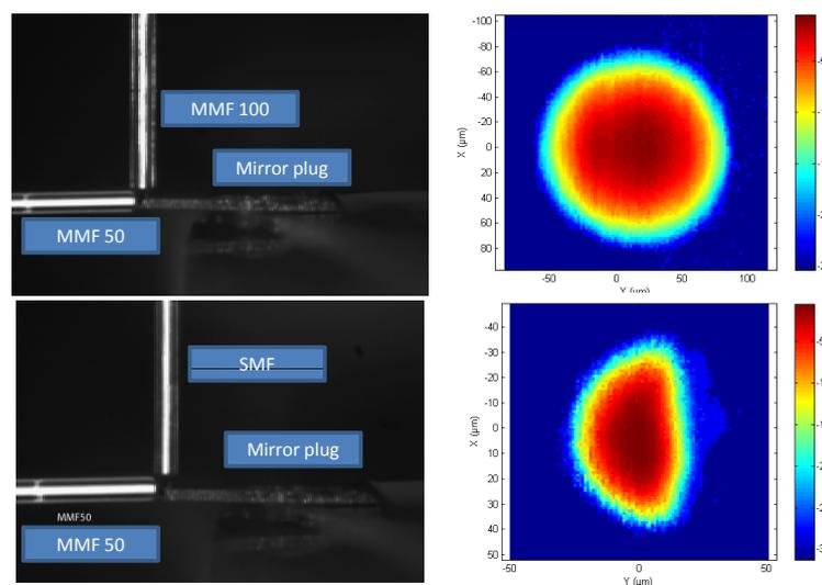
**Figure 7.25:** Coupling efficiency measurements CCD camera pictures (left) and tolerance plots for the detecting fiber scan (top right) and the emitting fiber scan (bottom right).
