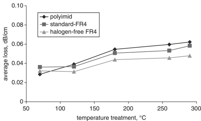
**Figure 4.1:** Thermal stability of waveguide foils transmission loss @ 850 nm using different PCB laminates. (source: University of Dortmund).
