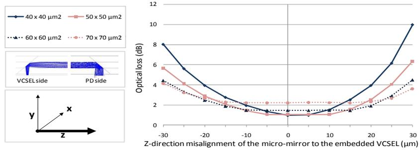
**Figure 7.10:** Optical loss simulation in function of the Z-misalignment of the micro-mirror with respect to the embedded VCSEL's for different waveguide dimensions.
