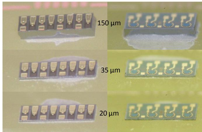
**Figure 5.11:** VCSEL arrays (left) and Photodiode arrays (right) in non-thinned status (top) and after lapping and polishing (center and bottom)
