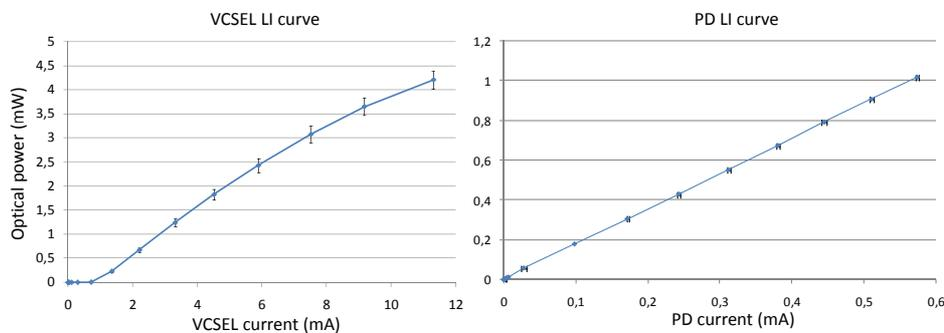
**Figure 8.1:** LI curve of an ULM Photonics 850 nm VCSEL ULM850-05-TT-C0104U (left) and a AlbisOptoelectronics photodiode PDCA04-70-GS (right).
