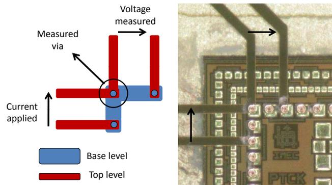
Figure 6.29: 4-points measurement schematic explanation (left) and picture of this principle applied to an embedded IC (right).
