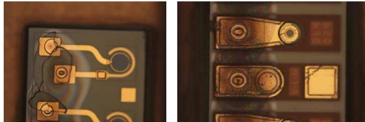
Figure 6.22: Pictures showing the local delamination around the laser ablated micro-via's, using PI2525 as an intermediate adhesion layer.
