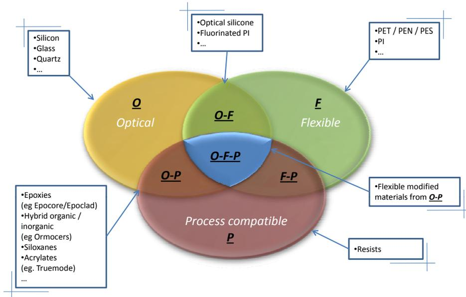
**Figure 2.1:** Venn diagram of the material market, benchmarked according to the proposed material requirements.
