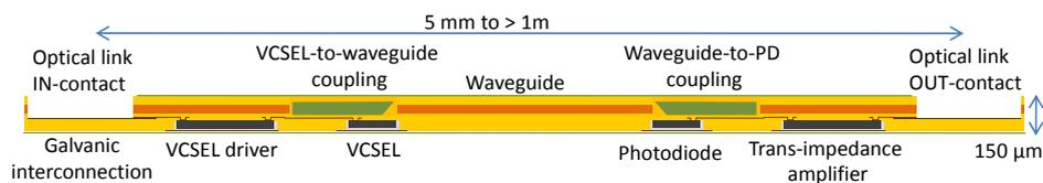
**Figure 1.1:** Overview on the cross-section of the different embedded components inside the active optical waveguide foil.
