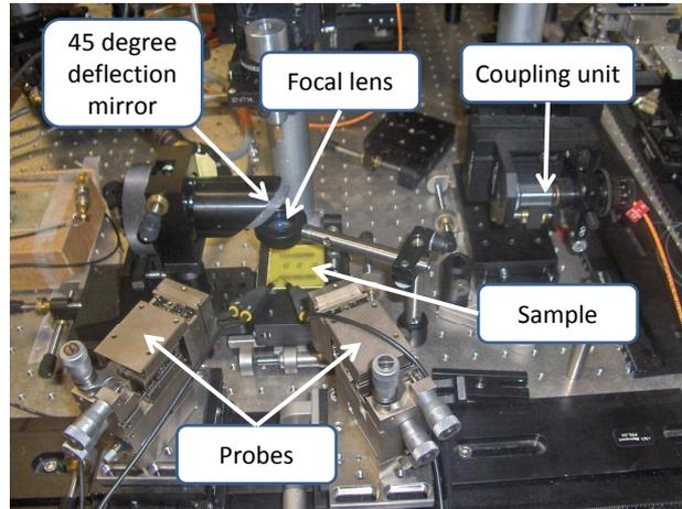
Figure 5.21: Optical measurement set-up for the characterization of thinned VCSELs
