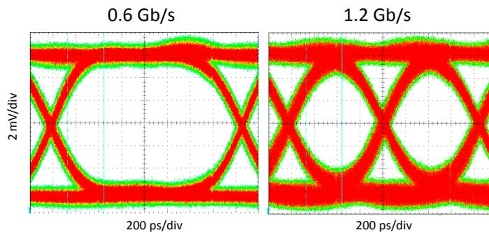
**Figure 8.14:** Eye diagram for 0.6 and 1.2 Gb/s for the embedded active optical link.
