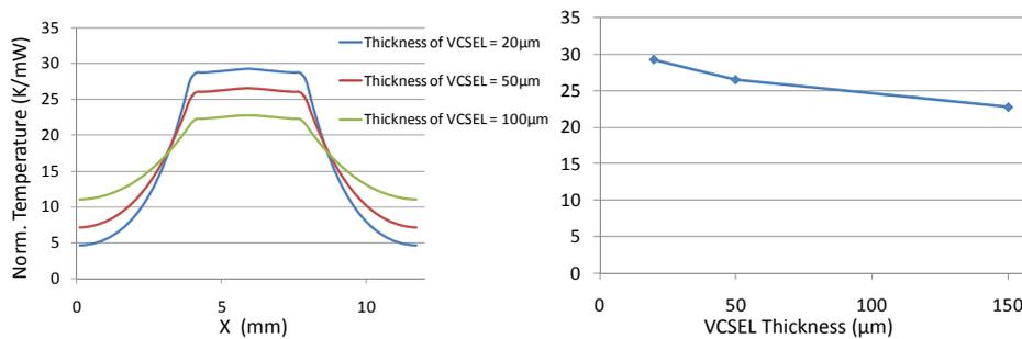
**Figure 8.27:** Normalized temperature distribution along the X-axis (left) and normalized VCSEL temperature (right) in function of the VCSEL thickness.
