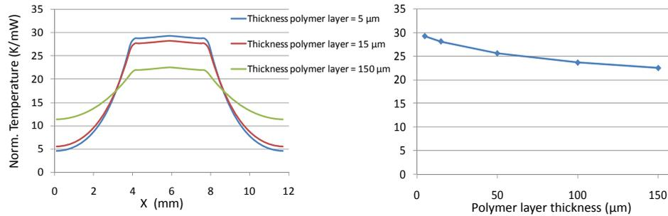
**Figure 8.28:** Normalized temperature distribution along the X-axis (left) and normalized VCSEL temperature (right) in function of the polymer thickness above the VCSEL.
