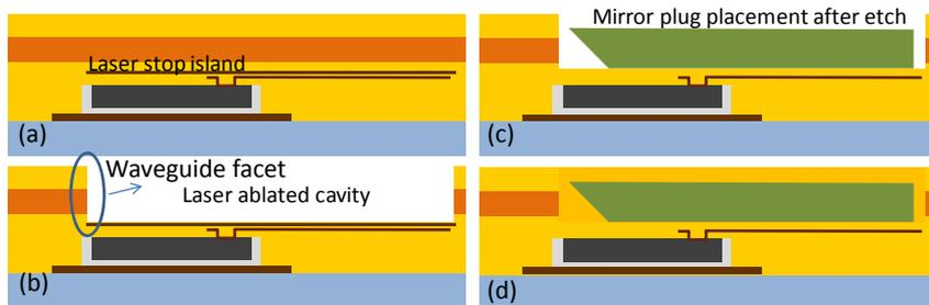
**Figure 7.28:** Schematic cross-sectional process flow for the embedding of mirror plugs into the layer build-up of the embedded optical link.
