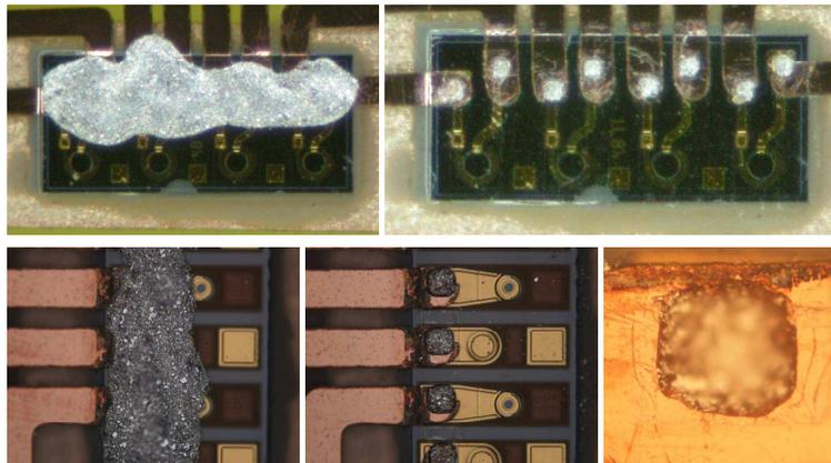
Figure 6.21: Metal paste via filling pictures.
