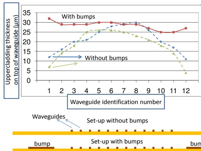
**Figure 3.21:** Schematic sketch of the bump principle for the reproducibility of the uppercladding thickness on top of the waveguides (bottom) and the uppercladding thickness for 12 different waveguides in a  $1 \times 12$  waveguide array for bumped and non-bumped waveguide fabrication (top).
