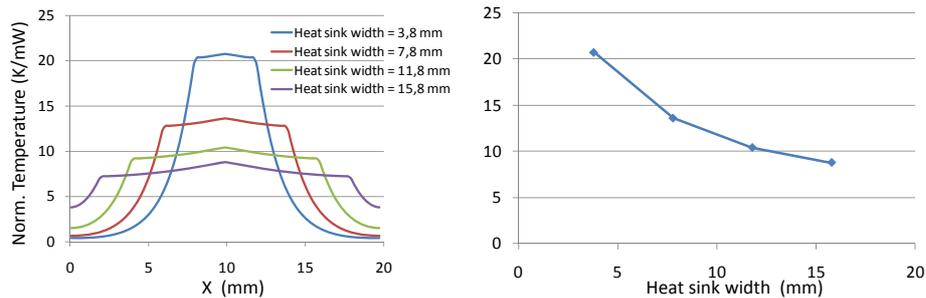
**Figure 8.25:** Normalized temperature distribution along the X-axis (left) and normalized VCSEL temperature (right) in function of the heat sink width.
