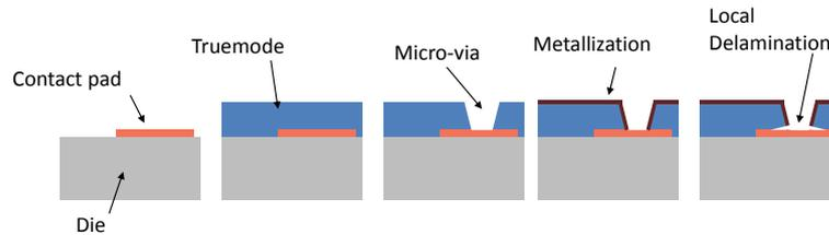
**Figure 6.18:** Schematic overview of the contact delamination problem during the embedding of actives inside Truemode™ Backplane Polymer material.
