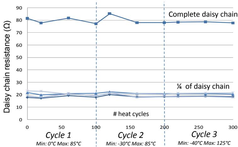
Figure 8.20: Evolution of the daisy chain resistance of an embedded IC on a rigid FR-4 board during temperature cycling.
