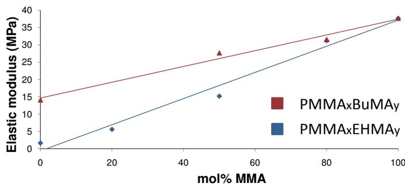
Figure 2.6: Elastic modulus of PMMAxBuMAy and PMMAxEHMAy.
