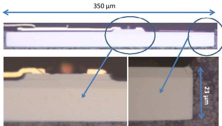
**Figure 5.15:** Cross-section of a lapped and polished VCSEL array and close-ups.
