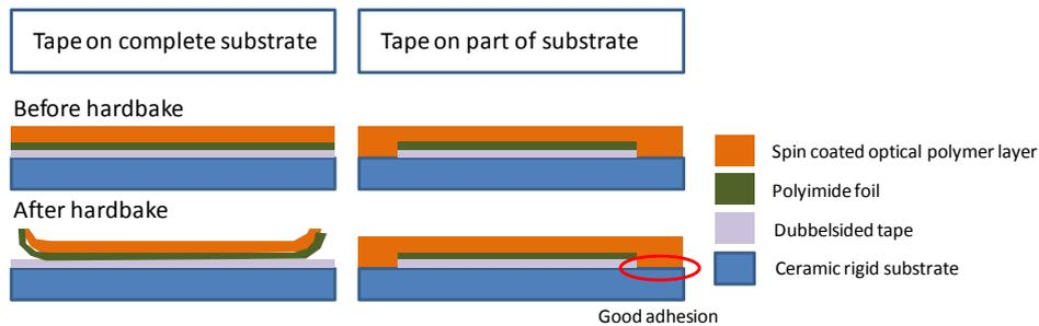
**Figure 4.9:** Edge adhesion approach for mounting of a Polyimide foil on top of a rigid substrate.
