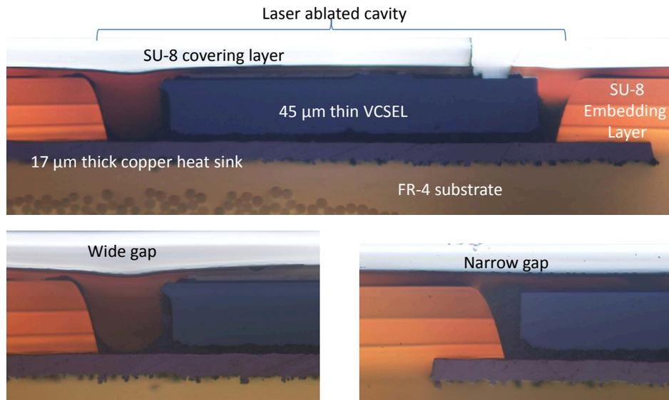
**Figure 6.5:** Cross-sectional photograph of a fully embedded 45  $\mu\text{m}$  thin VCSEL inside SU-8 material and a close-up on the filling of the VCSEL-cavity gap for a narrow and a wider gap.
