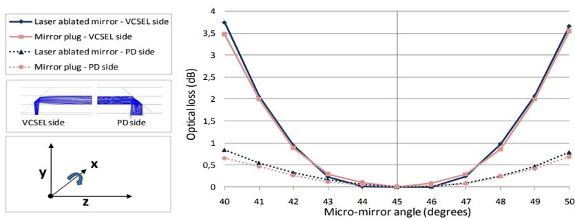
Figure 7.8: Optical loss simulation in function of the micro-mirror angle.
