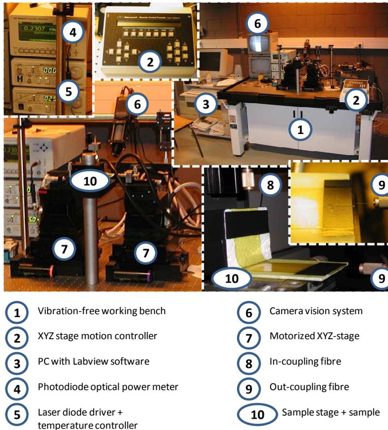
**Figure 4.17:** Newport optical measurement bench set-up for waveguide optical loss measurements.
