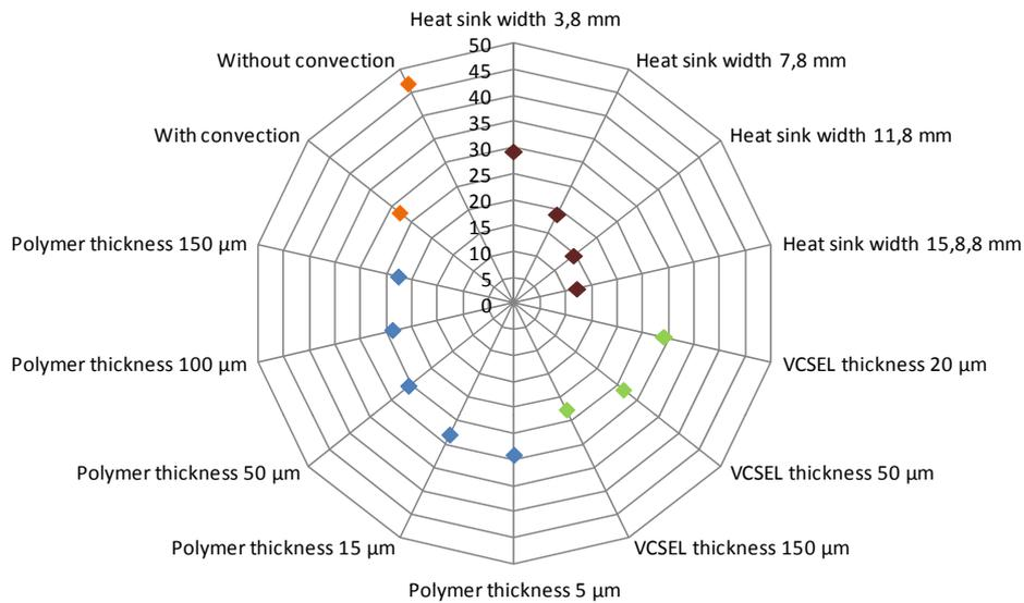
**Figure 8.29:** Overview of the influence of all studied parameters on the VCSEL normalized temperature.
