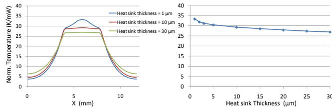
**Figure 8.26:** Normalized temperature distribution along the X-axis (left) and normalized VCSEL temperature (right) in function of the heat sink thickness.
