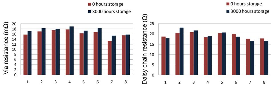
Figure 8.22: Via resistance and daisy chain resistance for an embedded IC on a rigid FR-4 board right after fabrication and after 4 months storage at room temperature and nominal room humidity.
