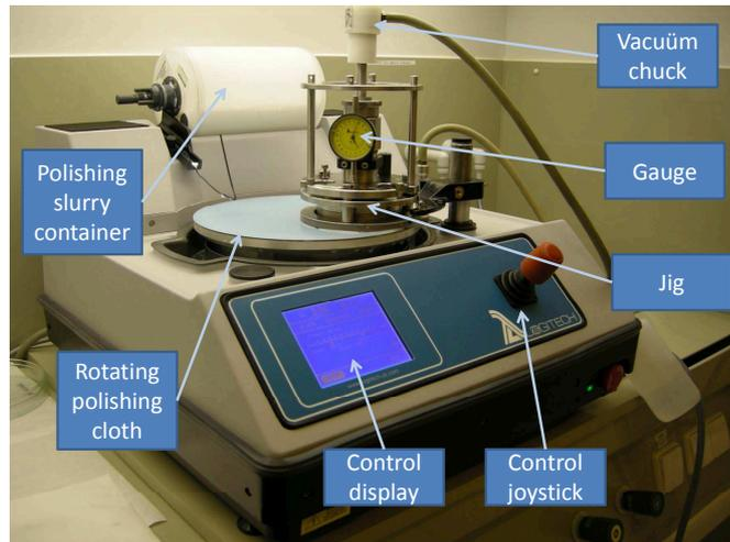
**Figure 5.6:** Logitech PM5 Precision Lapping & Polishing Machine as installed in the clean-room
