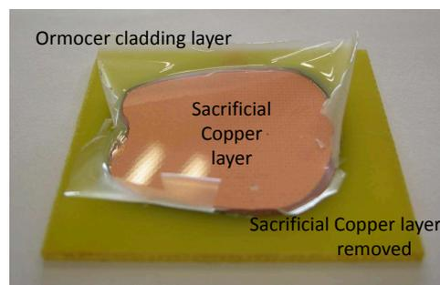
**Figure 4.3:** Partly released Ormocers® cladding layer processed on a copper coated FR4 board.
