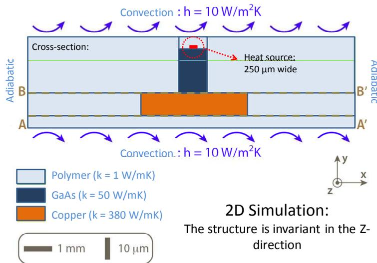
Figure 8.24: Two dimensional cross-sectional model overview.
