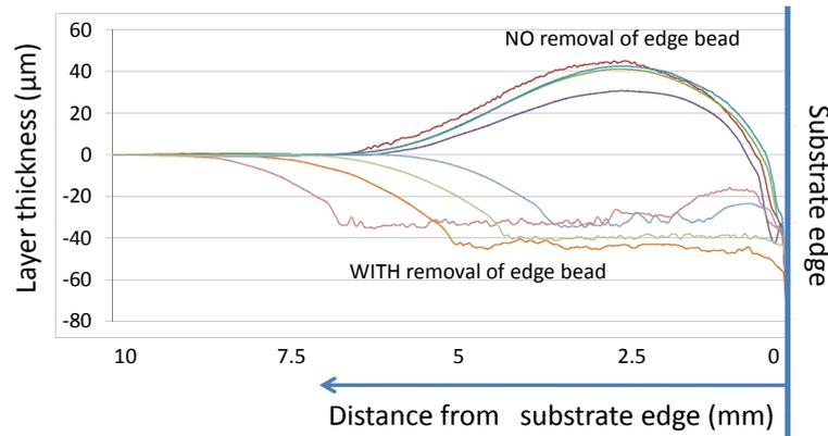
**Figure 3.2:** Edge layer thickness of wet film Truemode™ Backplane Polymer with and without edge bead removal (target layer thickness = 40 µm )
