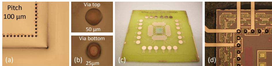
Figure 6.27: Pictures of the embedded IC (a) and the Excimer laser ablated micro-via's (b) after sputtering (a & b) and after etching (c & d).
