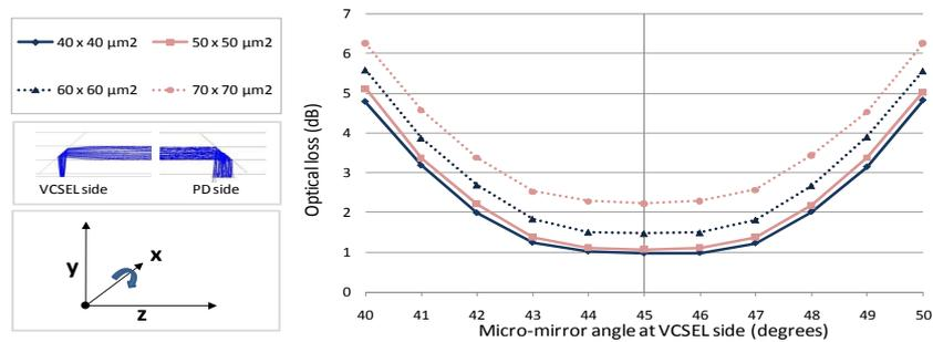
**Figure 7.12:** Optical loss simulation in function of micro-mirror facet angle for different waveguide dimensions.
