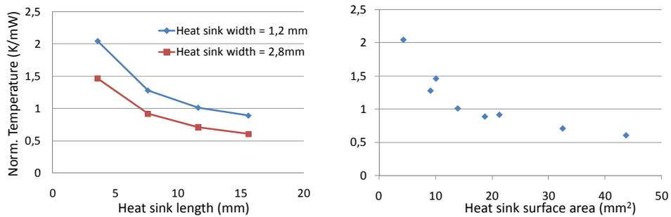
**Figure 8.32:** Normalized VCSEL temperature in function of the heat sink length for 2 different heat sink widths (left) and normalized VCSEL temperature in function of the heat sink total surface area (right).
