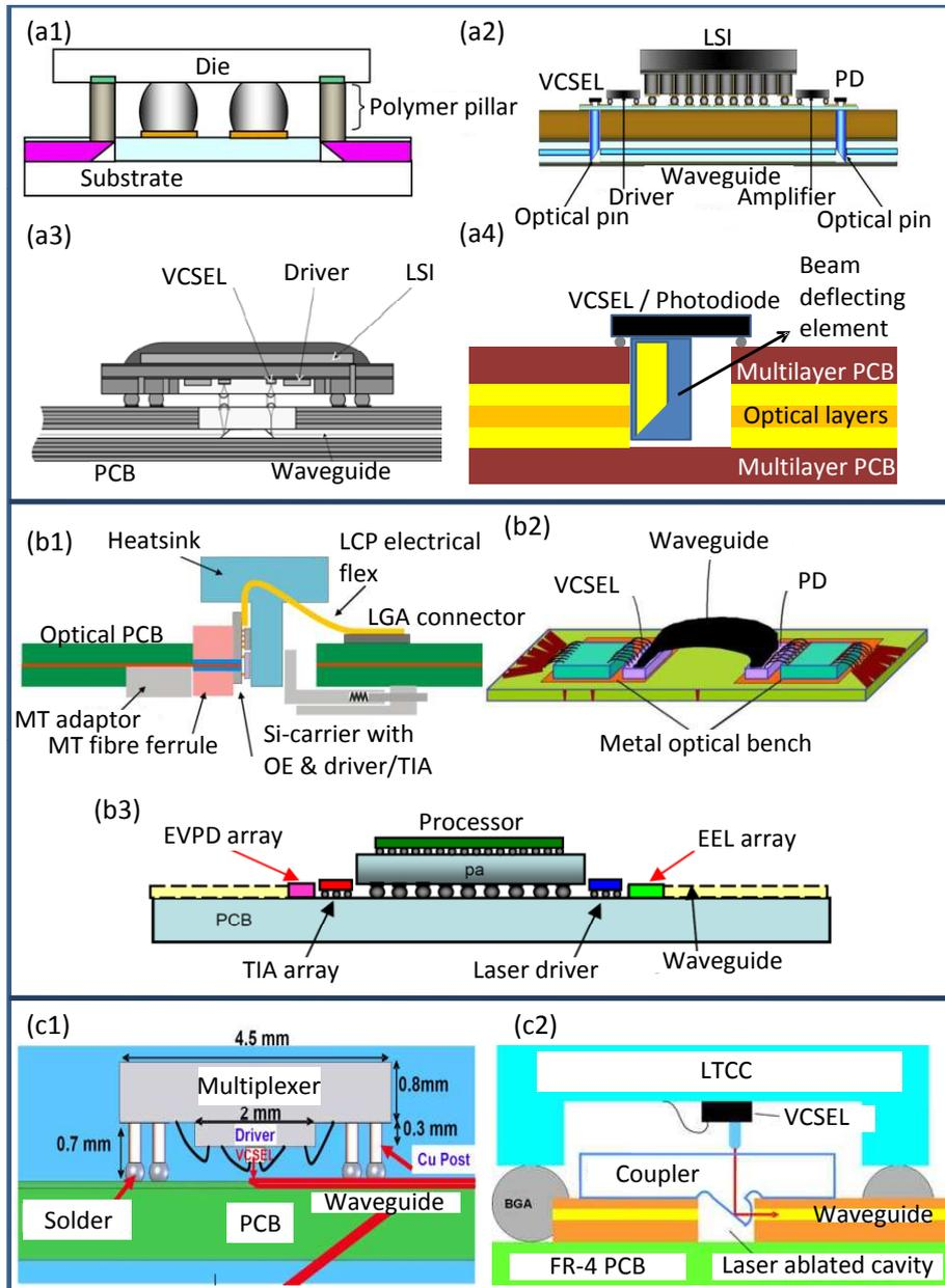
Figure 1.2: State-of-the-art opto-electronic mounting principle schemes ( Part 1 ).
