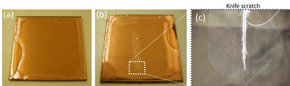
Figure 6.16: Scotch tape test (a) and scratch test (b)&(c) of a 30 μm thick copper layer on top of a 1 μm thin sputtered layer
