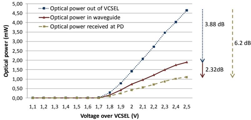
Figure 8.6: Results from the optical power loss measurement of both halves of the embedded optical link.
