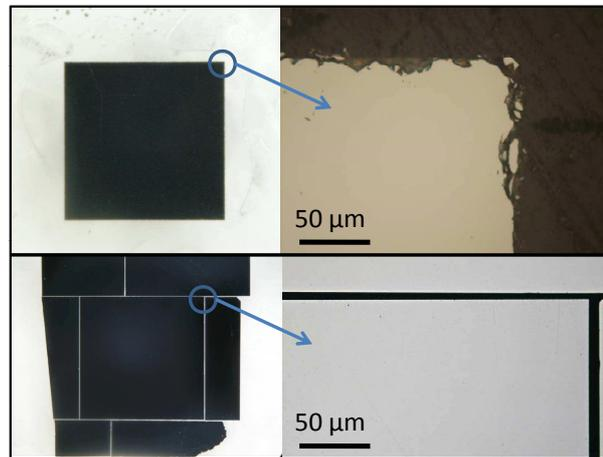
**Figure 5.18:** Edge damage after thinning of large GaAs dies ( $10 \times 10\ \text{mm}^2$ ) without the use of dummies (top) and with the use dummies (bottom).
