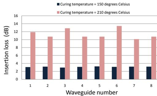
**Figure 4.21:** Optical insertion loss measurements for 3 cm long Truemode™ Backplane Polymer rigid optical waveguides on an FR4 board, cured at 150°C and at 210°C.
