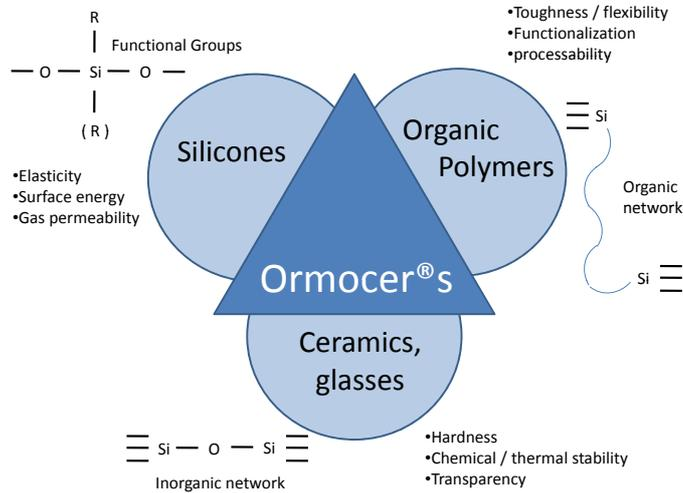
Figure 2.2: Structural composition of the Fraunhofer Institute Ormocers® .
