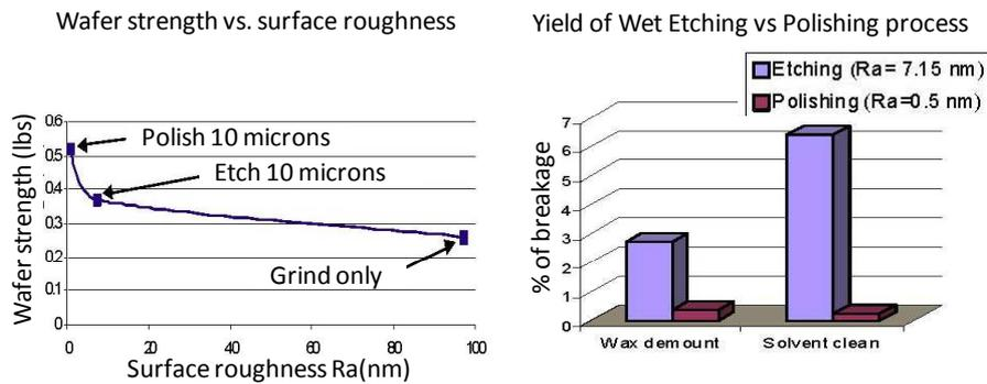
**Figure 5.2:** Relationship between backside roughness and wafer strength (*left*) and its consequences in the handling yield for grinded, polished and wet etched Si wafers (*right*) (Source: Skywork Solution Inc.).
