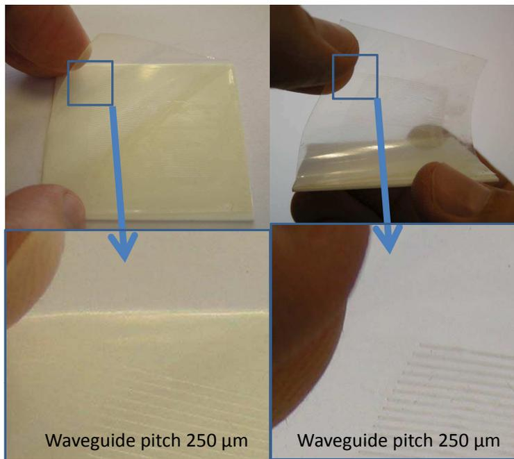
**Figure 4.5:** Manual release of a completed Epocore / Epoclad waveguide stack using the doublesided tape and LF0100 foil.
