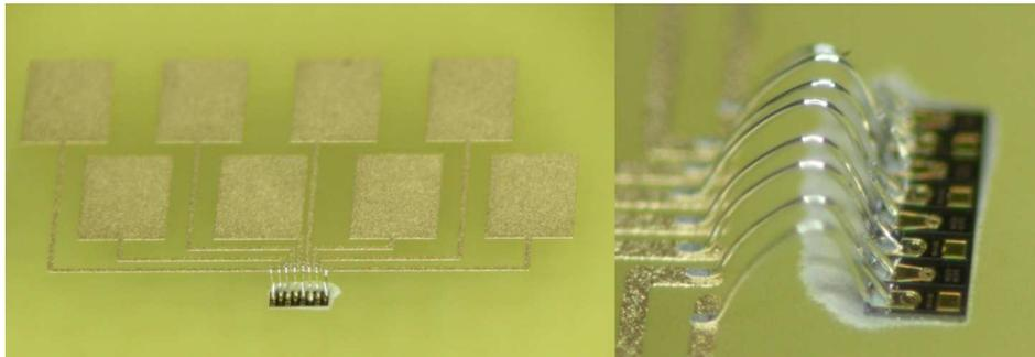
**Figure 5.20:** Wire bonded VCSEL package for optical characterization of a thinned VCSEL
