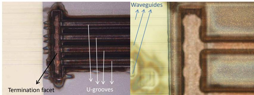
**Figure 7.34:** Laser ablated U-grooves for the embedding of optical fibers inside the optical foil.
