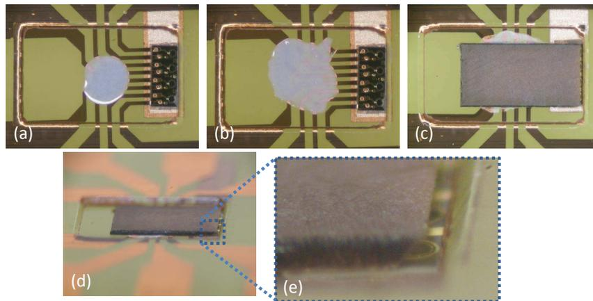
**Figure 7.30:** Pictures of the dispensing of the glue (a), the manual spreading of the glue (b), the placing of the mirror plug (c) and a close-up (d) & (e).
