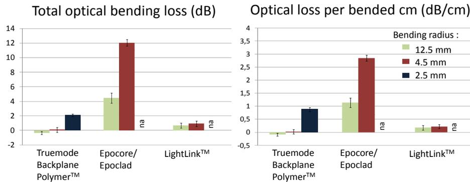
**Figure 4.24:** Total optical bending loss (left) according to the set-ups in Figure 4.23 and the recalculated losses per centimeter of bended waveguide length (right) for Truemode™ Backplane Polymer , Epocore / Epoclad and LightLink™ flexible waveguide foils.
