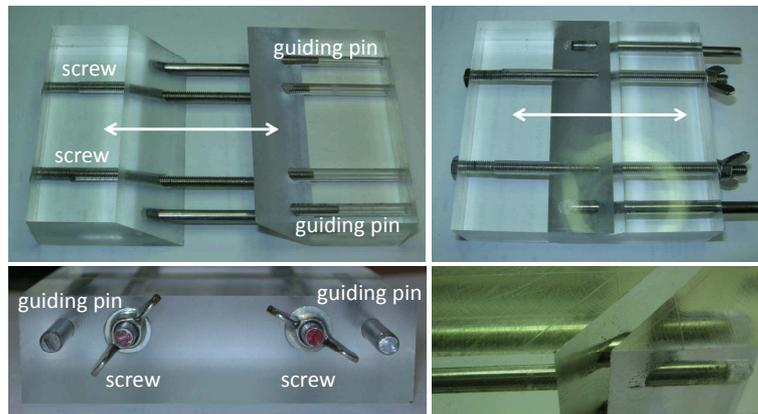
Figure 7.20: 45 degree mirror plug polishing tool.
