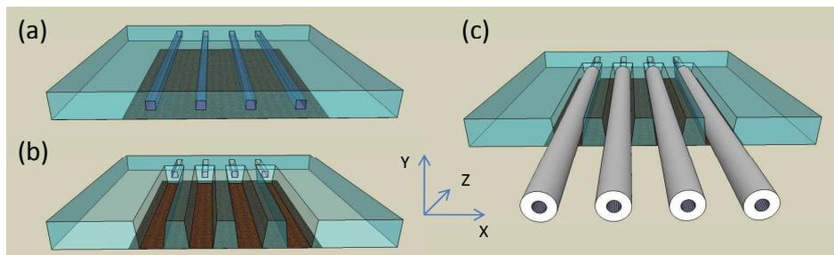
**Figure 7.32:** 3D schematic of the process flow to embed  $125\ \mu\text{m}$  diameter optical fibers inside the optical waveguide foil.
