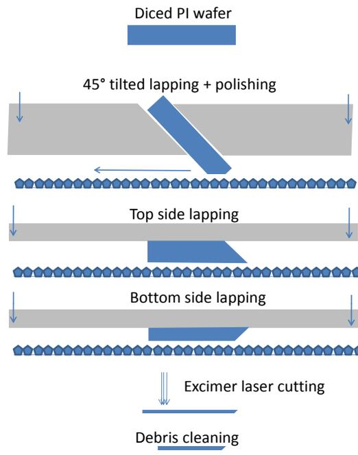
Figure 7.19: Schematic process flow for the fabrication of mirror plug components.
