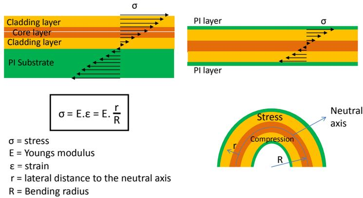
Figure 4.2: Principle of the neutral axis executed on the waveguide stack.
