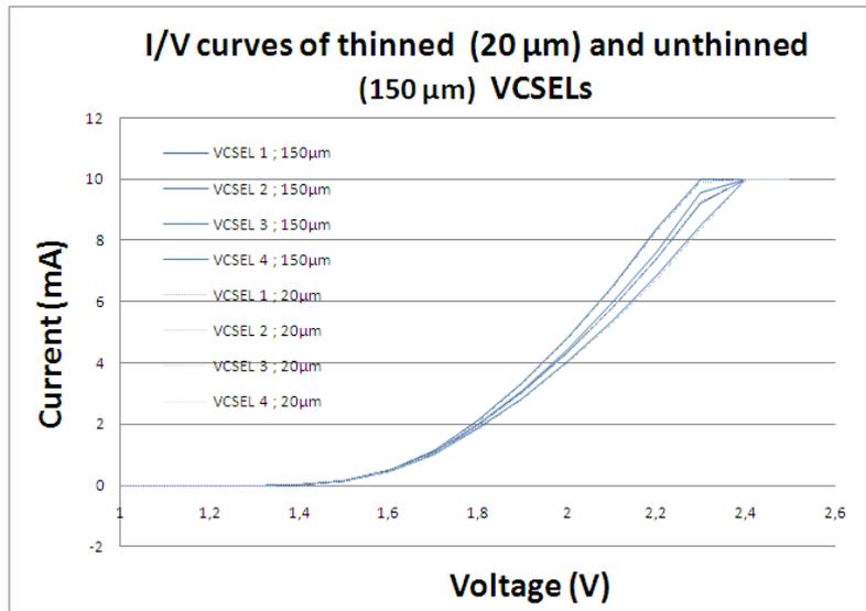
**Figure 5.19:** I/V Curves of 4 different VCSEL's in unthinned (150  $\mu\text{m}$ ) and in thinned (20  $\mu\text{m}$ ) status
