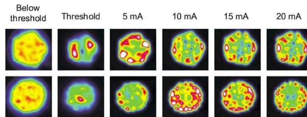
Figure 5.22: Near field images of 2 different oxide VCSELs for increasing driver current (Source: Finisar Corporation).
