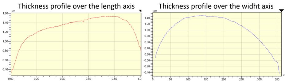
**Figure 5.13:** Thickness profile over the length and width axis of a polished 1 x 4 VCSEL array
