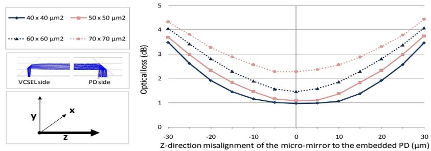
**Figure 7.11:** Optical loss simulation in function of the Z-misalignment of the micro-mirror with respect to the embedded photodiodes for different waveguide dimensions.
