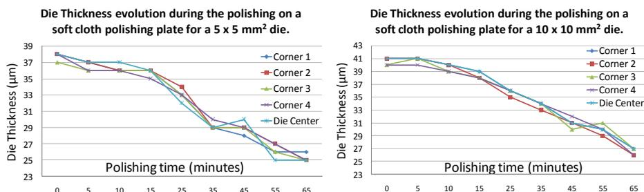
**Figure 5.9:** Chip thickness evolution during the polishing process for a  $5 \times 5\ \text{mm}^2$  and  $10 \times 10\ \text{mm}^2$  GaAs die
