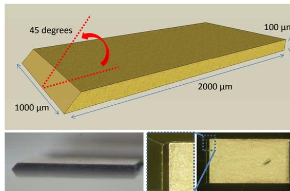
**Figure 7.27:** Overview of the dimensions of the mirror plug (top) and mirror plug pictures (bottom).
