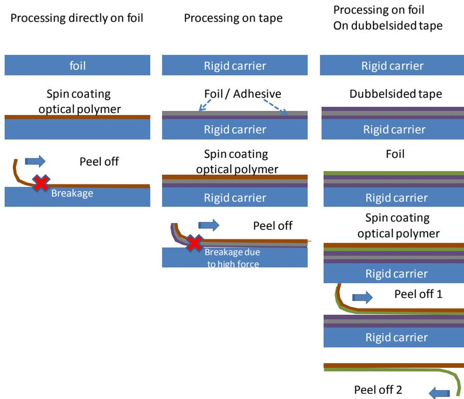
**Figure 4.4:** Peel off techniques for the release of optical polymer stacks after processing on a temporary rigid substrate.
