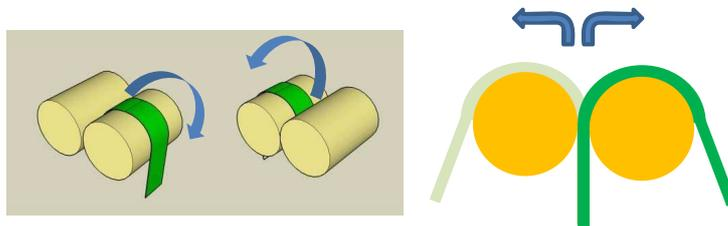
**Figure 4.22:** Bending test set-up for flexible optical waveguide foils
