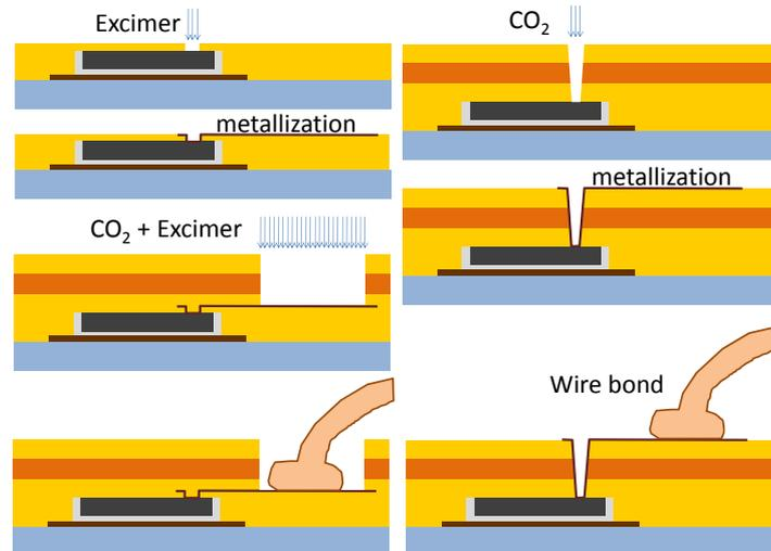
**Figure 6.7:** Schematic process flow for the fabrication of metalized micro-via's to the contact pads of embedded dies.
