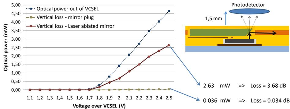
Figure 8.3: Optical power detected right above the VCSEL inside the optical link for laser ablated mirrors and mirror plug inserts.
