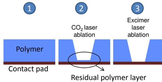
**Figure 6.24:** Schematic process flow for the opening of embedded contact pads.
