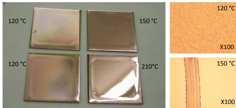
Figure 6.13: Pictures of 1  $\mu\text{m}$  thick sputtered Cu on a Truemode™ Backplane Polymer layer which was cured at 120°C, 150°C and 210°C.
