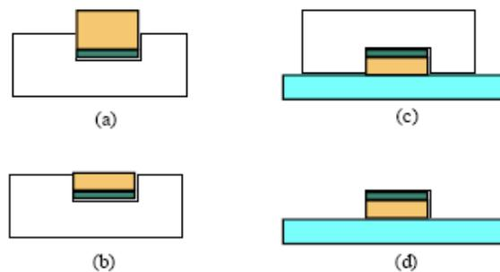
Figure 5.5: Cavity backgrinding approach for thickness control
