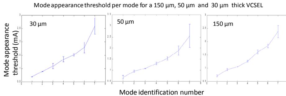
**Figure 5.25:** Mode appearance threshold per mode for a 150 μm , 50 μm and 30 μm thick VCSEL
