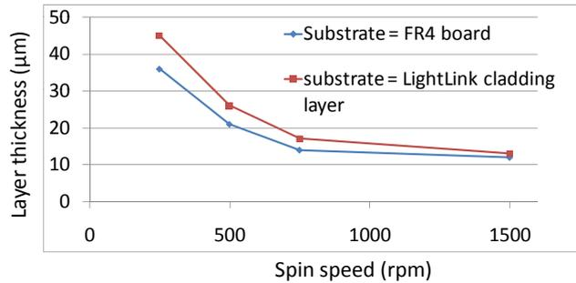
**Figure 3.5:** Influence of the underlying substrate on the spin speed curve of LightLink™ cladding material.
