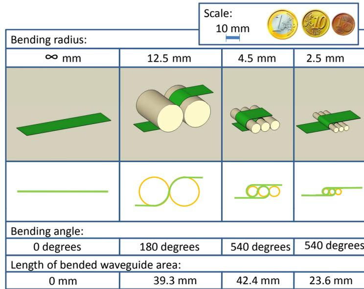
Figure 4.23: Optical bending loss measurement set-up for bending radii 12.5, 4.5 and 2.5 mm.
