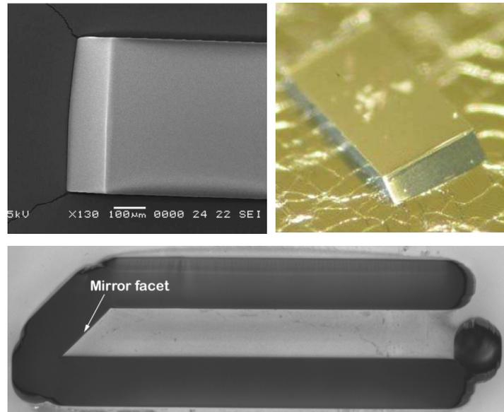
Figure 7.18: Mirror plugs fabricated with the use Deep Proton Writing (DPW).
