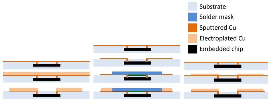
**Figure 6.17:** Three approaches for the plating of the fan-out of the galvanic interconnections towards embedded dies
