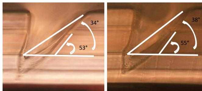
**Figure 7.16:** Cross-section of tilted laser ablation mirror trench, showing the different taper angle for the cladding and core material.
