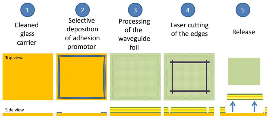
**Figure 4.15:** Schematic process flow of the release method for spincoated Polyimide on top of a float glass carrier, using selective adhesion promoter deposition.
