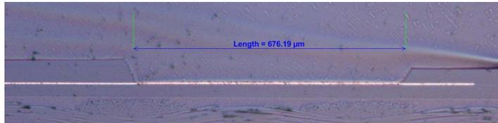
**Figure 6.23:** Cross-section of a contact pad, opened with CO<sub>2</sub> laser ablation.
