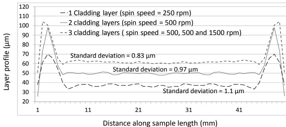
**Figure 3.7:** Planarization of a waved FR4 surface by spincoating LightLink™ cladding layers.
