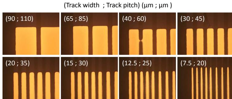
Figure 6.12: Copper fan-out etching resolution test
