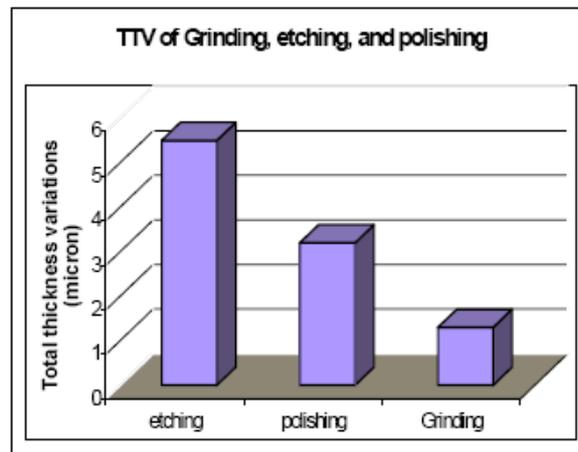
**Figure 5.1:** Influence of the thinning process on the total thickness variation (TTV)(Source: Skywork Solution Inc.).
