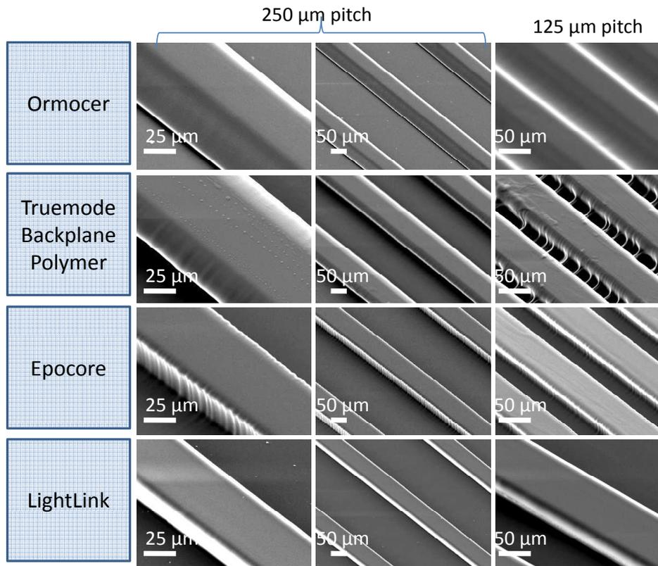
**Figure 3.16:** Scanning Electron Microscope pictures of Ormocers<sup>®</sup> , Truemode<sup>™</sup> Backplane Polymer , Epocore / Epoclad and LightLink<sup>™</sup> waveguides with a pitch of 250 and 125 μm .
