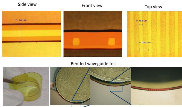
**Figure 4.16:** Side, front and top view of a Truemode™ Backplane Polymer flexible WG-foil using spincoated Polyimide (top) and bended state pictures.
