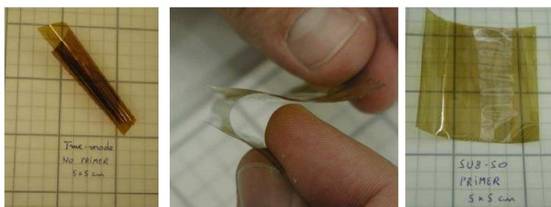
**Figure 4.10:** Examples of failure systems curling, cracking and delamination after processing of waveguide layers on top of an untreated Polyimide foil.
