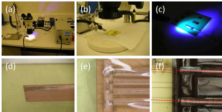
**Figure 7.35:** Mounting of the optical fibers inside the laser ablated U-grooves (a, b & c), side view of the mounted fibers (d) and top view (e & f).
