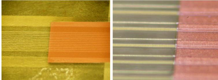
**Figure 7.33:** Copper island underneath the waveguides stack as laser stop for the U-grooves for optical fiber embedding.
