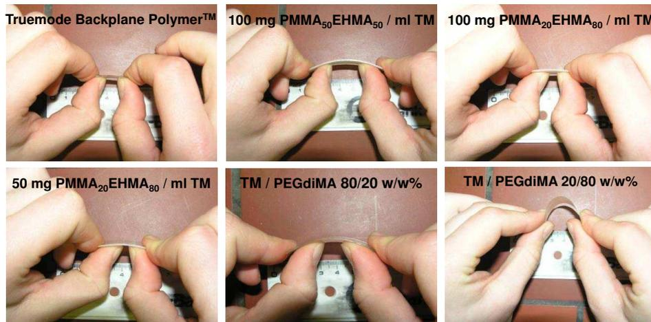
**Figure 2.9:** Visual comparison of the flexibility of the different developed mixtures/materials.
