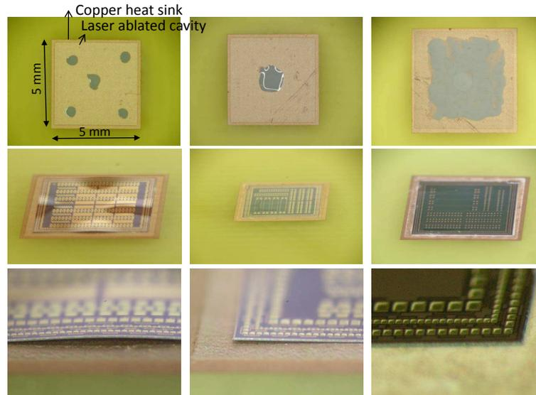
**Figure 6.26:** Three glue dispensing set-ups inside the cavity (top), together with the result after placement of the IC and the hardbake of the glue (center and bottom).
