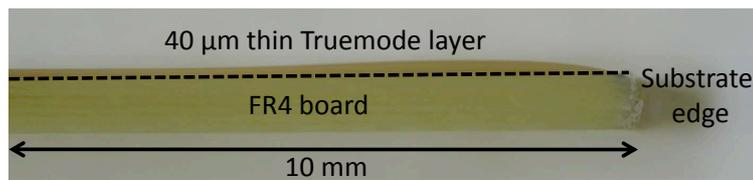
**Figure 3.3:** Cross-section of a 40 µm Truemode™ Backplane Polymer layer on top of an FR4 substrate with clearly visible edge bead
