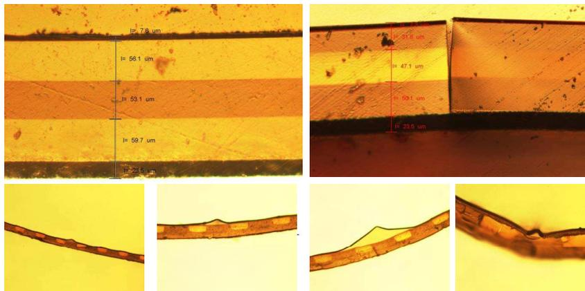
**Figure 4.14:** Truemode™ Backplane Polymer waveguide stack on top of a Polyimide foil and covered by a spincoated Polyimide layer (top left), breakage of the sample (top right) and delamination of the spincoated Polyimide layer (bottom).
