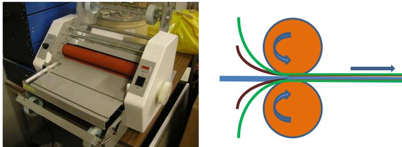
**Figure 4.6:** Dry film laminator picture (left) and schematic principle of the lamination process (right).
