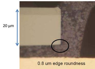
**Figure 5.10:** Edge roundness of a thinned VCSEL array due to the grooves in the wax at the edges of the die
