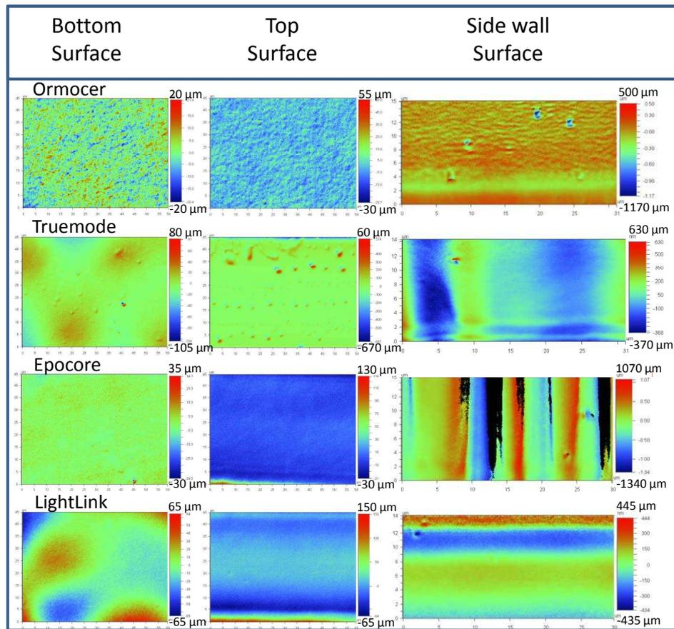
**Figure 3.19:** WYKO non-contact profilometer plot of Ra roughness measurements on the top and bottom surface of waveguides in Ormocers<sup>®</sup>, Truemode<sup>™</sup> Backplane Polymer, Epocore / Epoclad and LightLink<sup>™</sup> material ( $50 \times 50 \mu\text{m}^2$  area) and on the side wall surface ( $15 \times 30 \mu\text{m}^2$  area).
