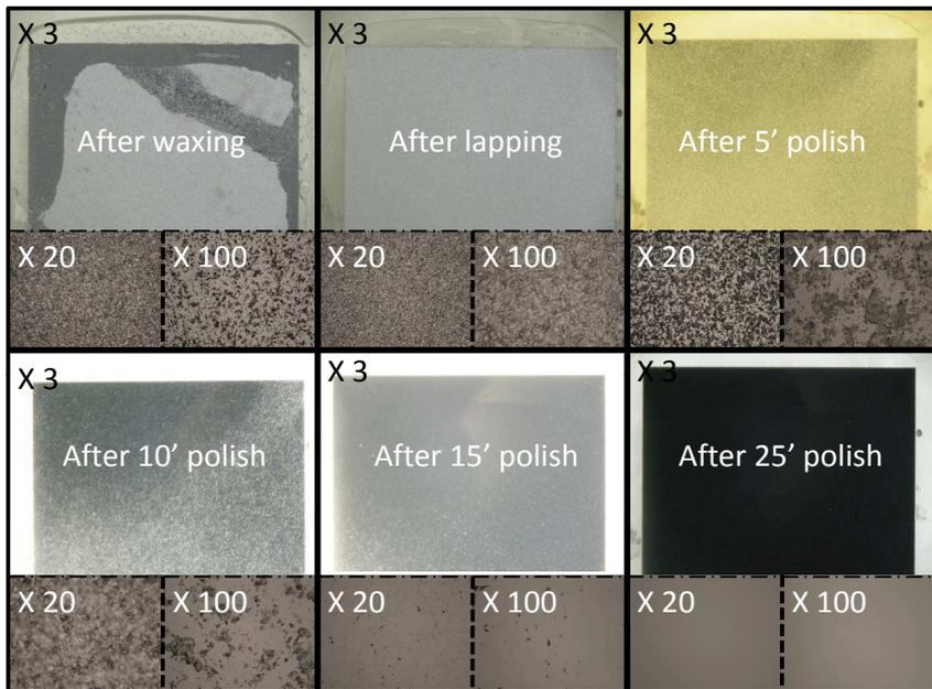
**Figure 5.16:** Backside roughness pictures for a  $10 \times 10 \text{ mm}^2$  GaAs die during the different thinning steps with magnification 3X, 20X and 100X
