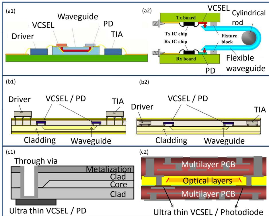
Figure 1.3: State-of-the-art opto-electronic mounting principle schemes ( Part 2).
