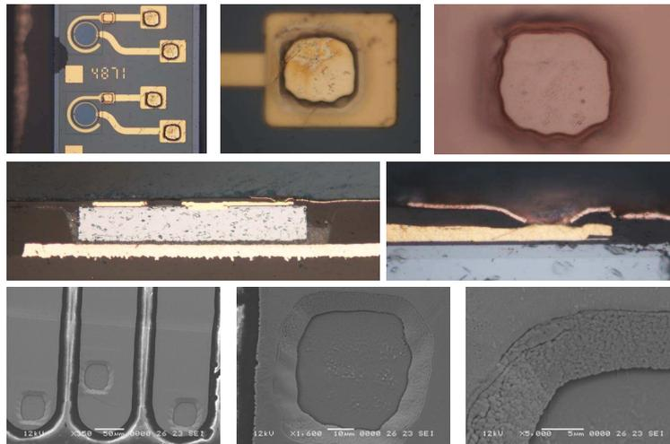
**Figure 6.19:** Microscopic pictures (top), cross-sections (center) and SEM pictures (bottom) of the contact pad delamination of Truemode™ Backplane Polymer .
