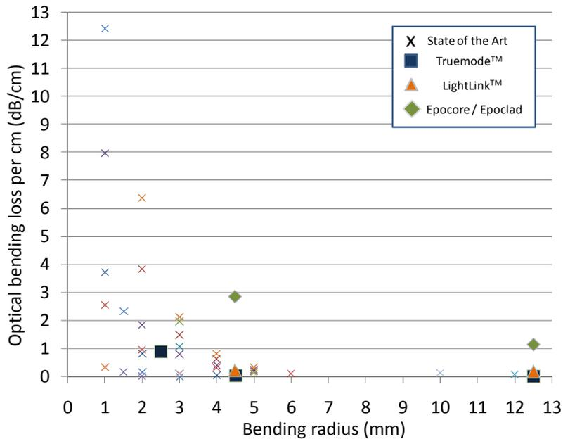
Figure 4.25: Bending losses of Truemode™ Backplane Polymer , LightLink™ and Epocore / Epoclad flexible waveguides versus the bending losses of state-of-the-art flexible waveguides.
