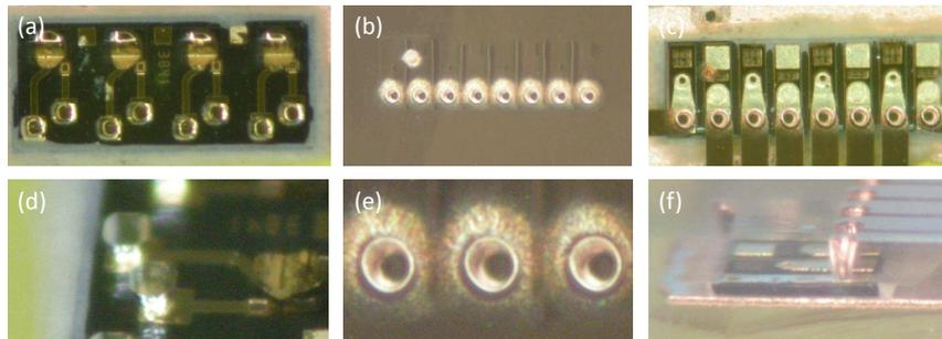
Figure 6.9: Photographs of CO<sub>2</sub> laser ablated vias to embedded opto-electronic components
