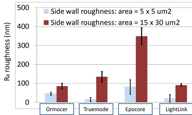
**Figure 3.18:** Ra roughness of waveguide side wall surfaces. Waveguides were fabricated in Ormocers<sup>®</sup>, Truemode<sup>™</sup> Backplane Polymer, Epocore / Epoclad and LightLink<sup>™</sup>. WYKO non-contact profilometer measurement on an area of  $5 \times 5 \mu\text{m}^2$  and on an area of  $15 \times 30 \mu\text{m}^2$ .
