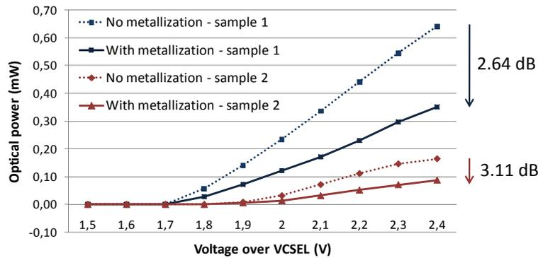
**Figure 8.7:** Total optical link loss with tilted laser ablated mirrors before, and after gold deposition on the mirror surface.
