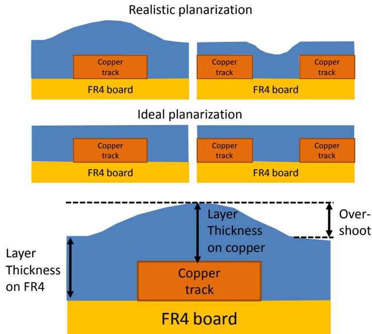
**Figure 3.6:** Planarization of a polymer spin-coated layer on top of a copper track or trench.
