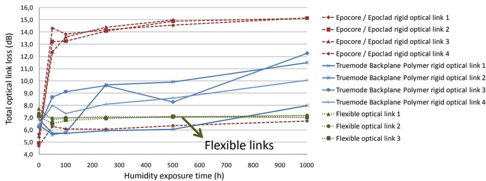
**Figure 8.18:** Evolution of the total optical link loss during the humidity exposure for flexible and rigid embedded optical links.
