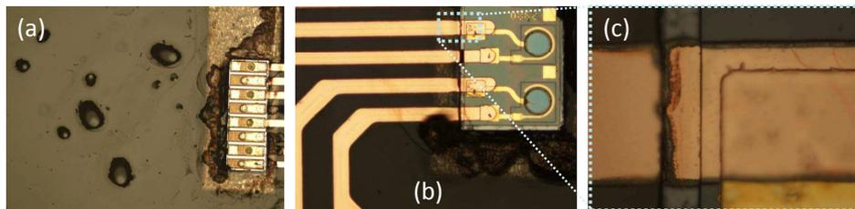
**Figure 6.31:** Drawbacks of Ormocers® as a chip embedding material.
