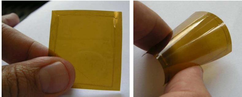
**Figure 4.8:** Laminated Truemode™ Backplane Polymer waveguide stack in between two Polyimide foils after lamination (left) and in bended state (right).
