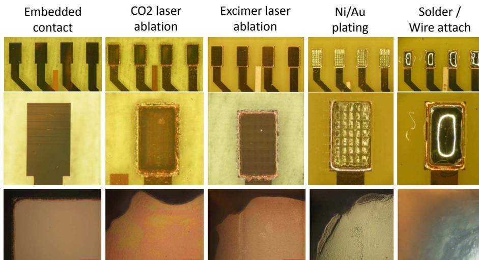
**Figure 6.25:** Pictures and close-ups of contact pads which are (from left to right): Embedded, CO<sub>2</sub> laser opened, Excimer laser cleaned, NI-Au plated and soldered.
