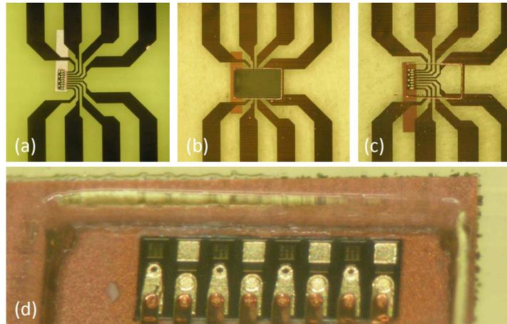
**Figure 7.29:** Picture of an embedded VCSEL with fan-out layer (a), of the laser stop island for the mirror plug cavity (b), of the cavity after wet etching of the cavity floor (c) and of a close-up on the waveguide facet (d).
