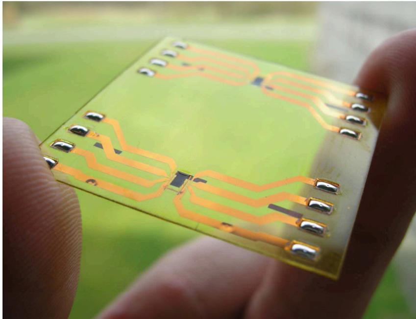
**Figure 9.1:** Picture of a  $180\ \mu\text{m}$  thin foil with embedded VCSEL-to-PD links and galvanic interconnections.
