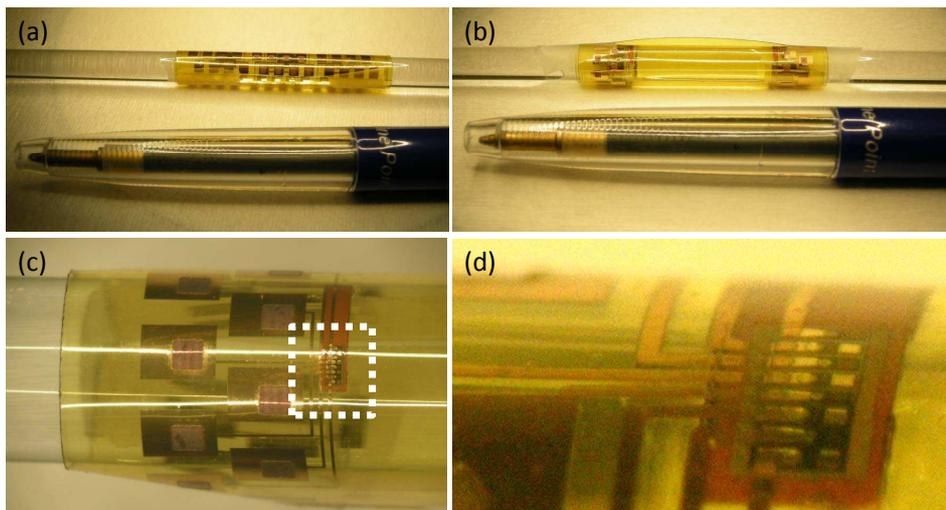
**Figure 8.15:** VCSEL and PD array package (inside one sample) rolled up around a cylinder with a 2 mm radius in both directions (a & b) and close-ups on the  $1 \times 4$  VCSEL array (c & d).
