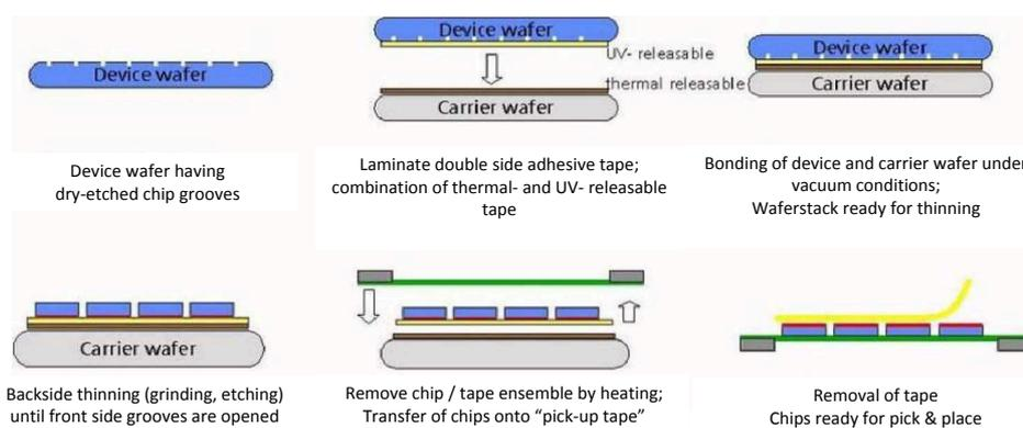
**Figure 5.4:** Schematic overview of the "dicing by thinning" principle followed by the transfer of the dies from the thinning carrier wafer to a low tac tape (pick & place tape). (source:IZM)
