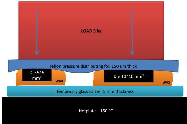
**Figure 5.8:** Wax mounting of 5 x 5 mm<sup>2</sup> and 10 x 10 mm<sup>2</sup> GaAs dies with the use of a Teflon pressure distribution foil for optimized leveling of the dies after mounting.
