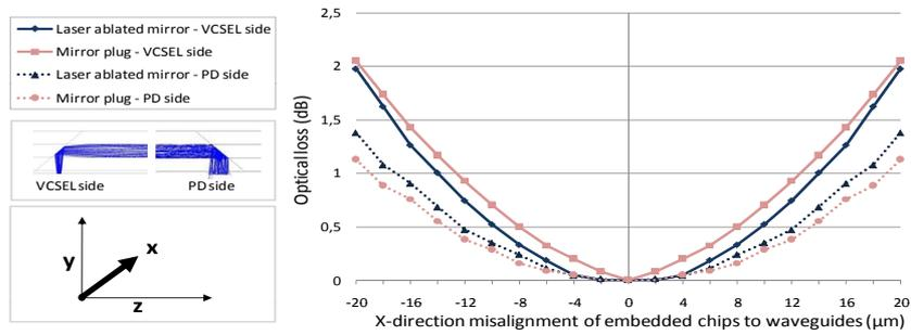
Figure 7.3: Optical loss simulation in function of the X-direction misalignment of the waveguides with respect to the active embedded VCSEL's and photodiodes.
