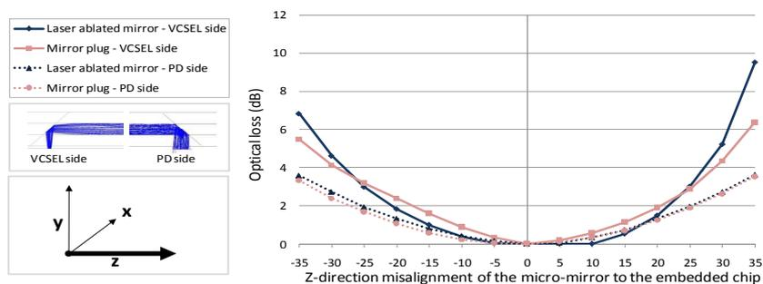
Figure 7.5: Optical loss simulation in function of the Z-misalignment of the micro-mirror with respect to the embedded VCSEL's / photodiodes.
