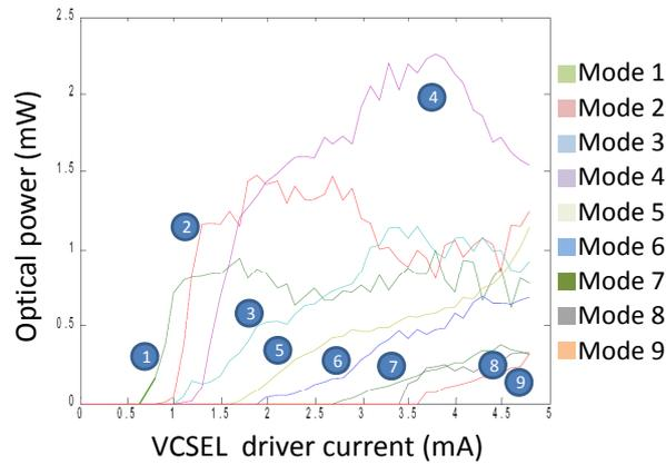
**Figure 5.24:** Power of each mode peak in the optical spectrum emitted by a multimode VCSEL versus the driver current.
