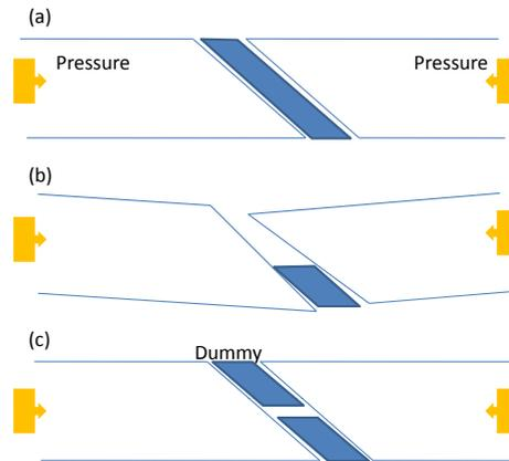
**Figure 7.21:** Dummy approach for the correct clamping of the mirror plug motherpiece in the PMMA 45 degree polishing tool.
