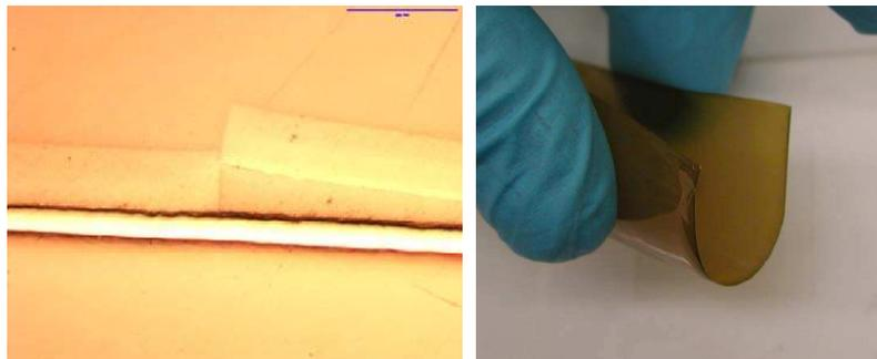
**Figure 4.12:** Cross-section of a fracture of a Truemode™ Backplane Polymer waveguide stack on top of a Polyimide foil (left) and a bended SU-8 layer stack on top of a Polyimide foil (right).
