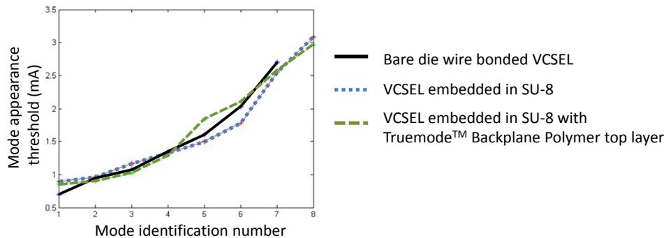
**Figure 8.35:** Comparison of the mode appearance thresholds for bare die wire bonded VCSEL's, embedded VCSEL's in SU-8 and embedded VCSEL's in SU-8, with a 30  $\mu\text{m}$  Truemode™ Backplane Polymer layer spincoated and cured on top.
