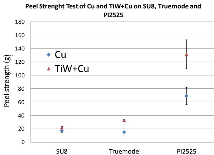
Figure 6.14: Peel strength test results of (1μm Cu)-strips and (50 nm TiW + 1 μm Cu)-strips on top of a PI2525, SU-8 and Truemode™ Backplane Polymer layer.
