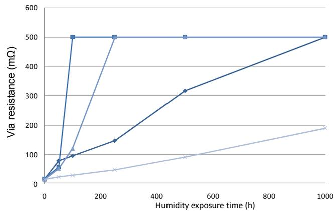
**Figure 8.21:** Evolution of the via-resistance of an embedded IC on a rigid FR-4 board during humidity exposure.
