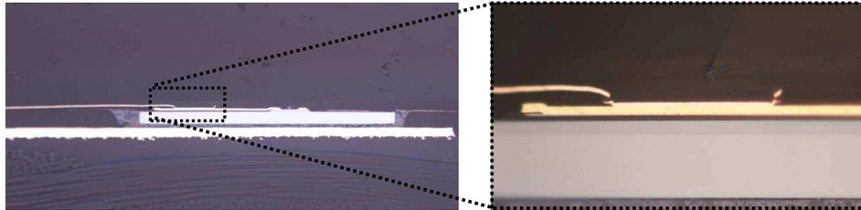
**Figure 6.20:** Cross-section of an Excimer laser ablated via through the SU-8 chip covering layer
