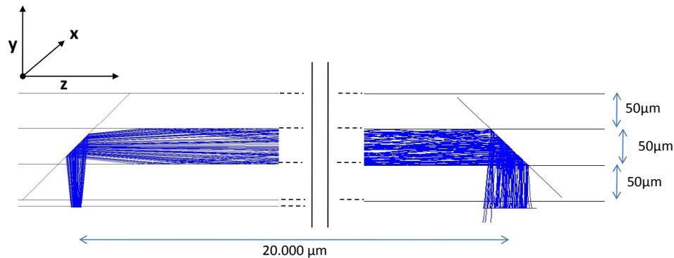
Figure 7.2: ZEMAX ray-tracing simulation set-up for the dimensional optical simulation of the embedded optical link.
