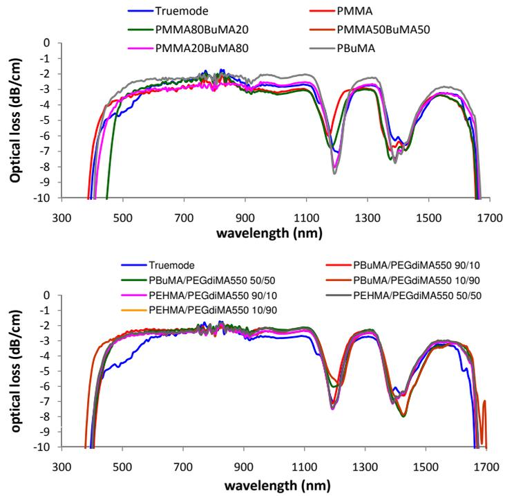
Figure 2.8: Optical bulk losses of Truemode™ Backplane Polymer material and the different mixtures/materials.
