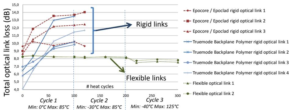
**Figure 8.17:** Evolution of the total optical loss of embedded flexible and rigid optical links during temperature cycling.
