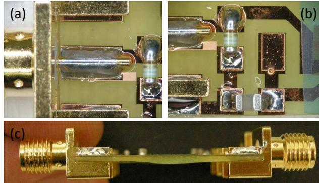
Figure 8.11: Soldering of the SMD and SMA components onto the opened contact pads (a & b) and a side view on the thinned substrate (c).
