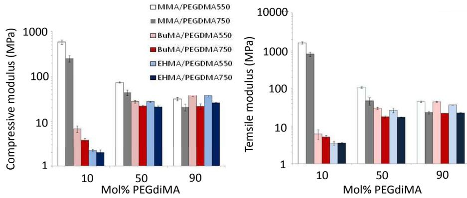
Figure 2.7: Compressive modulus and tensile modulus of the investigated mixtures/materials for different mol% PEGdiMA.
