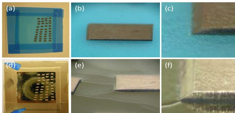
Figure 7.24: Pictures of mirror plugs mounted on a blue low-tac tape before metallization (a,b & c) and after metallization (d,e & f).
