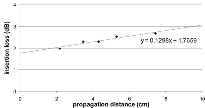
**Figure 4.20:** Cut-back optical waveguide propagation loss measurement for wet film Truemode™ Backplane Polymer laser ablated waveguides (Source: PhD-thesis Geert Van Steenberge)
