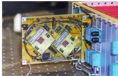
**Figure 3.1:** Fiber based optical interconnections integrated in a PCB (source: ACTS PLATO Project)
