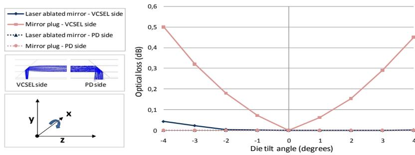
Figure 7.6: Optical loss simulation in function of the die tilt angle of the embedded VCSEL/photodiode.
