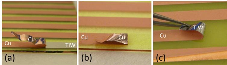
Figure 6.15: Pulling of the 3 mm wide metal strips for the peel strength tests.
