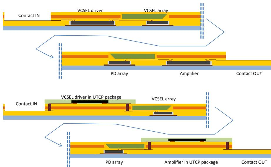
**Figure 9.2:** Next generation demonstrator principle with VCSEL drivers and trans-impedance amplifiers
