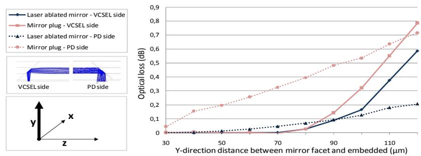
Figure 7.4: Optical loss simulation in function of the Y-distance between the embedded VCSEL's / photodiodes and the corresponding micro-mirrors.
