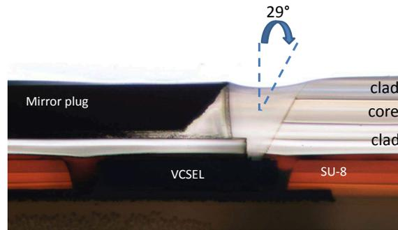
**Figure 7.13:** Cross-section of an embedded VCSEL array and mirror plug, showing the taper angle of the laser ablated mirror plug cavity side wall.
