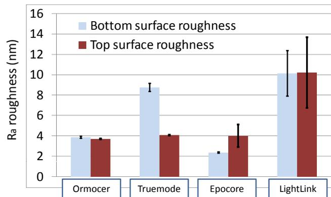
**Figure 3.17:** Ra roughness of waveguide top and bottom surfaces. Waveguides were fabricated in Ormocers®, Truemode™ Backplane Polymer, Epocore / Epoclad and LightLink™. WYKO non-contact profilometer measurement on an area of  $50 \times 50\ \mu\text{m}^2$
