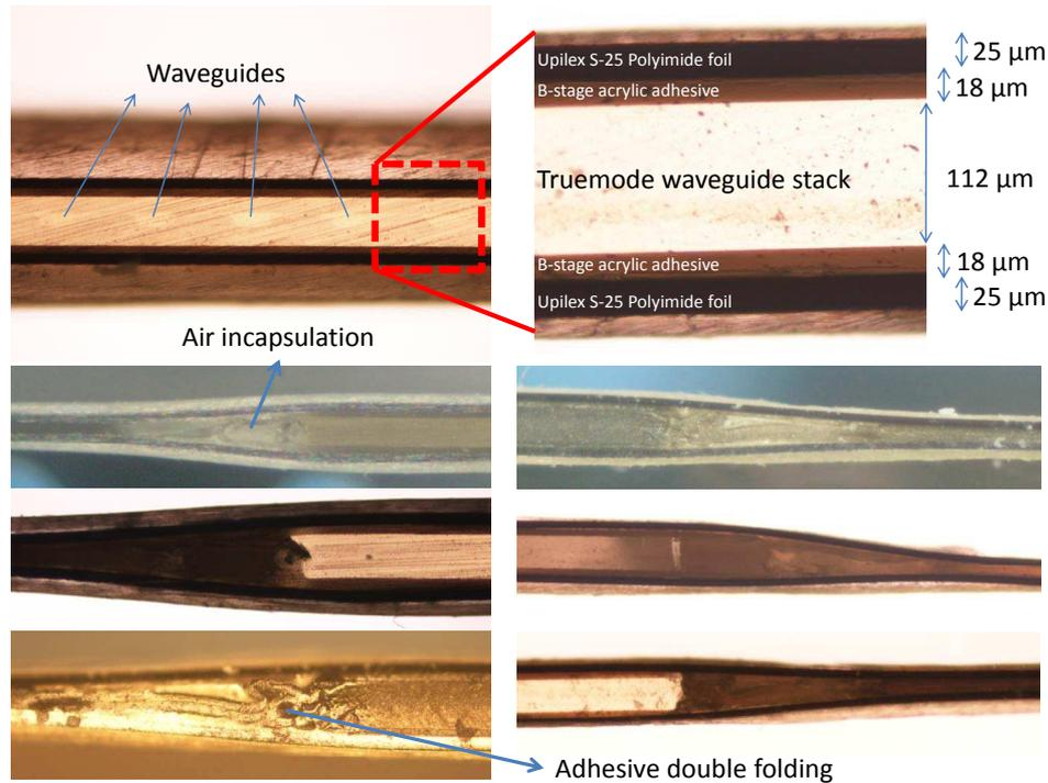
**Figure 4.7:** Cross-sections of a Truemode™ Backplane Polymer laminated waveguide stack with the layer thicknesses (top 2 pictures) and close-ups on the edges of the waveguide stacks (bottom 6 pictures)
