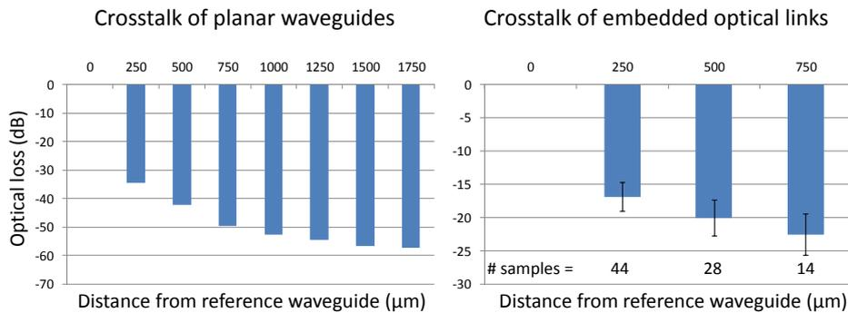
**Figure 8.8:** Crosstalk in neighboring plane waveguides (left) and crosstalk in neighboring complete optical links with embedded mirror plugs (right).
