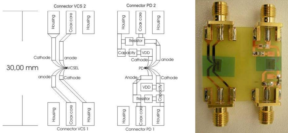
**Figure 8.10:** Design (left) and assembled rigid sample (right) for the embedded optical link to do time and frequency domain characterization at high-speed/high-frequency.
