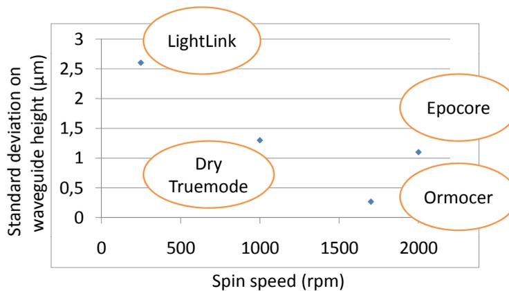
**Figure 3.15:** Spin speed versus waveguide height deviation for the 4 different materials, aiming at a waveguide thickness of 40 μm .
