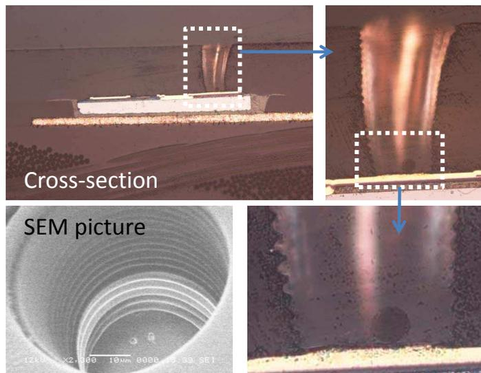
Figure 6.10: Cross-section of a CO<sub>2</sub> laser ablated via through the waveguide layers to the contact pad of an embedded VCSEL and an SEM picture thereof.
