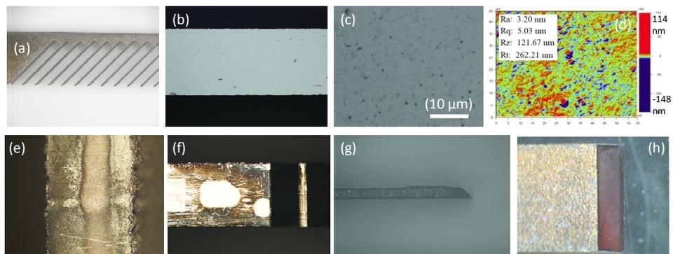
Figure 7.26: Pictures and measurements of Wire-EDM fabricated mirror plugs.
