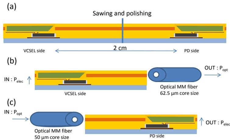
**Figure 8.5:** Set-up for the optical loss measurement of both halves of the embedded optical link.
