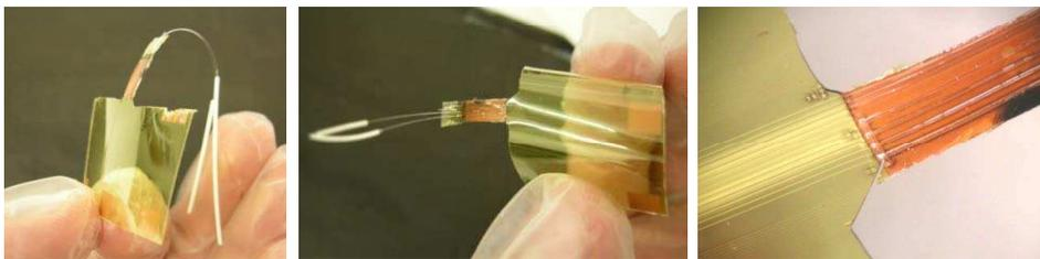
**Figure 7.36:** A completed optical waveguide foil connected to two optical fibers, bended in different directions (left and center) and a close-up of the fiber-connection (right).
