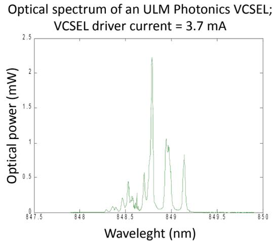
**Figure 5.23:** Optical spectrum of an unthinned ULM Photonics VCSEL, driven with a current of 3.7 mA.
