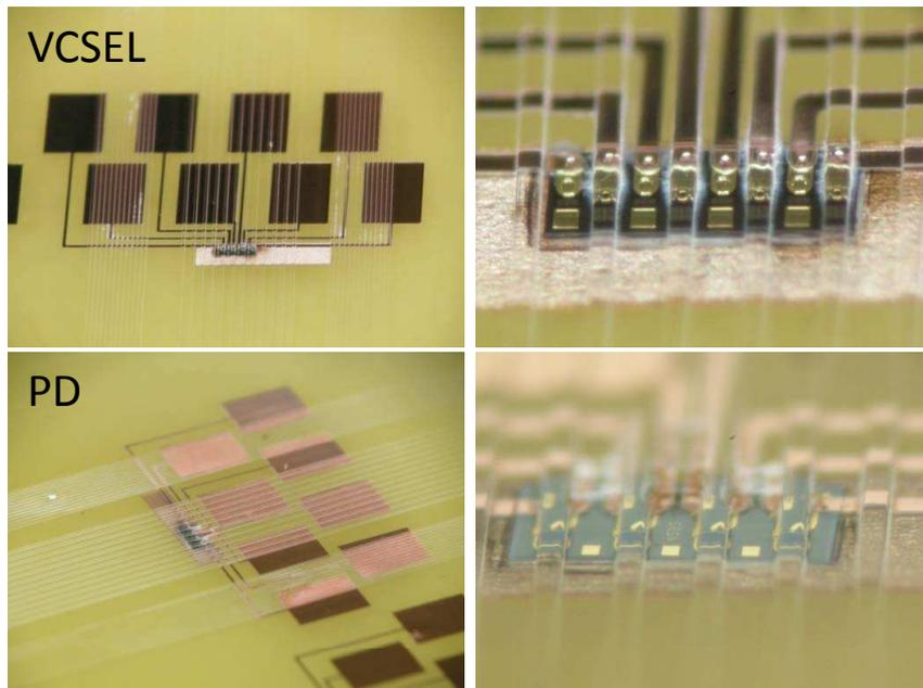
**Figure 6.6:** Microscope pictures of finished waveguides on top of an embedded VCSEL (top) and a photodiode (bottom).
