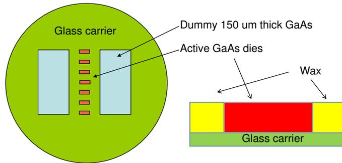
**Figure 5.7:** Wax mounting on glass carrier of 7 VCSEL arrays with 2 large ( $2 \times 3 \text{ mm}^2$ ) dummy dies (left) and cross-section (right)
