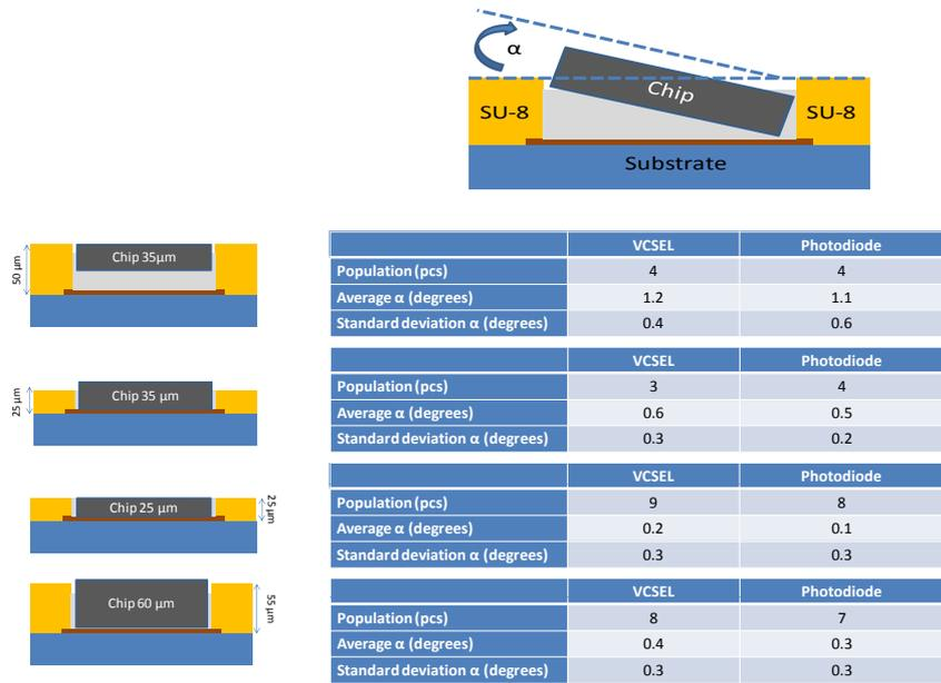
**Figure 6.4:** Tilt angle of a placed and leveled chip inside a laser ablated cavity with respect to the embedding layer surface.
