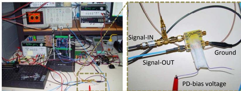
Figure 8.13: Set-up used to connect the optical link to a pattern generator to generate an eye diagram (left) and a close-up on the wired sample (right).
