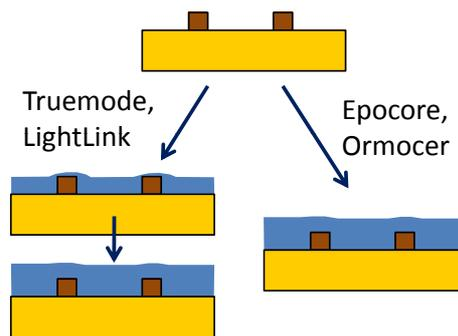
**Figure 3.20:** Applying of the uppercladding layer to cover the waveguides for Truemode™ Backplane Polymer , LightLink™ , Ormocers® and Epocore / Epoclad
