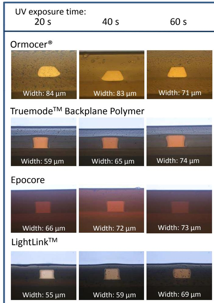
**Figure 3.11:** Cross-section of 250  $\mu\text{m}$  pitch waveguides in Ormocers®, Truemode™ Backplane Polymer, Epocore / Epoclad and LightLink™ material for different UV exposure times.
