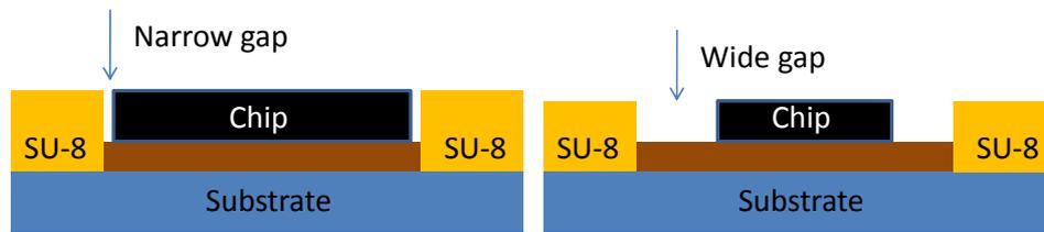
**Figure 6.2:** Schematic view on the aspect ratio of the gap between the embedded die and the cavity edge.
