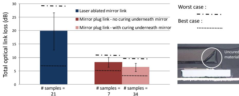
Figure 8.4: Average, standard deviation, worst case and best case of the total optical link loss for different coupling mirror situations.
