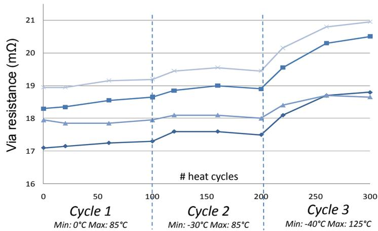
Figure 8.19: Evolution of the via-resistance during temperature cycling of an embedded IC.
