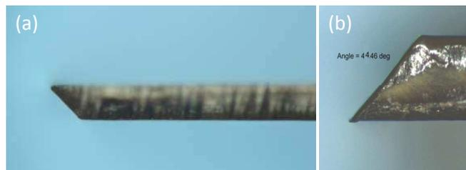
Figure 7.23: Sideview on a mirror plug (a) and close-up on the mirror facet (b).
