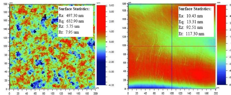
**Figure 5.14:** Backside roughness measurement with a non-contact profilometer (WYKO) of a lapped (left) and a polished (right)  $1 \times 4$  VCSEL array
