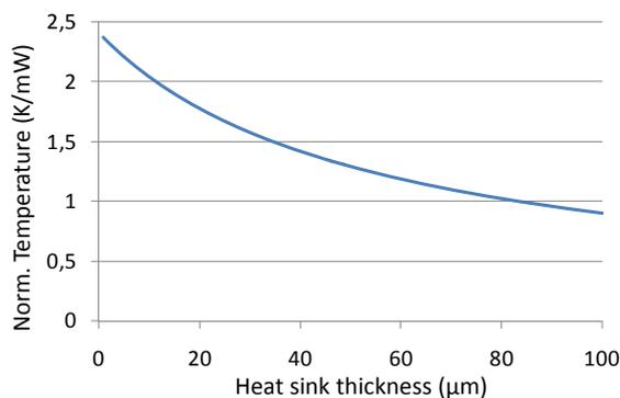
**Figure 8.33:** Normalized VCSEL temperature in function of the heat sink thickness.
