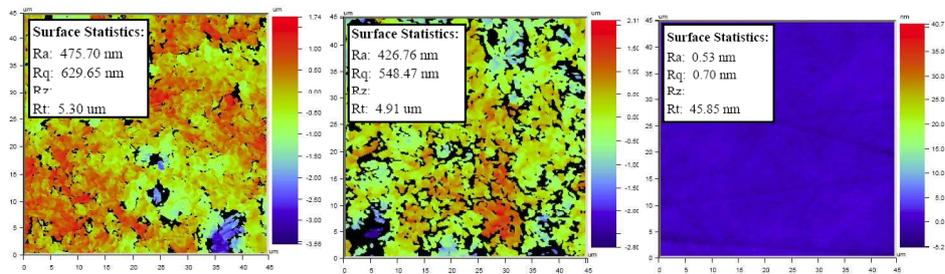
**Figure 5.17:** Non contact profilometer (WYKO) roughness measurements of a  $10 \times 10\ \text{mm}^2$  GaAs die on an area of  $50 \times 50\ \mu\text{m}^2$ . Left: not thinned; center: after lapping ; right: after 65 minutes polishing
