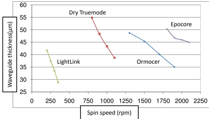
**Figure 3.13:** Spin speed curves for the core material of LightLink™ , Truemode™ Backplane Polymer , Ormocers® and Epocore / Epoclad .
