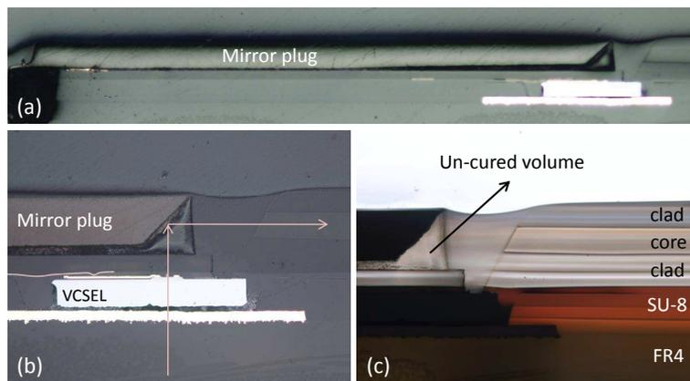
**Figure 7.31:** Cross-sections of a fully embedded mirror plug above an embedded VCSEL array.
