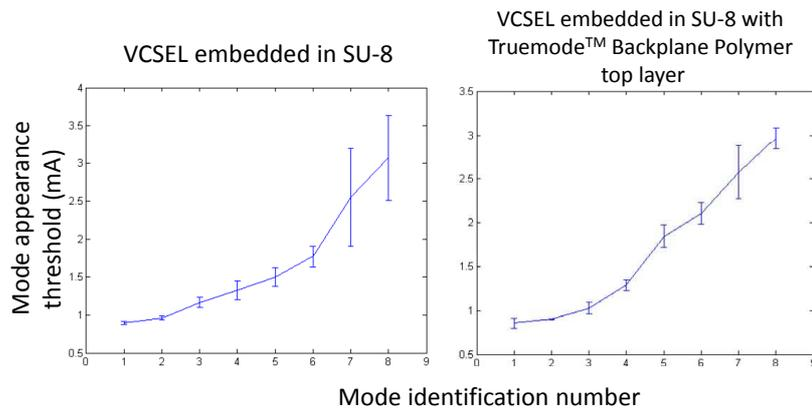
**Figure 8.34:** Mode appearance thresholds for embedded VCSEL's in SU-8 (left) and embedded VCSEL's in SU-8, with a 30  $\mu\text{m}$  Truemode™ Backplane Polymer layer spincoated and cured on top (right).
