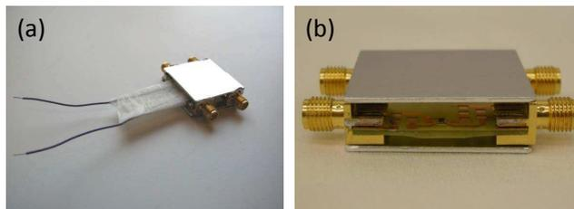
Figure 8.12: Soldered grounding/shielding plates and PD bias voltage wires to the rigid embedded optical link.
