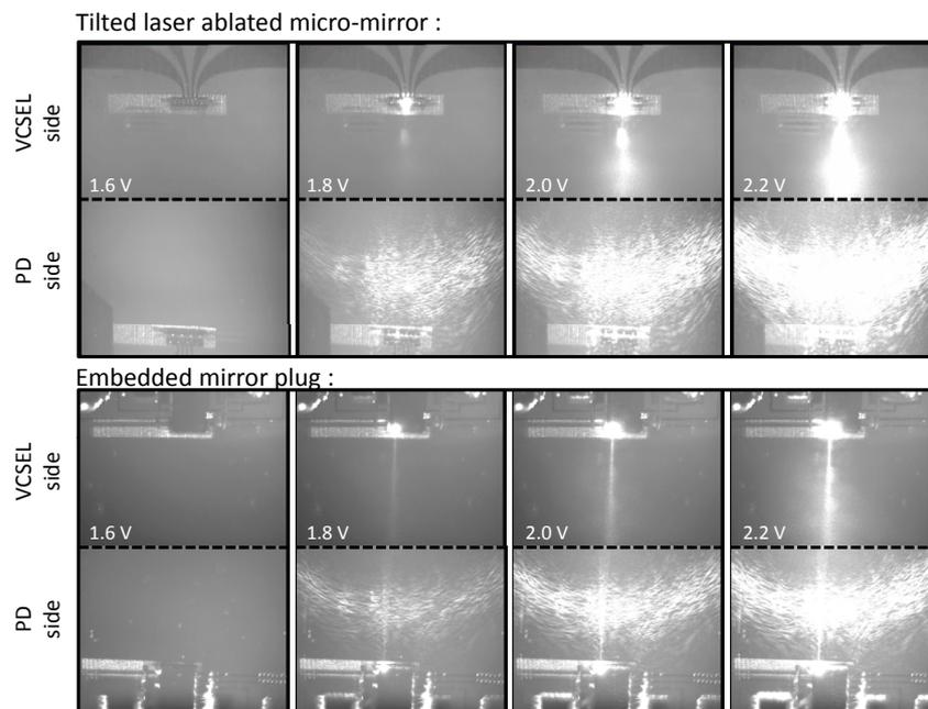
**Figure 8.2:** CCD camera screenshots above VCSEL and PD for an embedded link with laser ablated micro-mirrors (top) and with embedded mirror plugs (bottom).
