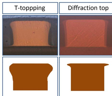
**Figure 3.10:** Pictures and schematic view of a cross-section from a waveguide suffering from T-topping (left) and a diffraction top (right).
