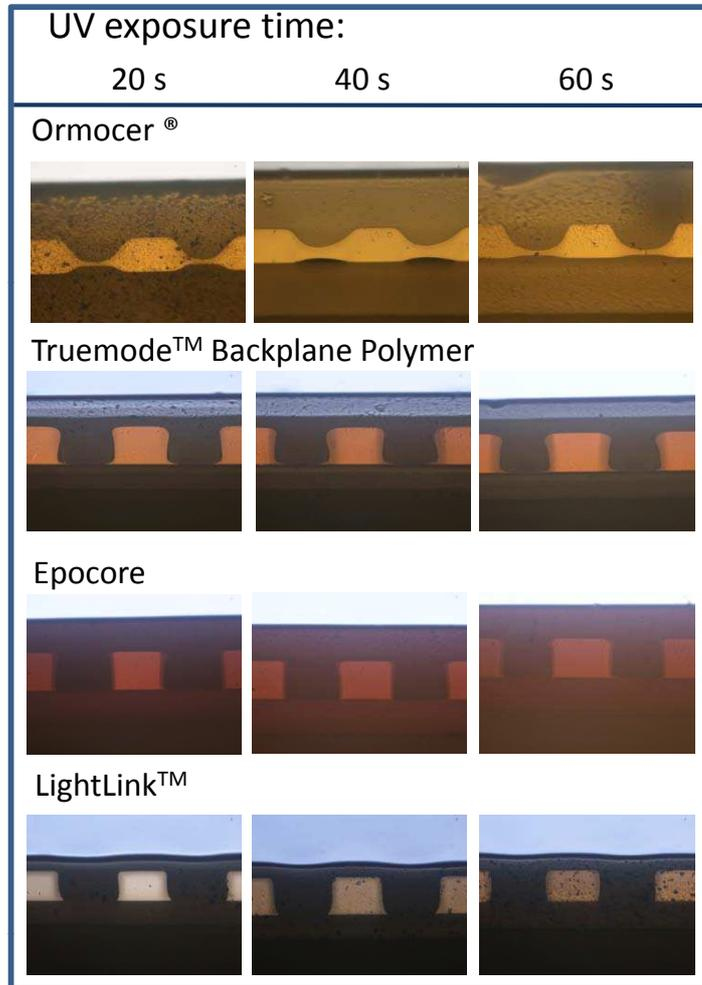
**Figure 3.12:** Cross-section of 125  $\mu\text{m}$  pitch waveguides in Ormocers<sup>®</sup> , Truemode<sup>™</sup> Backplane Polymer , Epocore / Epoclad and LightLink<sup>™</sup> material for different UV exposure times.
