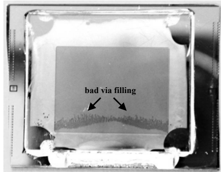
Fig. 4.4: Bad via filling when using the VFM.
