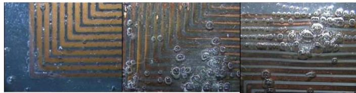
**Figure 7.13:** Inductive link after 1 month emersion in water environment: increasing number of bubbles and oxidation of copper.
