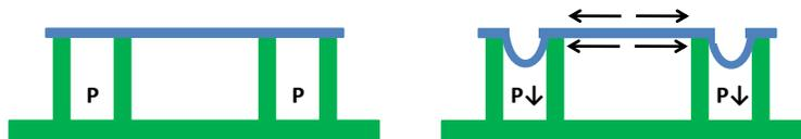
**Figure 7.2:** Stretchable multi electrode array: uniaxial stretching is realized by creating underpressure in the device.
