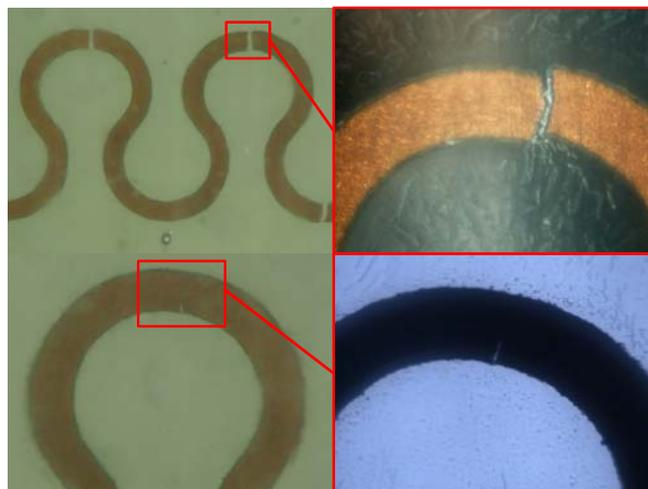
**Figure 6.20:** Complete breakdown and observed microcracks at top of meanders in pure copper sample after stretching 0-5%. Trace width is 100  $\mu\text{m}$ .
