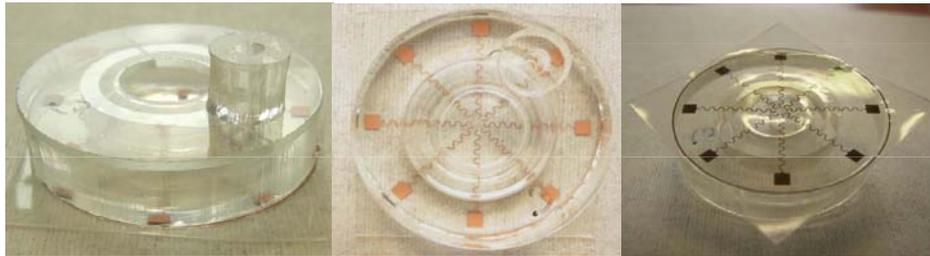
**Figure 7.1:** Stretchable multi electrode array cell cultivating device.
