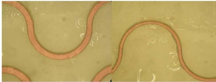
**Figure 5.40:** View on double sided meander tracks: silver conductor overprinting leads to shorts between top and bottom conductor.
