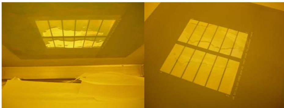
**Figure 5.14:** Behaviour of Durimide 116 on screen.
