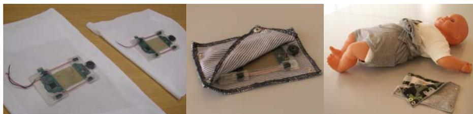
**Figure 7.34:** Stretchable respiratory monitor production: moulded demonstrator attached to different textiles.
