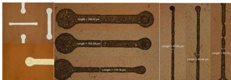
Figure 5.33: Closer view on printed tracks.
