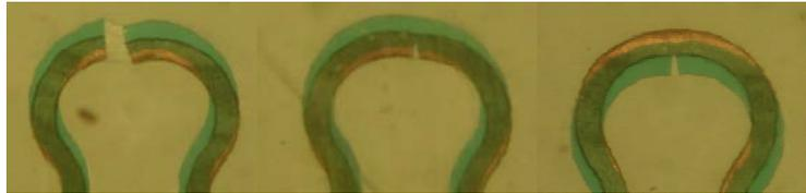
**Figure 6.22:** Complete breakdown and observed microcracks at top of meanders in soldermask covered copper interconnects after stretching 0-5%. Trace width is 100  $\mu\text{m}$ .
