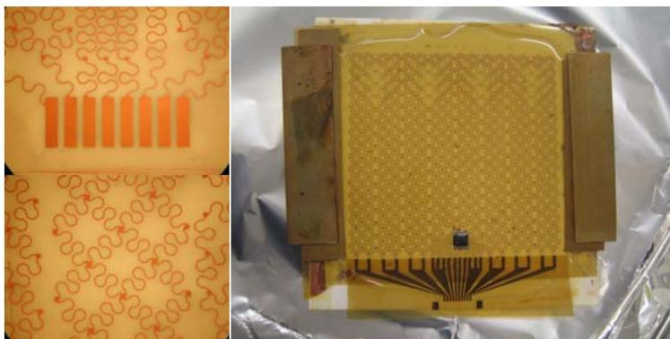
**Figure 7.23:** Stretchable heater: detail of stretchable connections.
