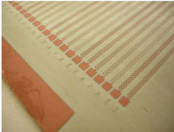
**Figure 4.19:** Spray etched sample containing meander tracks with different widths.
