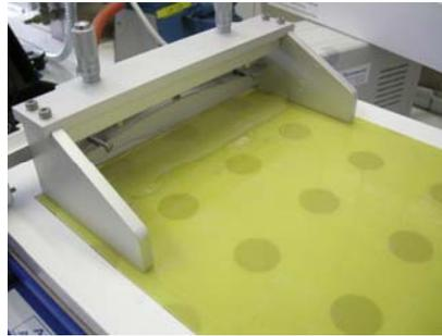
**Figure 4.26:** Application of PDMS by casting using a doctorblade.
