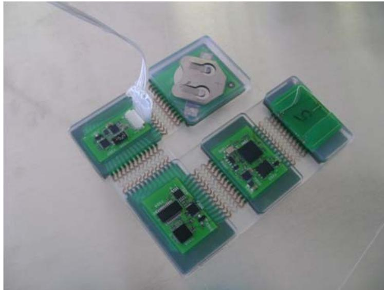
**Figure 7.45:** Production of fitness activity monitor: after moulding into Sylgard 186.
