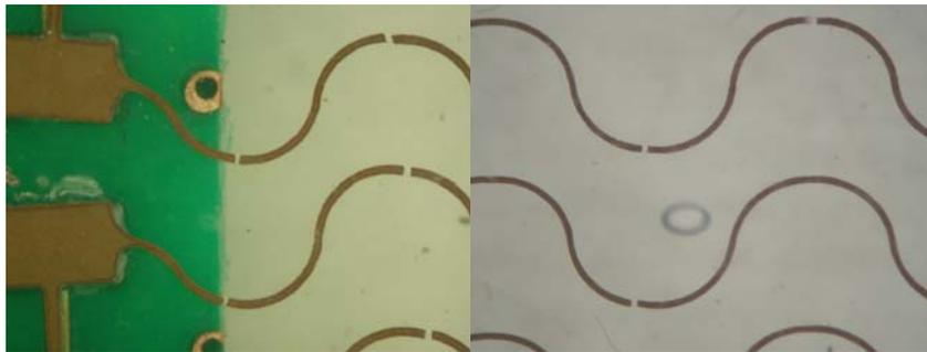
Figure 6.26: Observed failures after cyclic stretching.
