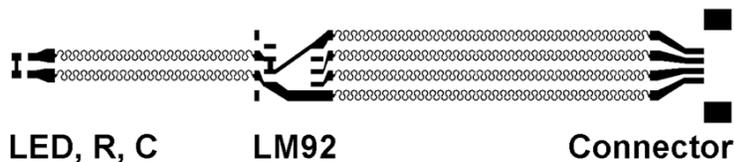
**Figure 7.3:** Electronic design of stretchable temperature sensor: copper etch mask.
