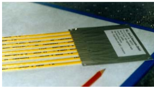
(c) Embedded optical fibers as a passive optical back-plane
