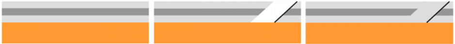
Figure 5.6: Process flow for the fabrication of a metal coated mirror embedded in the optical layer
