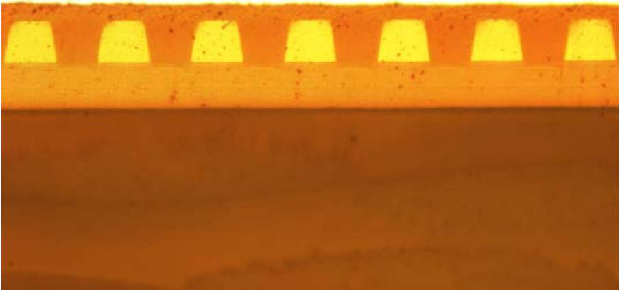
Figure 4.4: Microscope image of an array of KrF excimer laser ablated waveguides on a pitch of 125 μm (Truemode™)
