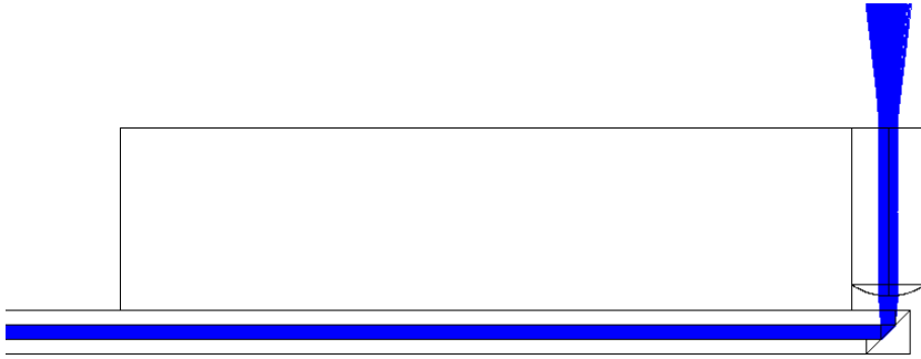
Figure 6.12: Ray-tracing simulation of the coupling interface
