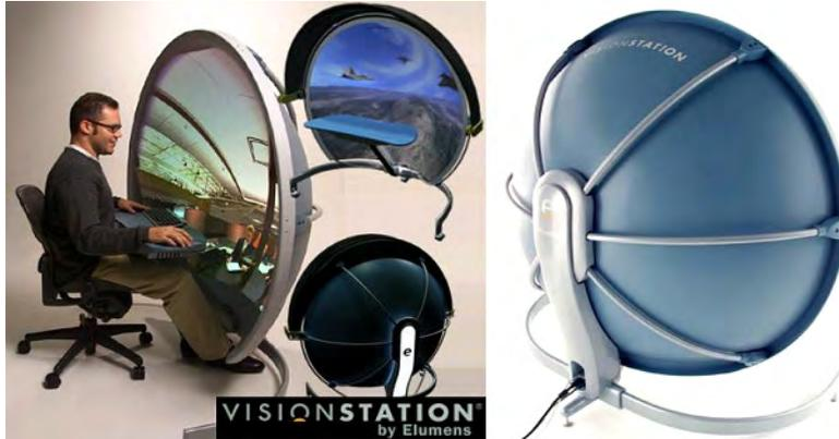
*Figure 1.16: The VisionStation (Elumens corp.) introduces 3D-vision by projecting the image on a parabolic screen*
