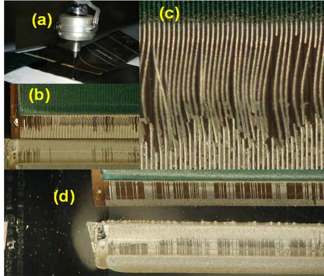
Figure 4.28: Peel strength tests on a bonded Hitachi TCP: (a) peel setup, (b) result of peeling along the bond length, (c) zoomed view and (d) result of peeling perpendicular to the bond length
