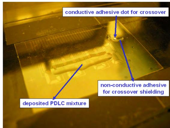
Figure 4.36: The PDLC mixture is deposited onto the bottom substrate after applying the crossover dot and an arc of shielding non-conductive adhesive
