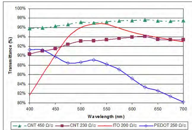
Figure 1.32: Optical performance: visible light transmittance of ITO, PEDOT and CNT films (EIKOS)
