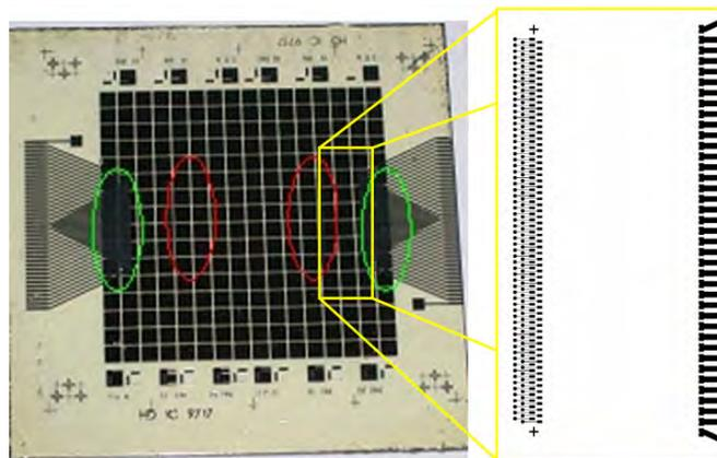
Figure 3.23: The detector substrate: a matrix of square photodiodes is visible, and the patterns where the read-out chips have to be bonded are marked and shown up-close (as designed)
