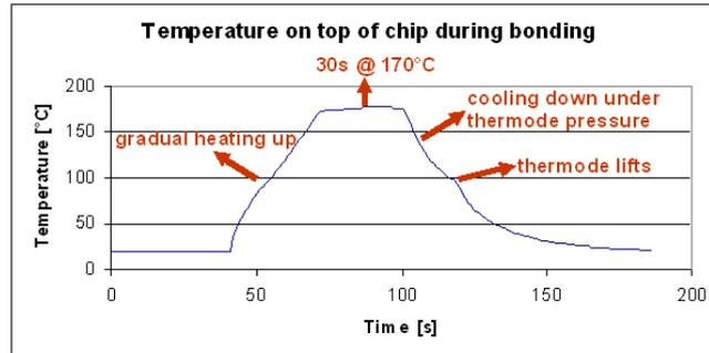
Figure 4.9: Temperature on top of chip throughout the actual bonding process
