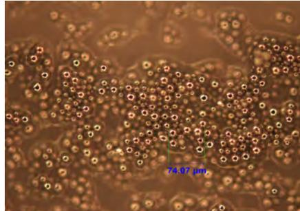
*Figure 2.33: Solder paste as seen through a microscope: the SnAgCu solder particles in the flux material are approximately 20  $\mu\text{m}$  in diameter*
