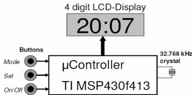
Figure 3.7: System design of the watch demonstrator
