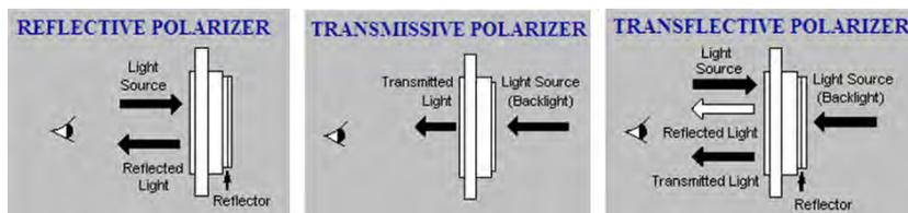
Figure 1.19: Light transmission modes for LCDs
