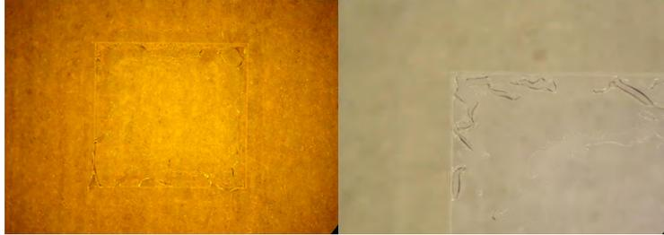
*Figure 6.28: Bad results after lithography of PI on a white ceramic background: traces remain at the edges of the cavity (5 mm by 5 mm)*
