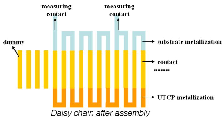
Figure 6.21: A daisy chain is formed between UTCP and substrate after assembly
