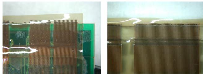
Figure 3.42: Flex foils bonded: column flex to PCB (left) and row flex to glass (right)
