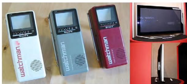
Figure 1.5: “Advanced” CRT technologies: flat CRTs by Sony (left) and an SED by Canon (right)
