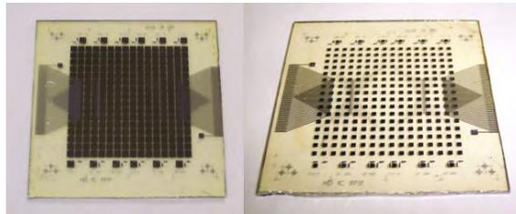
Figure 3.28: Two types of demonstrator substrates were used: large photodiodes (left) and small photodiodes (right)
