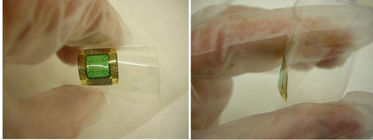
Figure 6.25: The resulting assembly, illustrating its bendability
