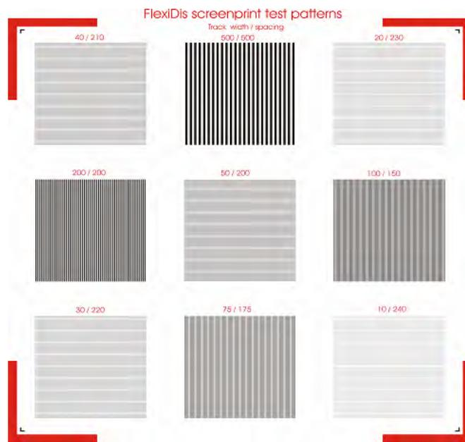
Figure 2.8: Test pattern design for fine line printing
