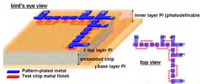
Figure 6.3: Interconnection test pattern design
