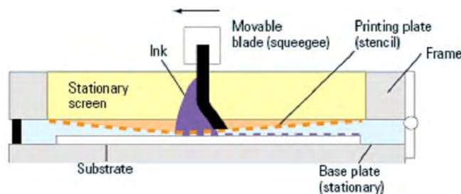
Figure 2.7: Stencilprinting principle
