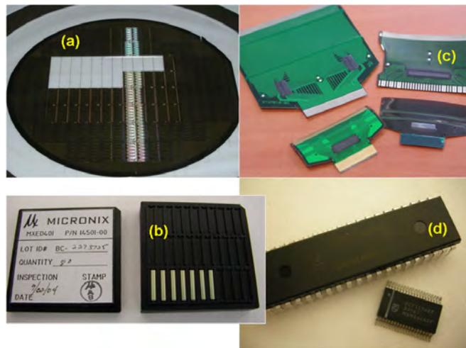
Figure 1.26: Examples of separate driver chips: (a) *Mjölnir* (see further on in Section 3.4) bare dies for row driving diced on a wafer tape, (b) bare die column drivers from Clare Micronix in a transport carrier, (c) driverchips from ST Microelectronics packaged as TCP, and (d) drivers in conventional through-hole and surface-mount packages
