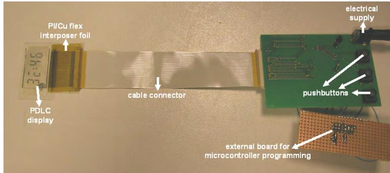
Figure 4.44: The final demonstrator of the thesis showing the PDLC display and its connected driving electronics on PCB; external power is supplied by a 12V-adapler; the pushbutton and crystal are assembled on the visible side of the PCB, the other components are mounted on the other side
