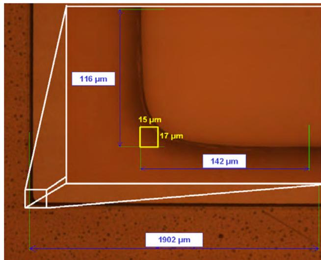
Figure 6.46: Picture of a cavity: zooming in illustrates how the rounded corners require the cavities to be larger than the chip
