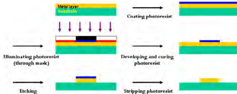
Figure 2.6: Schematical representation of typical lithographic patterning
