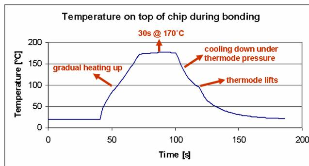
Figure 3.24: The temperature profile on top of the chip during thermocompression
