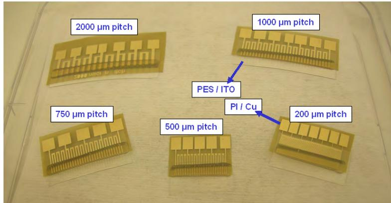
Figure 4.42: Bonded test patterns for electrical measurements
