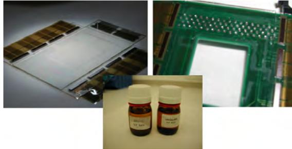
*Figure 3.43: The status of the display assembly before (left) and after (right) gluing the display to the PCB; the 2-component epoxy adhesive is shown in the middle*
