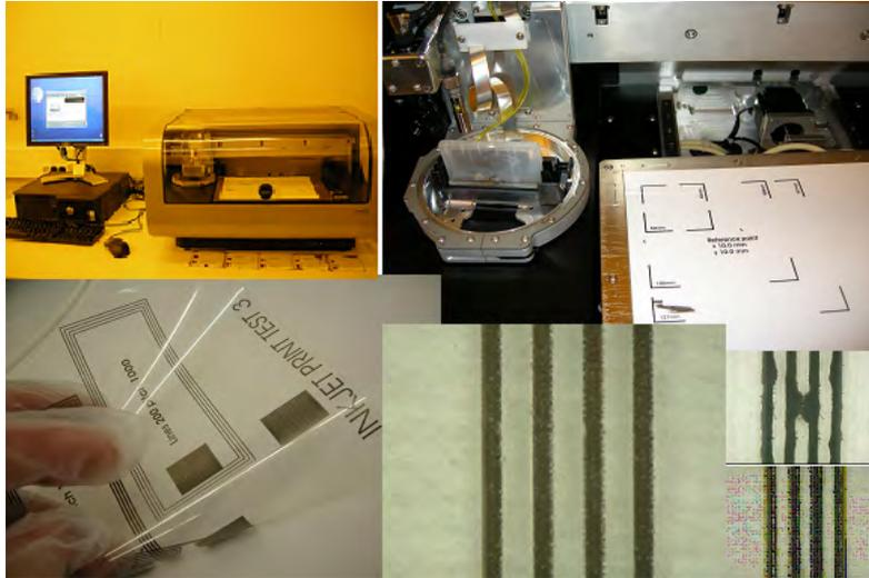
*Figure 2.21: Inkjetprinting: the PC-controlled Dimatix Materials Printer (top left), the inside of the printer (top right) and some bad and good results on PET (below)*
