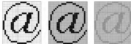
Figure 1.17: Illustrating the contrast ratio
