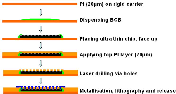
Figure 5.16: Process flow of the first UTCP technology, illustrating the principle
