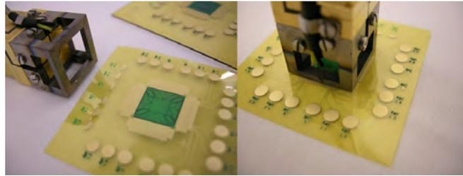
*Figure 6.17: The thermode for UTCP assembly matches the outputs' area of the UTCP; the round test pads on the package can be used for testing the embedded chip after packaging and are cut off prior to bonding*
