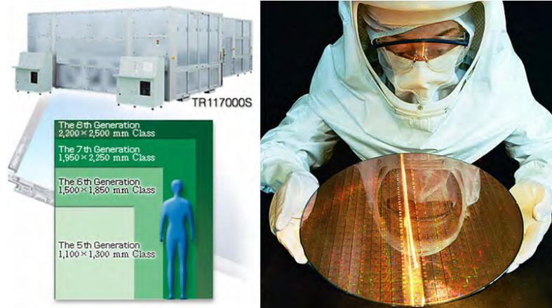
Figure 1.27: Illustration of the evolution in size: glass for LCD manufacturing (left, coating equipment TR117000S, Spinless) and maximal wafer sizes at present (right, Intel wafer)
