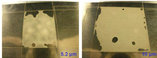
*Figure 4.32: The uniformity of the PDLC is influenced by the size of the spacers, specifically when flexible substrates are used*
