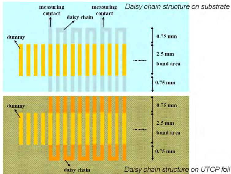
Figure 6.20: Matching designs for UTCP and substrates
