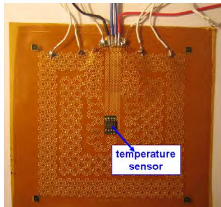
*Figure 2.1: First version of the heating element: note the temperature sensor in the middle and the (rather primitive) wiring interconnection as interface*
