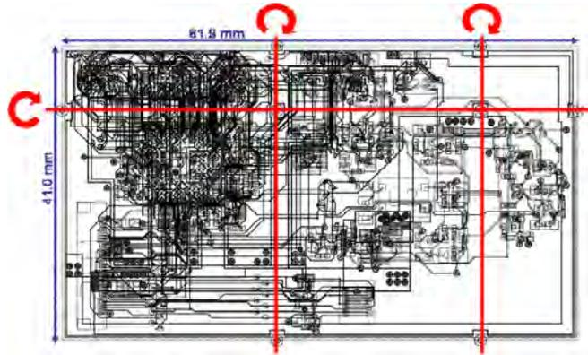
Figure 5.2: A flexible PCB for the driving electronics: the 3 flexing axes divide the substrate in 6 “rigid” islands onto which the components will be assembled, the punched holes at the intersection of the flexing axes are included to allow for bidirectional bending
