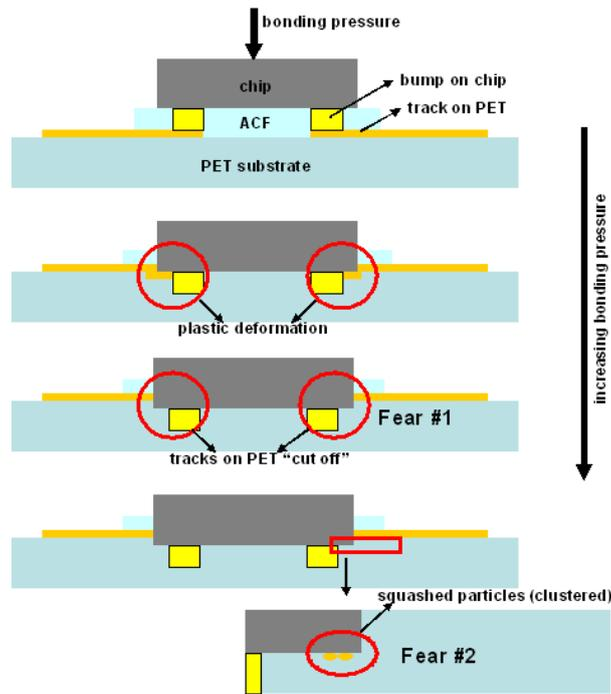
Figure 4.13: Schematic presenting fears that turned out to be wrong
