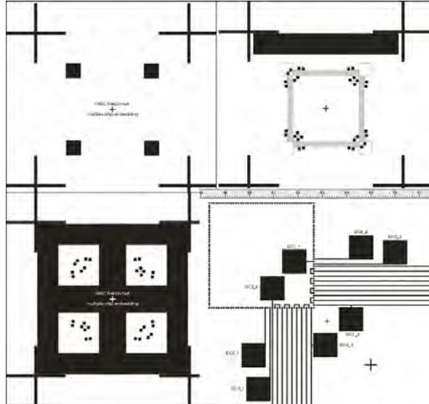
Figure 6.43: Mask layouts for multiple chip embedding: the cavities (upper left), metallization layer (upper right) and soldermask (below left); additionally the design of the upper left corner is shown more in detail (below right)
