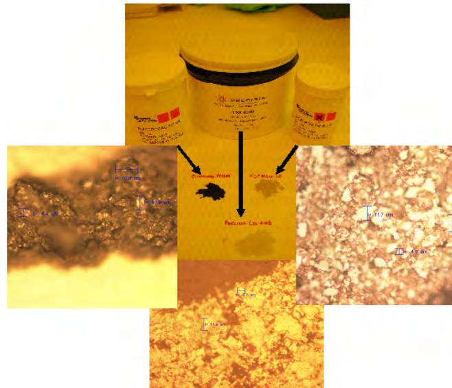
*Figure 2.12: Acquired inks for stencilprinting trials: Electrodag PM-406 (left), CSS-010B (middle) and XCE-80212-3iP (right)*
