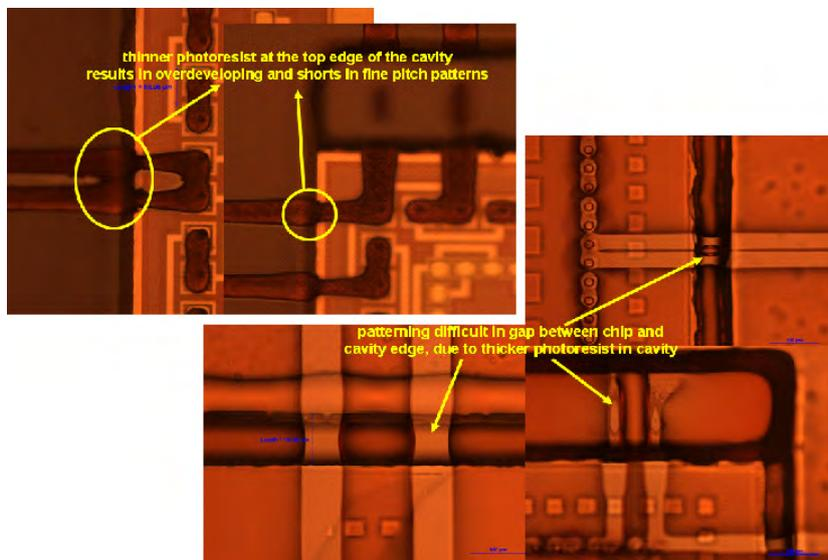
Figure 6.30: Problems arising in lithographic steps due to height differences between chip and PI layers
