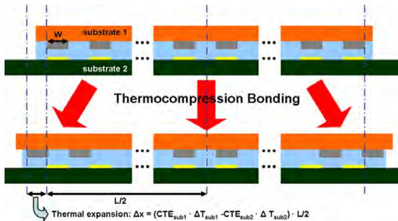
Figure 2.45: Principle of linear mismatch due to a difference in thermal expansion of the two substrates:  $L$  is the total bond length,  $W$  is the width of the bond pads,  $\Delta T$  is the difference between thermocompression and room temperature
