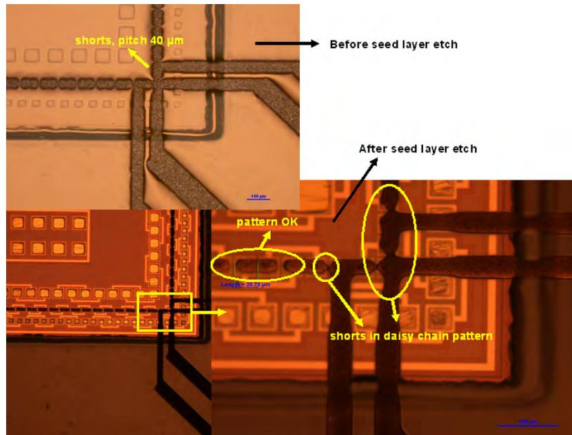
Figure 6.31: Fine pitch limitations in pattern definition ( $40\ \mu\text{m}$  pitch tracks)
