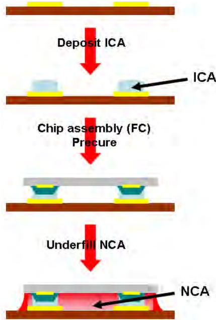
Figure 2.38: The principle of conventional adhesive assembly with isotropic conductive adhesives
