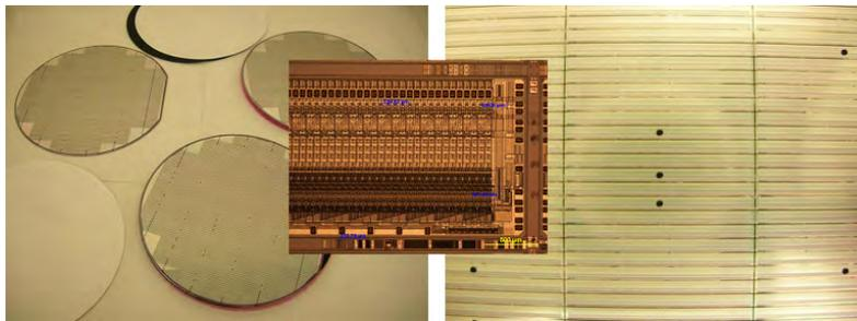
Figure 6.34: Wafers of the eDrive021 as supplied by ST: two were tested, one wasn't (the dots mark the faulty dies)
