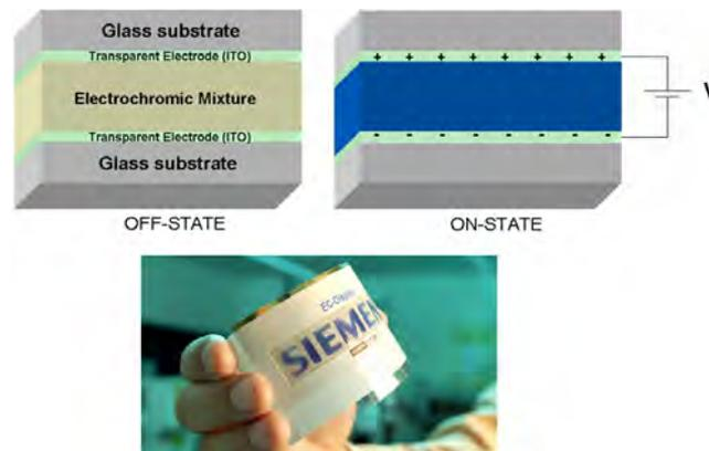
Figure 1.12: The electrochromic principle and an example of a display based on this principle (Siemens)
