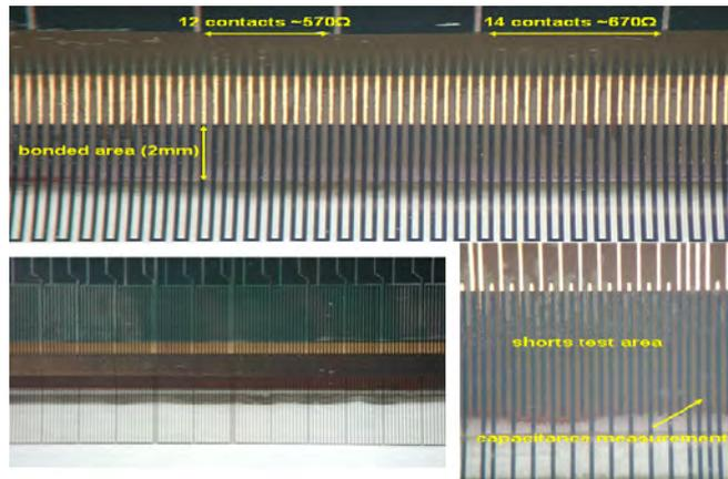
Figure 4.20: Assembled test TCPs (not on scale, widened): daisy chain (top) and shorts and capacitance (bottom) designs
