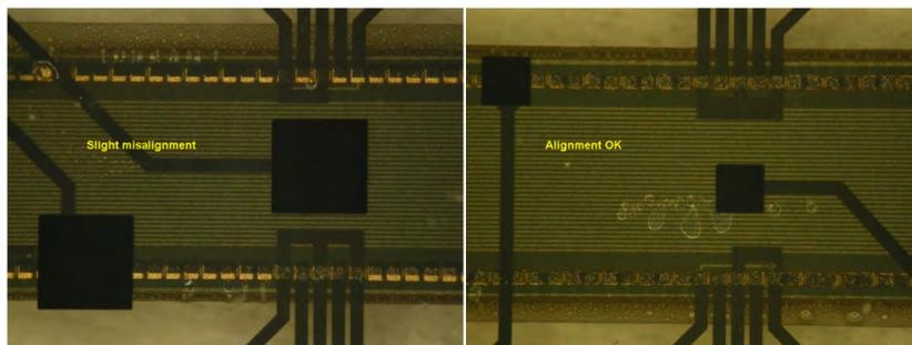
Figure 3.26: Some close-up results of the bonding trials: note the slight misalignment on the left, and the indentations on the contact pads (these are marks caused by the ACF's metal particles being pressed into the thin contact pads on the substrate during thermo-compression)
