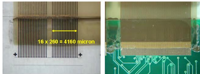
Figure 3.41: Flex foils bonded: column flex to glass (left) and row flex to PCB (right)
