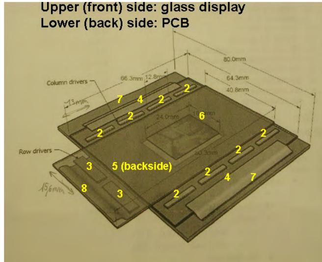
Figure 3.37: The assembly sequence for the HeMind module, illustrated on the design
