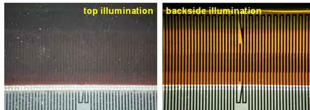
Figure 4.17: Aligning is much easier with backside illumination, mainly due to the thick PI
