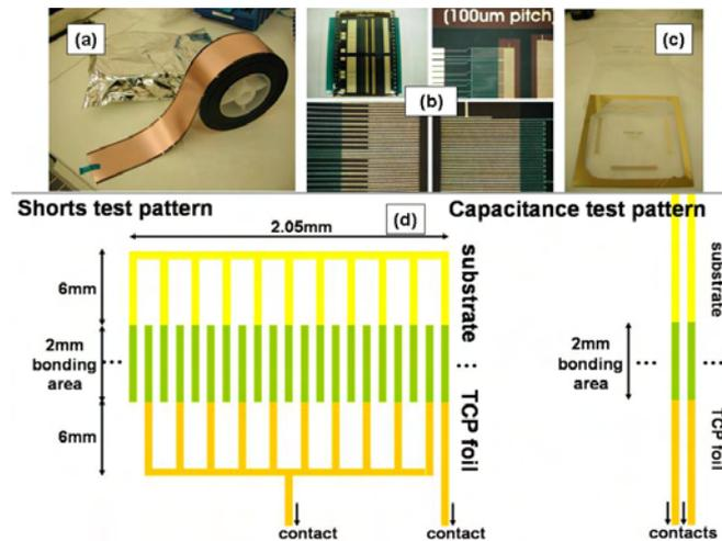
Figure 4.16: Tape material as delivered (a), after processing (b), patterned PET substrate (c) and design setup for shorts and capacitance testing (d)
