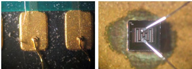
Figure 2.35: examples of wirebonding: gold wire ball-bonded to a gold contact pad (left) and aluminum wires wedge-bonded to a naked die (right)
