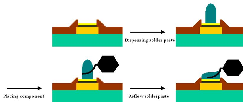
Figure 2.32: Bonding by Soldering
