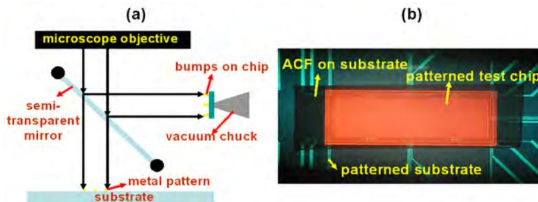
Figure 2.42: Aligning a chip to the substrate: (a) side view of principle, and (b) top view through microscope
