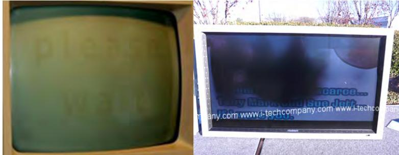
Figure 1.21: Illustrations of lifetime-limiting phenomena: phosphor burn-in, where an image is retained even when the display is off (left), and the isotropic stage, damaging liquid crystal so that the display effect is lost (right)
