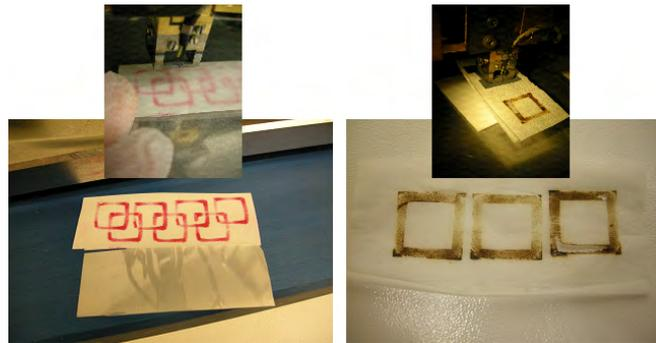
Figure 2.46: Two methods for calibrating the bonding thermode: using pressure-sensitive tape (left), and with filter paper (right)
