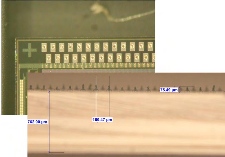
Figure 3.22: The input pads of the ISC9717 after bumping: the Au studbumps have a height of approximately  $75\ \mu\text{m}$
