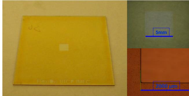
Figure 6.7: A cavity created in the photodefinable PI layer: two close-up top views of the cavity are shown on the right
