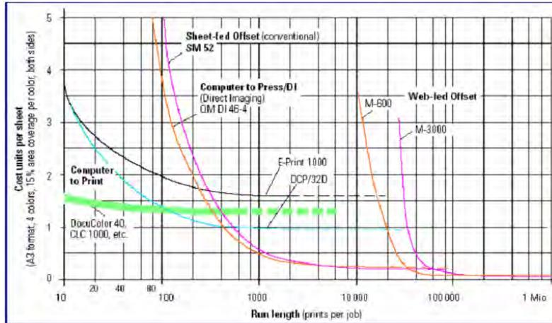
Figure 2.29: Examples of how to compare printing technologies: cost units per sheet in function of the run length
