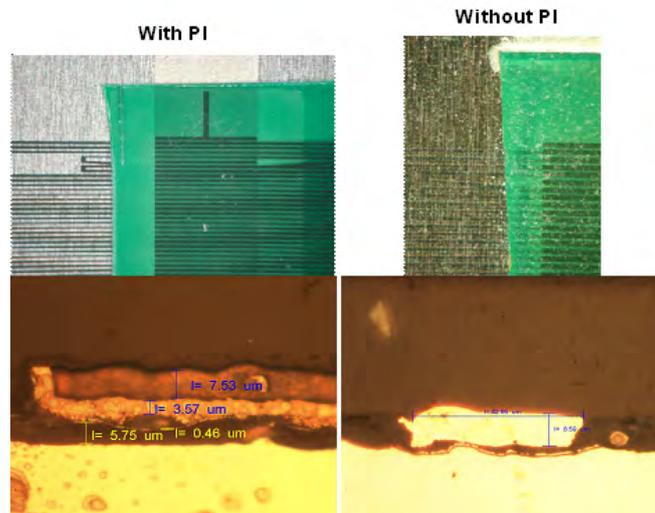
Figure 4.27: A PI insulating layer vs an  $\text{SiO}_2$  insulating layer for steel substrates
