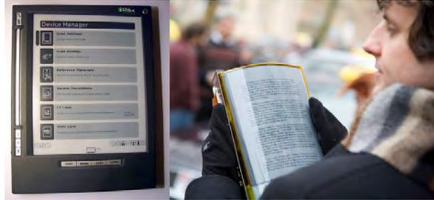
Figure 1.10: Electrophoretic displays: a rigid eReader, already commercially available (left, IREX Technologies), and a flexible variant under development (right, Plastic Logic)
