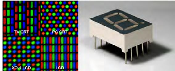
Figure 1.2: Pixel geometry of various CRT and LCD displays (left), and a typical 7-segment LED display component, with decimal point (right)
