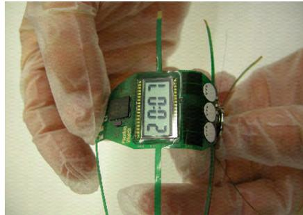
*Figure 3.8: An assembled flex watch*
