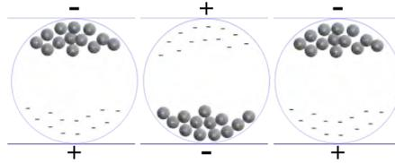
Figure 1.8: Principle of an electrophoretic display
