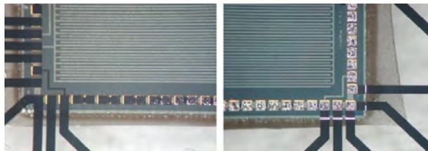
Figure 4.12: Pictures (left and right extremes) of an unevenly bonded test chip, 2.5 mm by 15 mm, 200  $\mu\text{m}$  pitch
