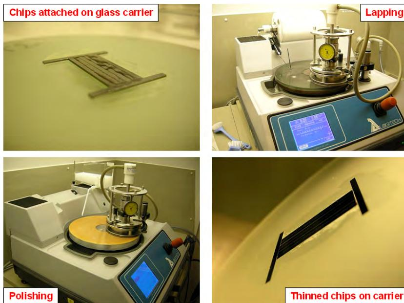
Figure 6.38: Illustration of the process of thinning the dies: here 8 dies are thinned at the same time (of which the outer 4 are dummies)
