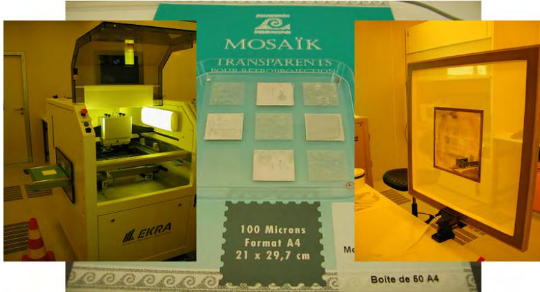
Figure 2.13: Stencilprinting setup: from left to right the screenprinter, one of the test prints, and the used stencil
