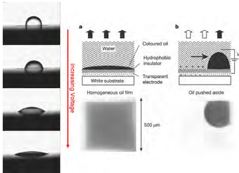
Figure 1.13: The principle of electrowetting illustrated (Liquavista): no voltage applied, therefore a coloured homogeneous oil film is present (a), DC voltage applied, causing the oil film to contract (b)
