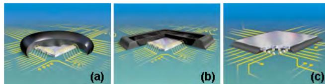
Figure 5.8: Reinforcement through encapsulation without (a) or with the aid of a damming material (b), or through underfilling (c)
