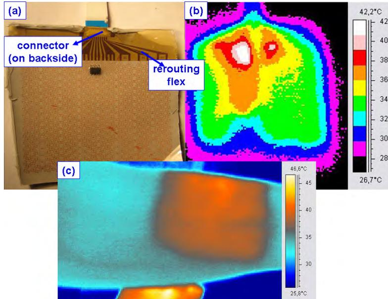
Figure 2.2: The upgraded version of the heating element: a picture of the fabricated result (a), as well as infrared images when operational, freestanding (b) and when placed on a volunteer's forearm (c)
