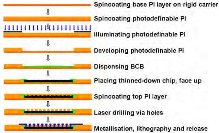
Figure 6.1: Process flow design for the flat UTCP technology
