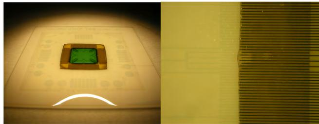
Figure 6.23: A UTCP assembled onto a patterned PES substrate
