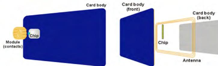
Figure 5.12: The principle of a smart card: with physical contact (left) and contactless (right)
