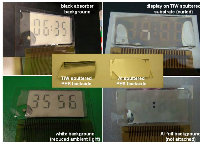
Figure 4.45: Illustrating the influence of the background on display performance: Al is a better mirror than TiW, but sputtering results in curling of the substrates
