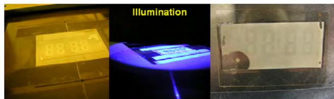
Figure 4.38: Once settled, the assembly is illuminated: after 5-10 seconds, polymerisation is visible as the PDLC turns opaque
