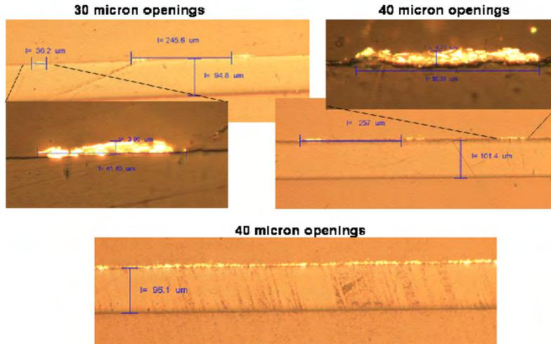
Figure 2.17: Stencilprinting results: cross-sections of the tracks corresponding with the 30 and 40  $\mu\text{m}$  openings
