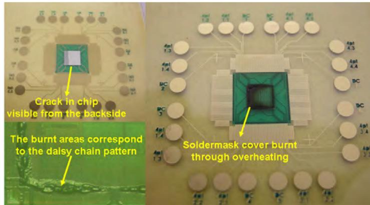
Figure 6.14: Burning the soldermask by electrically overheating through the daisy chain did not affect the electrical performance
