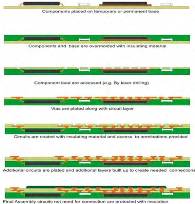
Figure 5.15: The Occam process (Verdant Electronics) proposes another route towards embedding
