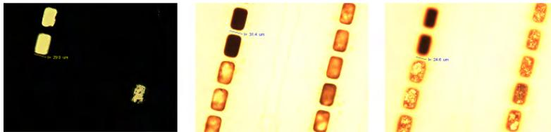
Figure 2.19: Stencilprinting results: clogged 30  $\mu\text{m}$  openings, lighted from the backside (left), focused on the stencil surface (middle) and focused on the clogged silver (right)
