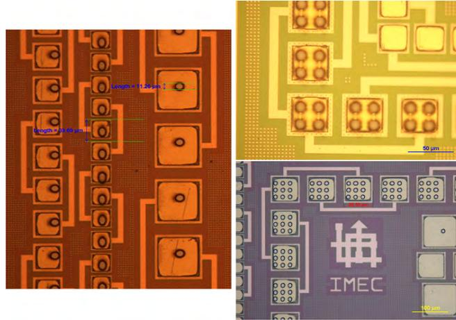
Figure 6.33: Laser drilled via holes in the top PI layer: from a single via for each contact (left), to a number of parallel vias, 2 by 2 and 3 by 3, to reduce contact resistance (right)
