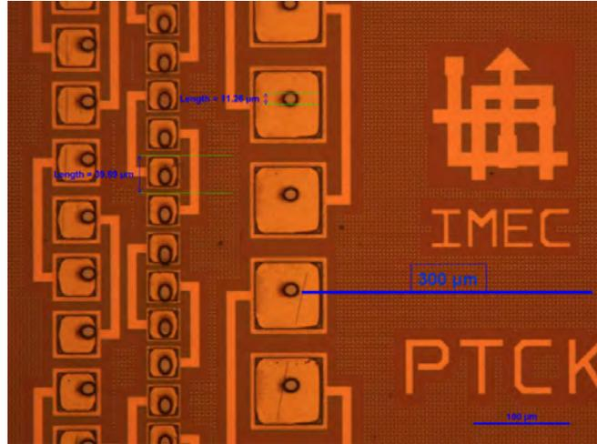
Figure 6.10: Laser drilled vias in the top PI layer to contact the bumped contact pads of the chip underneath, for all three types of bond pads
