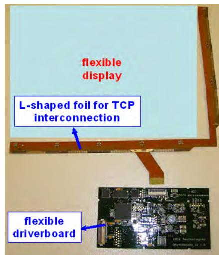
*Figure 5.4: The flexible driving electronics module for driving a flexible display demonstrator, developed within FlexiDis*
