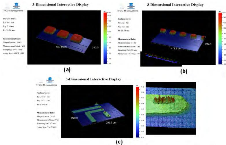
Figure 4.8: Optical inspection of the wafer surface, 2<sup>nd</sup> batch, shows the results of the test chip bumping process: pitches (a) 200  $\mu\text{m}$ , (b) 100  $\mu\text{m}$  and (c) 50  $\mu\text{m}$  (underplated)
