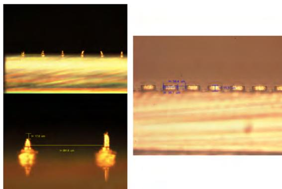
Figure 3.47: The highly irregular studbumps of the row driver (left), as compared to the flat, plated bumps of the column driver (right)
