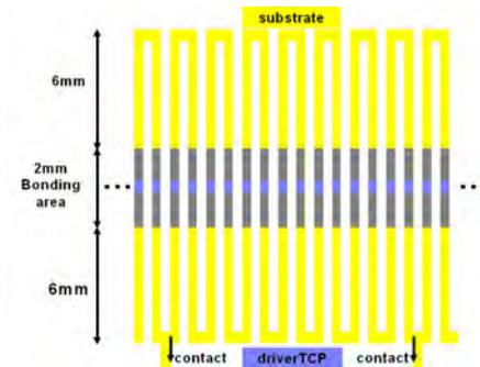
Figure 4.26: Setup for electrical interconnection testing of bonds with existing TCPs
