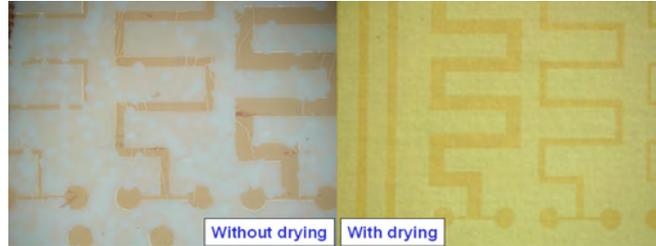
Figure 4.34: The influence of drying out the PES substrates before processing: without (left), bubbles are observed after illuminating the photoresist, resulting in bite-like marks and cracks after developing
