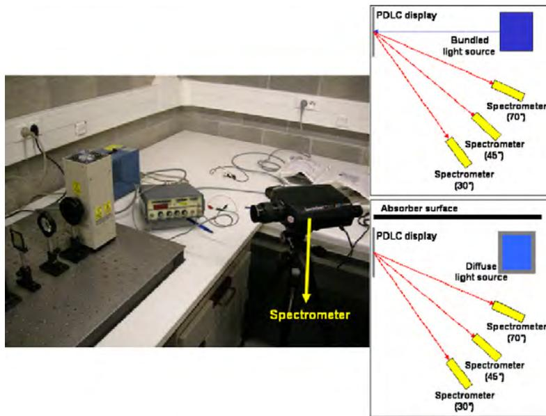
Figure 4.41: The setup for measurements in reflection, which better reflects the actual viewing experience for a user (considering the wristwatch-application in mind)
