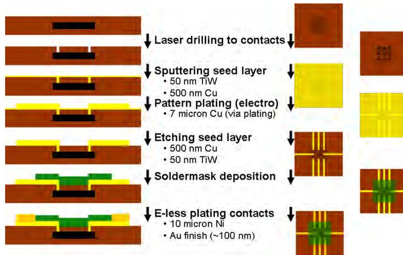
Figure 6.12: Schematic representation of the metallization process
