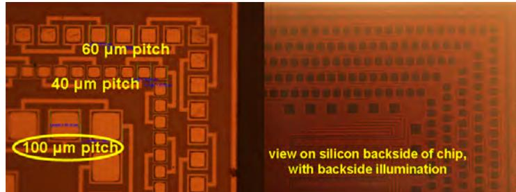
Figure 6.5: A thinned-down test chip: zoom on the different peripheral bond pads to be used (left) and a view of a backlit test chip illustrating the thinness (right)
