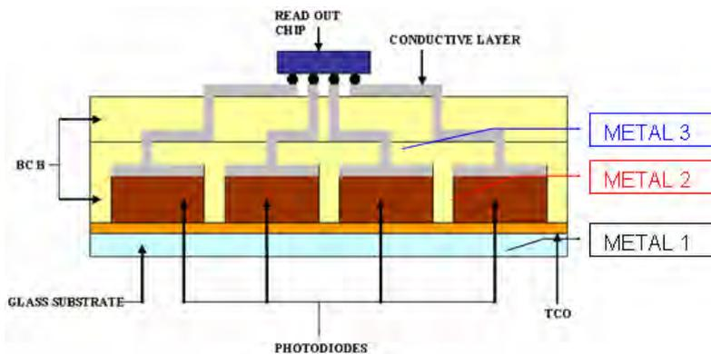
Figure 3.20: A schematic crosssection view of the detector structure (Patent application: A. Nascetti, M. Overdick, WO2003019659, "Sensor arrangement consisting of light-sensitive and/or x-ray sensitive sensors", Koninklijke Philips Electronics N.V.)
