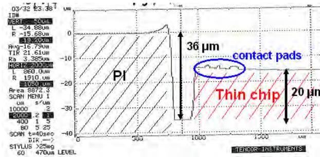
Figure 6.9: An AFM (Atomic Force Microscopy) measurement shows that the PI layer is thicker than the thin chip, and even the bumped contact pads can be spotted
