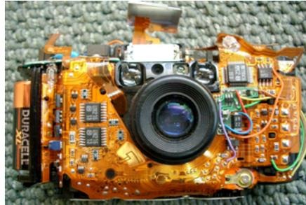
*Figure 2.5: A camera without the case, revealing the flex circuit assembly (Olympus)*
