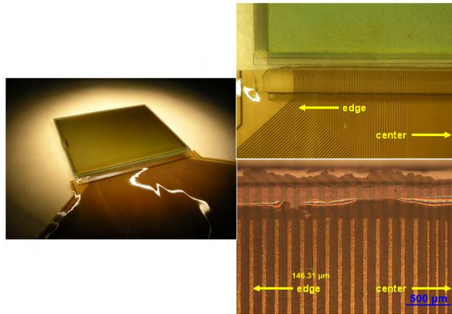
Figure 3.2: A display contacted by an interposer tape: the contacts are significantly denser towards the middle of the bond area (right)
