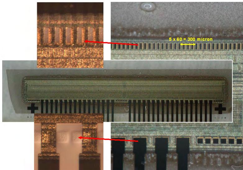
Figure 3.39: Column driver chips bonded to the display
