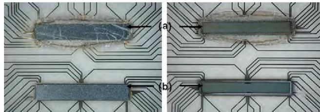
Figure 4.10: Comparison between bonding on glass and on PET, top and bottom view: (a) bonding carried out under “glass conditions”, 30s @ 300°C, no interposer; (b) bonding with modified conditions, 30s @ 170°C, 0.2mm silicone interposer
