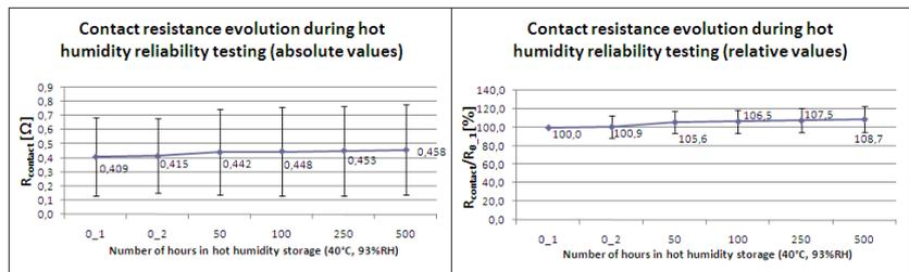
Figure 6.48: Hot humidity storage reliability in absolute and relative values
