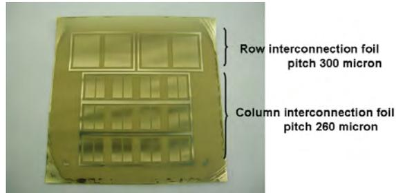
Figure 3.34: Patterned flex foils for interconnecting driver inputs (row and column) to the underlying PCB
