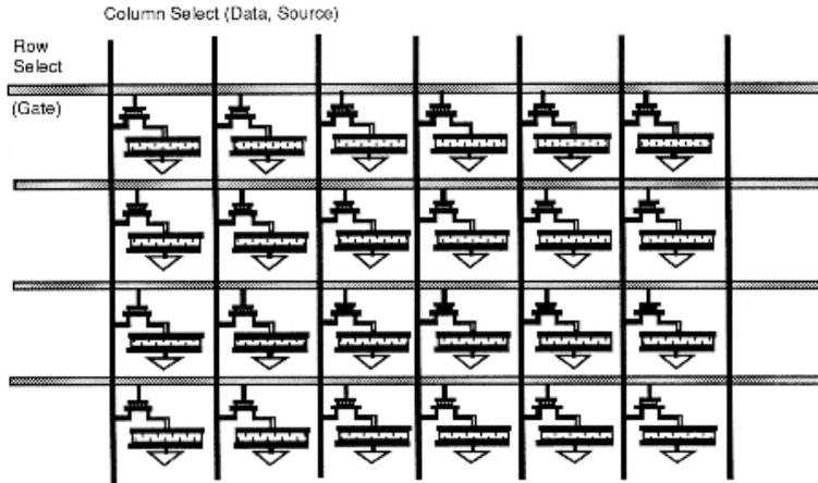
Figure 1.25: Schematic of an active-matrix driven display
