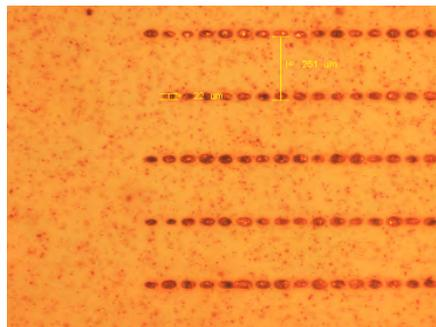
Figure 2.18: Stencilprinting results: drops at the extremities of the smaller printed lines
