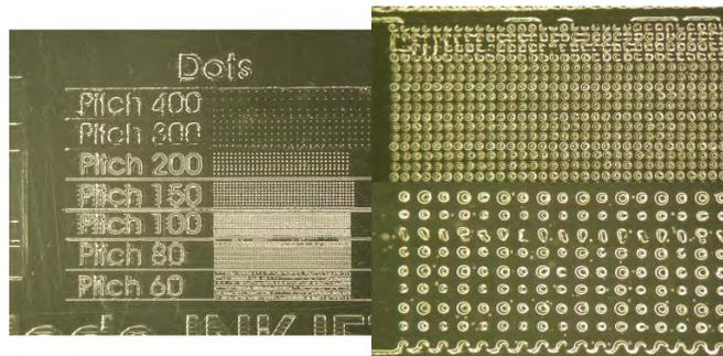
Figure 2.31: Inkjetprinting an etch mask: first trials on glass
