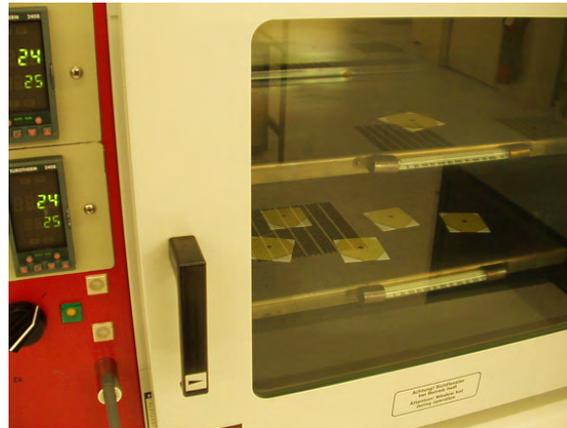
Figure 6.8: After aligning and placing the chip, the BCB is cured in an oven
