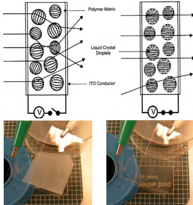
Figure 4.31: Working principle of PDLC displays: the liquid crystal is dispersed under the form of spheres in a polymer matrix, and is driven similarly as in a standard liquid crystal display
