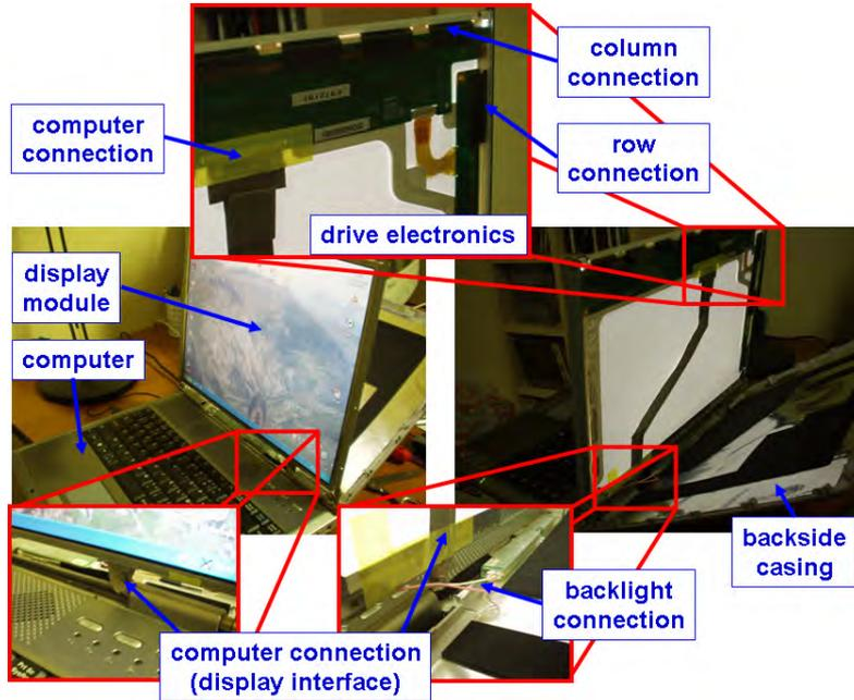
Figure 1.1: A disassembly of a laptop reveals the display module and its interconnection mechanism: the driving electronics are integrated at the back of the display (on top of the backlight), the display interface is connected to the computer by a single wiring foil
