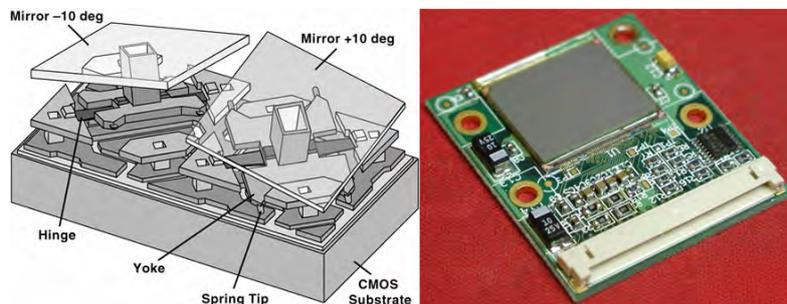
Figure 1.15: A schematic of a Digital Micromirror Device (left, Texas Instruments), and a microdisplay built with LCoS technology (right, TFCG Microsystems)
