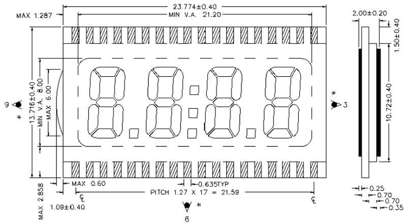
Figure 3.13: Layout schematics of the VI-451(R0) Varitronix LCD display (dimensions in mm)
