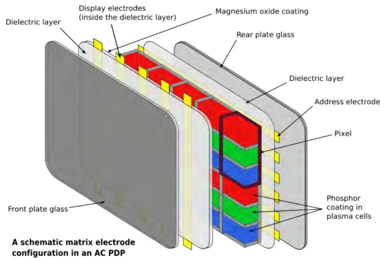
Figure 1.11: Composition of plasma display panel (PDP)
