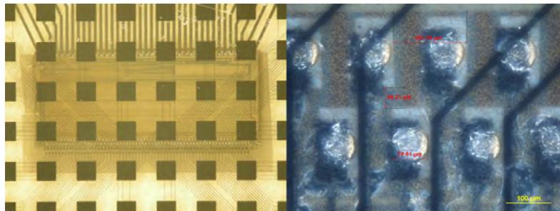
Figure 3.30: Results of the assembled demonstrators: an ACF bonded chip (left) and a close-up of the input area of the read-out chip (right, the studbumps are aligned to the contact pads on the substrate)
