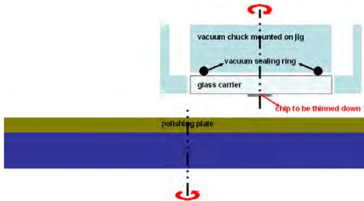
Figure 6.37: A cross-section view of the chip thinning process, based on lapping and polishing
