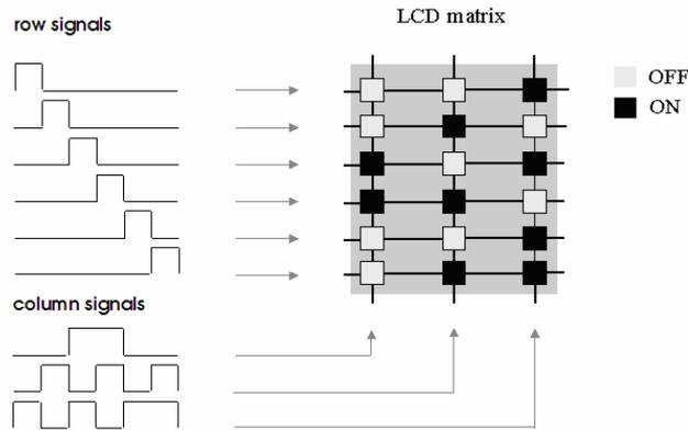
Figure 1.24: Principle of a passive-matrix driven display
