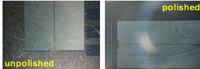
Figure 4.25: Comparison of polished and unpolished steel substrates
