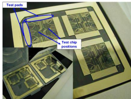
Figure 4.6: Pictures of Au-patterned PET substrates for flip chip tests
