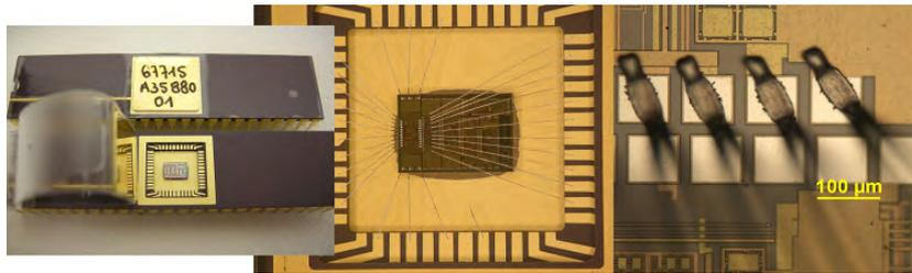
*Figure 2.36: Illustration of wirebonding as a standard technique for assembling chips in semiconductor packages*
