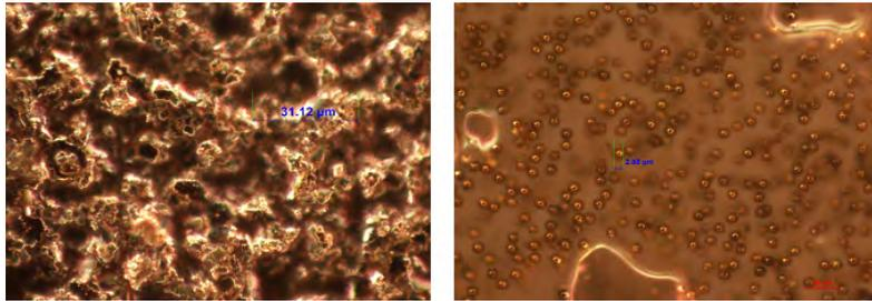
Figure 2.37: Isotropic and anisotropic conductive adhesive as seen through a microscope
