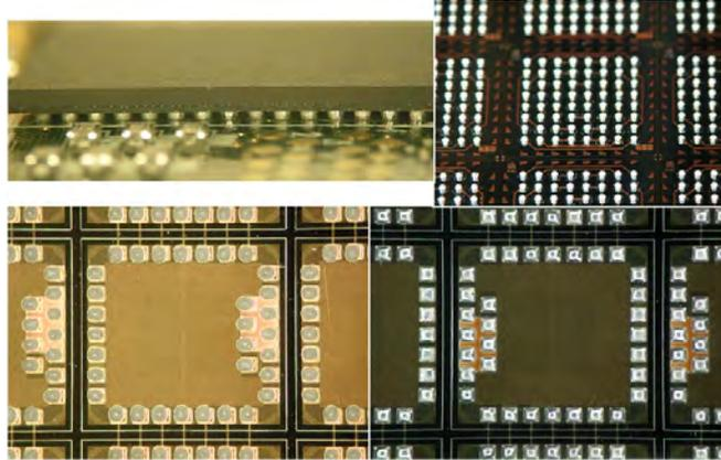
Figure 2.34: Illustrating the use of solder bumps: an assembled BGA package (top left), solder balls applied as bumps on naked dies (top right, 450  $\mu\text{m}$  pitch), and the deposition of solder paste for wafer-level bumping before and after curing (bottom left and right, 300  $\mu\text{m}$  pitch)
