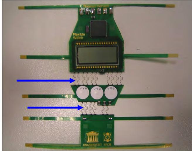
*Figure 3.9: The stretchable adaptation of the flex version: note the meander shaped interconnections*
