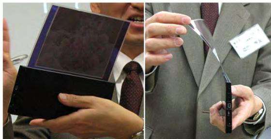
*Figure 5.7: Bridgestone's flexible QR-LPD (Quick Response - Liquid Powder Display), as shown at the FPD International 2007 exhibition in Yokohama*
