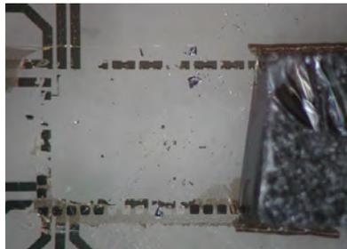
Figure 4.15: Chip broken off the substrate
