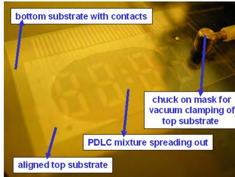
Figure 4.37: The top substrate is aligned and brought into soft contact with the bottom substrate; the drop of PDLC spreads out across the cell gap defined by the spacers
