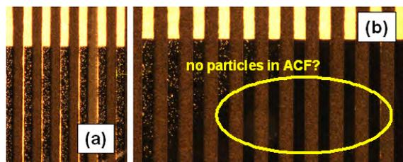
Figure 4.19: (a) ACF particles are pressed into the contacts, as seen through the substrate. (b) No electrical interconnection due to a lack of particles in the ACF (visible because no indentations are noticed)
