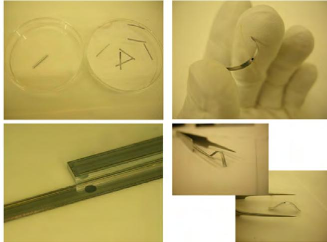
Figure 6.39: Results of the thinning process: note the flexibility of the thin dies
