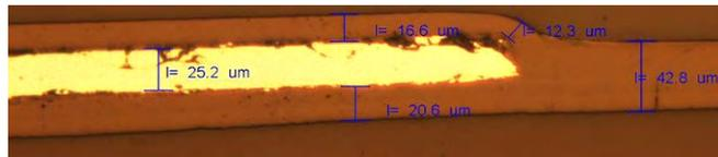
Figure 5.18: A cross-section of the fabricated UTCP illustrates the thicknesses of the different layers
