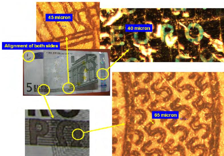
*Figure 2.24: Banknotes are good examples of the possibilities of high speed printing technologies: high volume, small features and aligning both sides*
