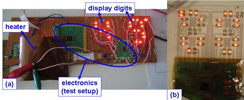
Figure 2.3: The complete setup: (a) the setup to test driving and reading out the heating element, and (b) the upgraded version of the setup, with stretchable display and flexible electronics
