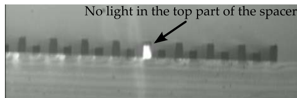
Figure 4.10 – Light stays confined and is not escaping into the top part of the spacer owing to its lower refractive index.
