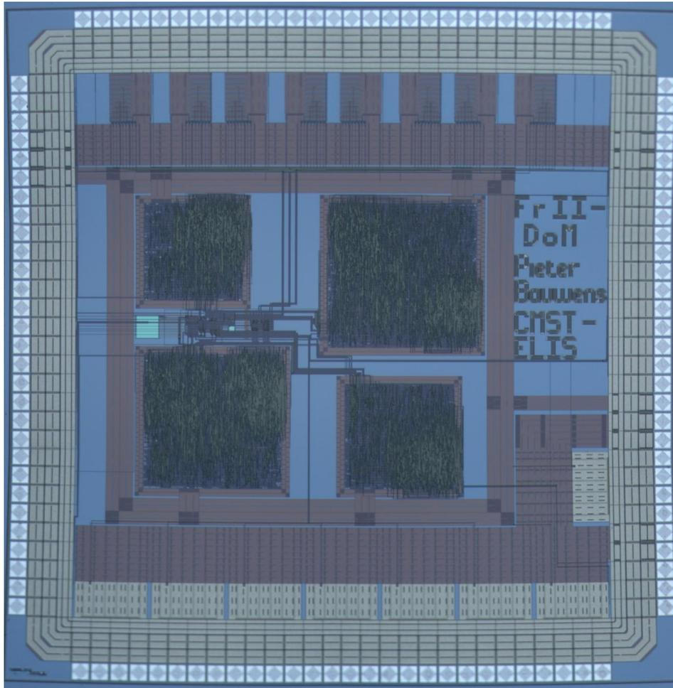
**Figure 9.2** – The layout of the FrIIDoM driver. The four distinct blocks are the four drivers (left to right, top to bottom: driver 0, driver 3, driver 2, driver 1). On top and at the bottom you can see the 8 current sources and 8 switches respectively.
